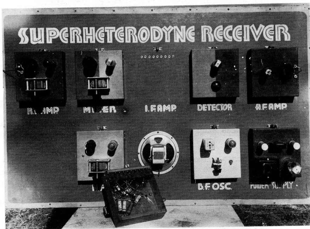
HERE THE I.F. BLOCK IS REMOVED TO SHOW PLUG-IN CONNECTIONS.
