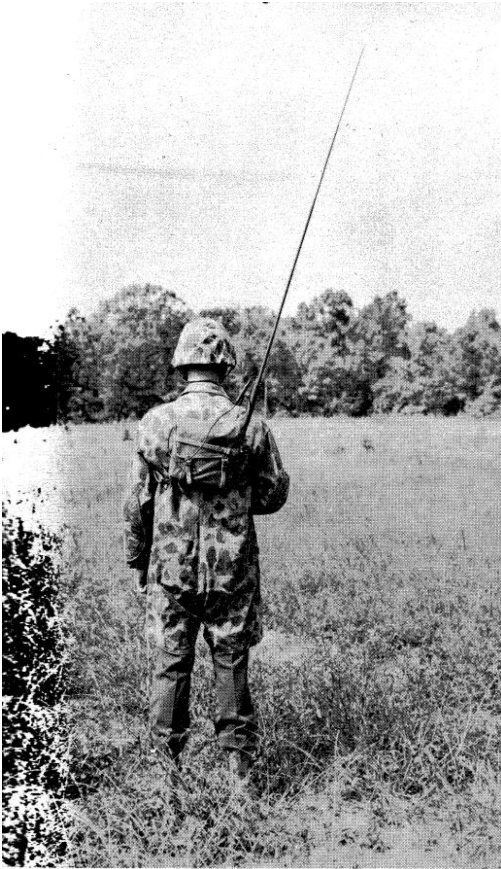
Position of MAB Equipment Ready for Operation After Jumping.
