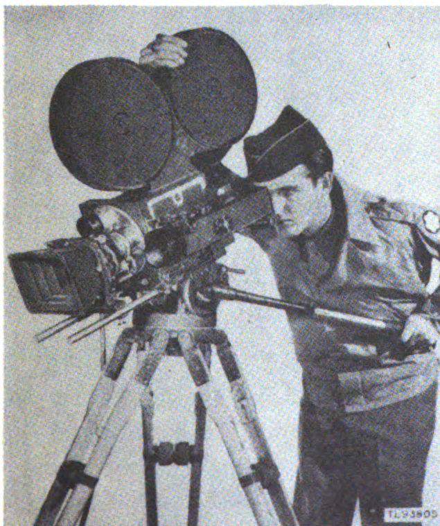
Figure 98. Operating camera: downward tilt movement.
