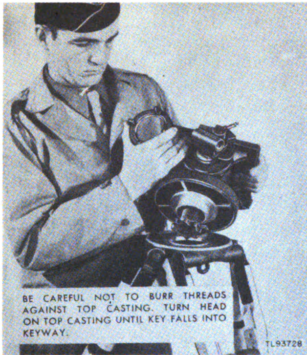
Figure 21. Mounting tripod head on tripod.
