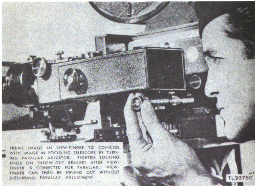
Figure 83. Adjusting view-finder for parallax.
