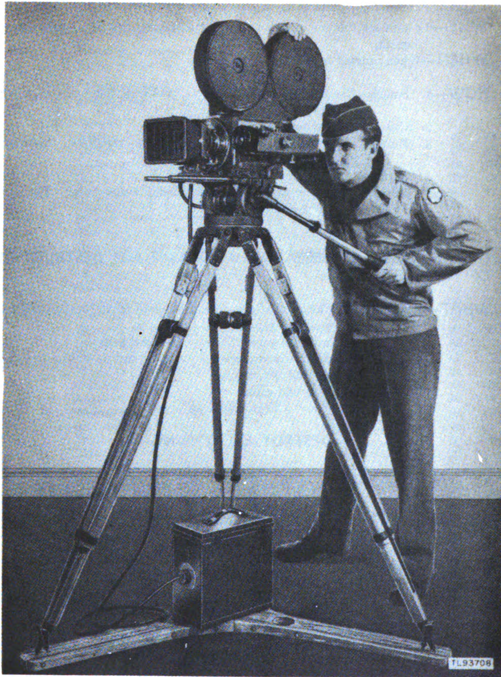
Figure 1. Camera set up for normal operation.
