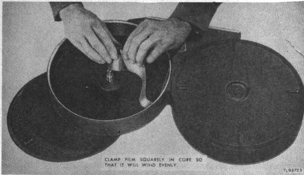
Figure 16. Loading magazine: attaching film to take-up core.
