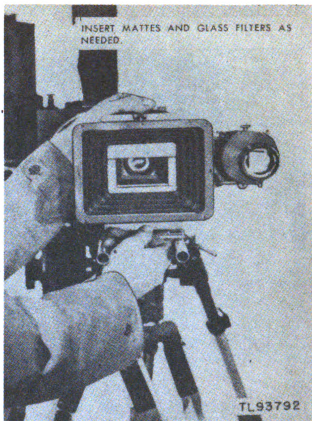
Figure 85. Inserting mattes in sunshade and matte box.
