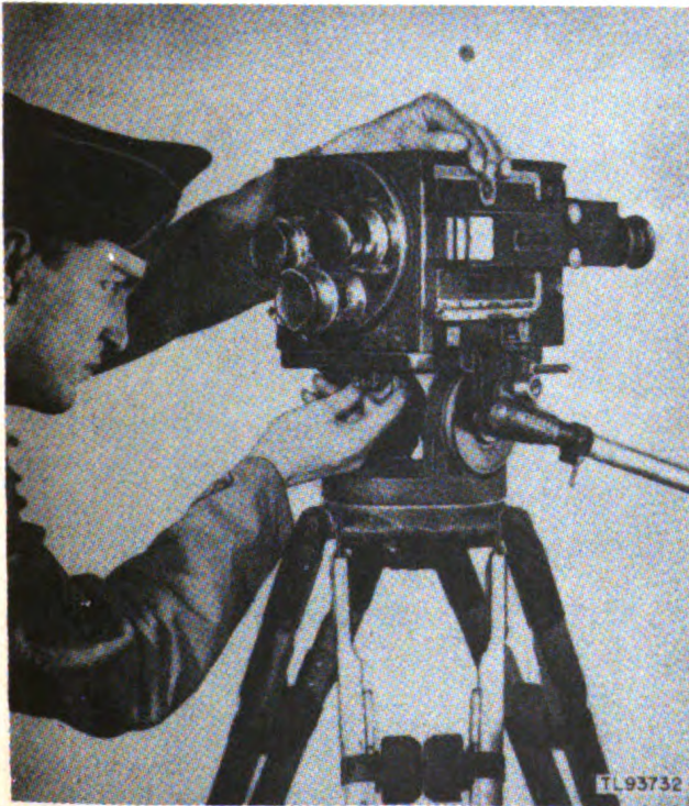
Figure 25. Hand-tightening camera on tripod head.
