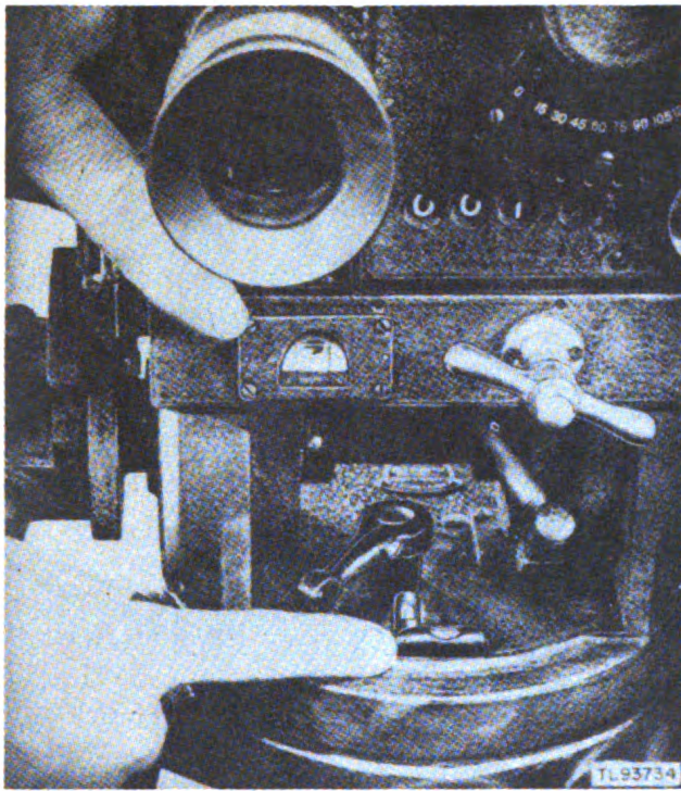
Figure 27. Camera and tripod levels.
