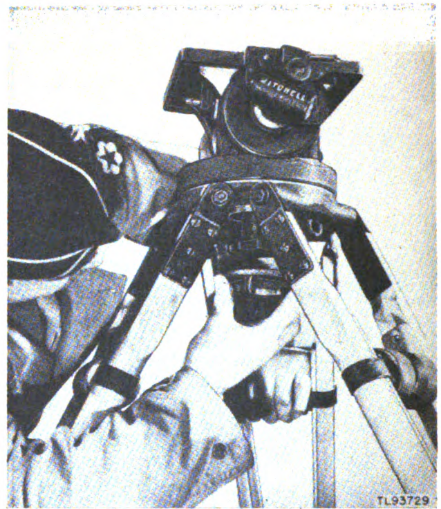
Figure 22. Securing tripod head to tripod with locking nut.
