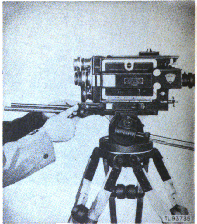
Figure 28. Attaching sunshade and matte box bracket.
