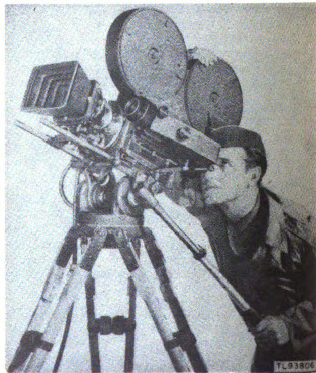
Figure 99. Operating camera: upward tilt movement.
