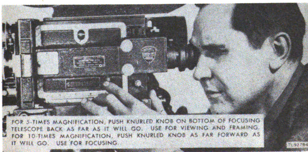
Figure 77. Adjusting image magnifier of focusing telescope.
