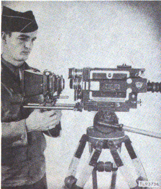
Figure 29. Attaching sunshade and matte box.
