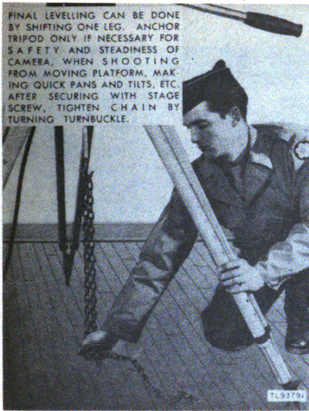
Figure 84. Anchoring tripod after final positioning of camera.
