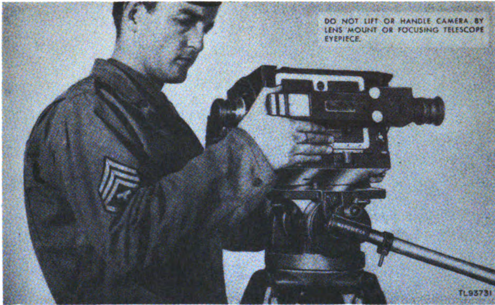
Figure 24. Mounting camera on tripod.
