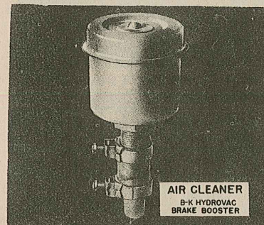
Fig. 3 - Look for an air cleaner on things that suck in air and have delicate parts.
