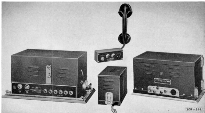
Figure 90. Radio Set SCR-298, components.
