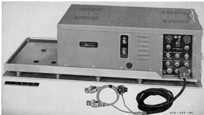
Figure 89. Radio Receiver and Transmitter BC-500-B in Mounting FT-239, part of Radio Set SCR-293-B.
