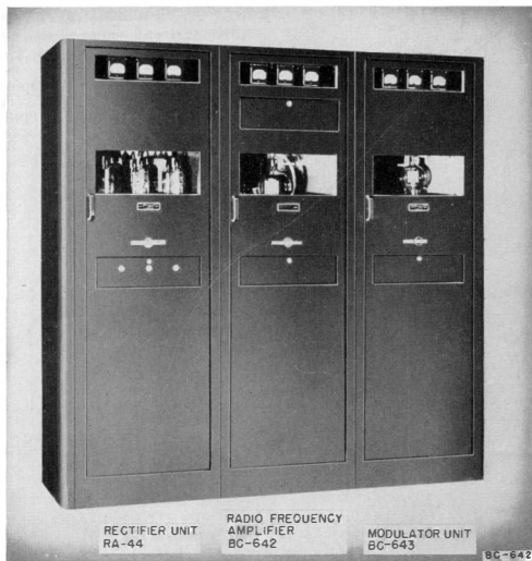
Figure 45. Radio Frequency Amplifier BC-642 in operating position with Rectifier Unit RA-44 and Radio Modulator Unit BC-643.
