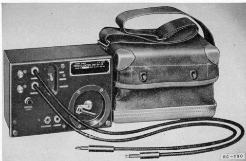
Figure 81. Remote Control Unit RM-29 and Case CS-76 components of Remote Control Equipment RC-290.
