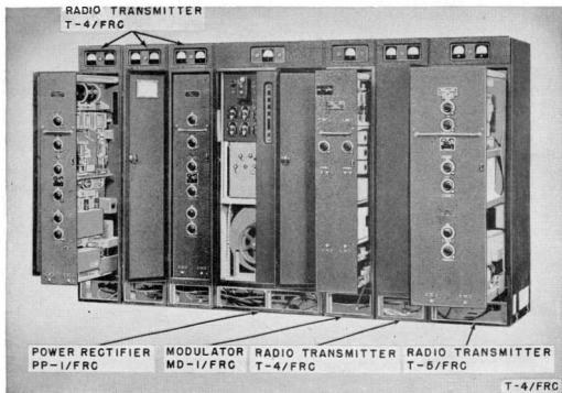
Figure 115. Radio Transmitter T-4/FRC and associated equipment, front view, units pulled out from rack.
