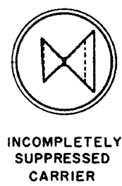
Figure 105. Double-trapezoid patterns observed on phase-shift ssb transmitter.
