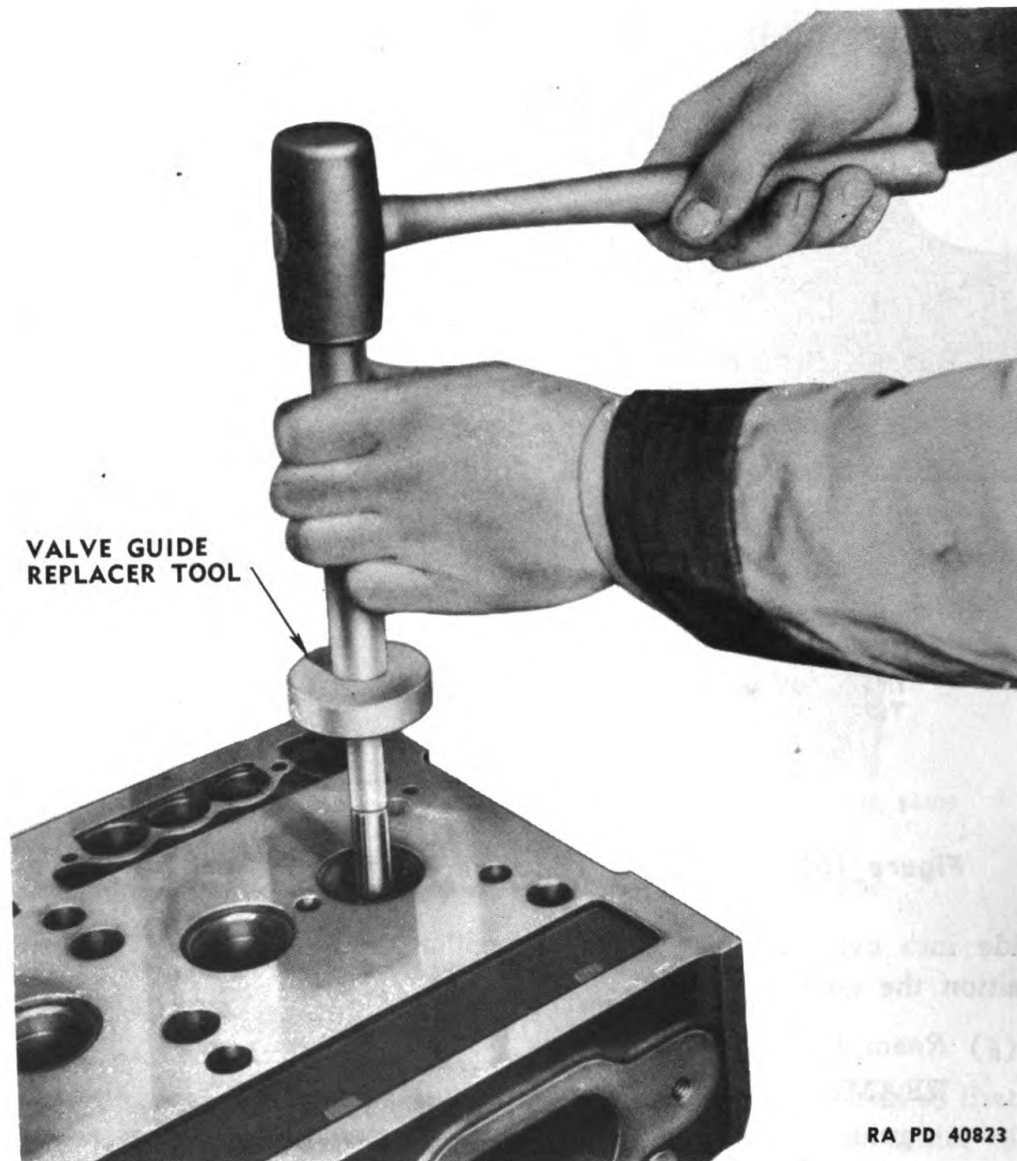
Figure 104 — Installing Valve Guides
