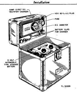
Figure 7. Power Supply PE-150.
