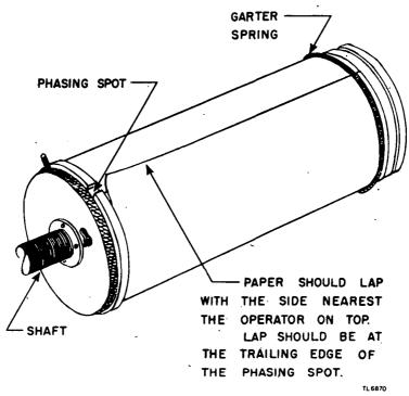
Figure 11. Correct way to mount direct recording paper on drum.
