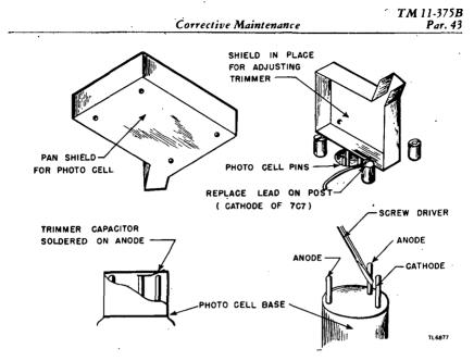
Figure 26. Balancing photocell of Facsimile Transceiver FX-1.
