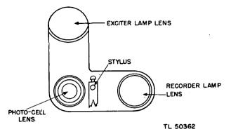
Figure 13. Exterior lenses to be cleaned.
