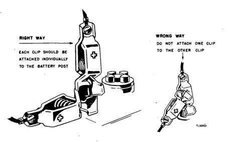
Figure 8. Battery terminal connections.
