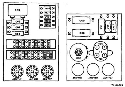
Figure 18.2. Parts lay-out, Facsimile Transceiver TT-1/TXC-1 (serial Nos. 91 through 190)
