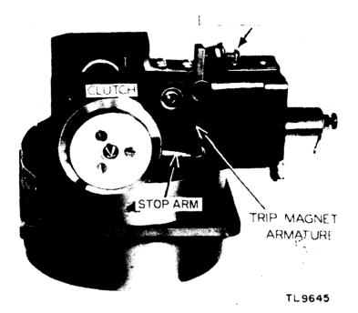
Figure 30. Motor and trip magnet of Facsimile Transceiver FX-1-B.
