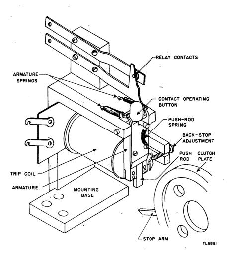
Figure 31. Trip magnet of Facsimile Transceiver FX-1.
