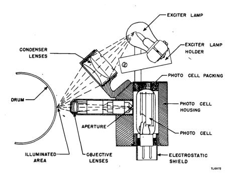
Figure 21. Transmitting optical system.
