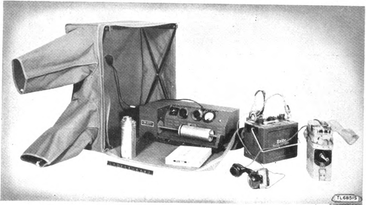
Figure 69. Set-up for photographic reception, battery operation, using portable dark tent.
