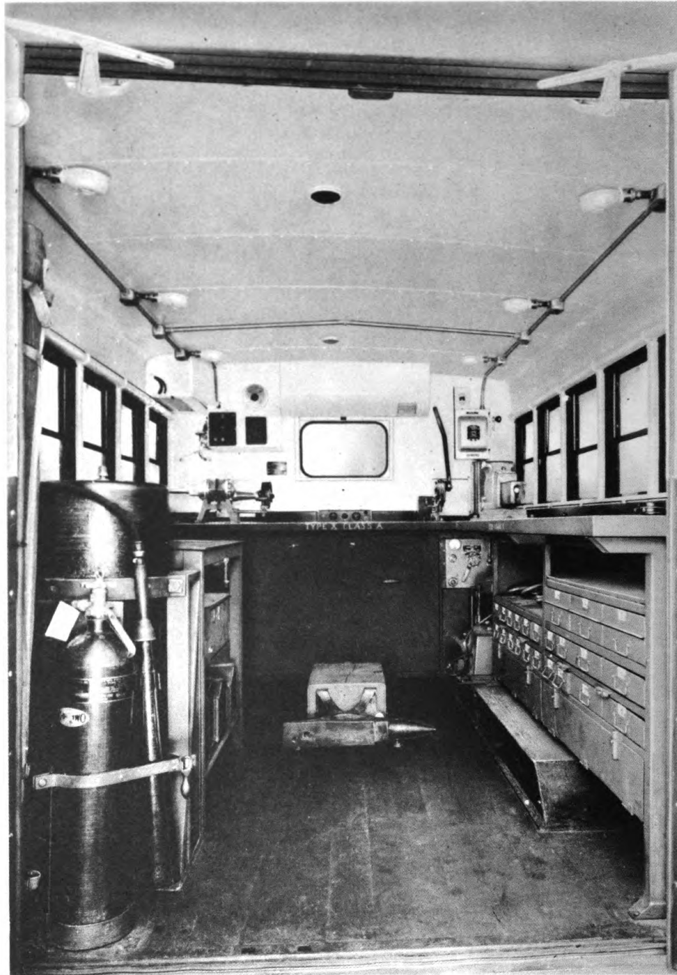
Figure 156a – Interior of Welding Truck M12 Showing Anvil and Block in Traveling Position
