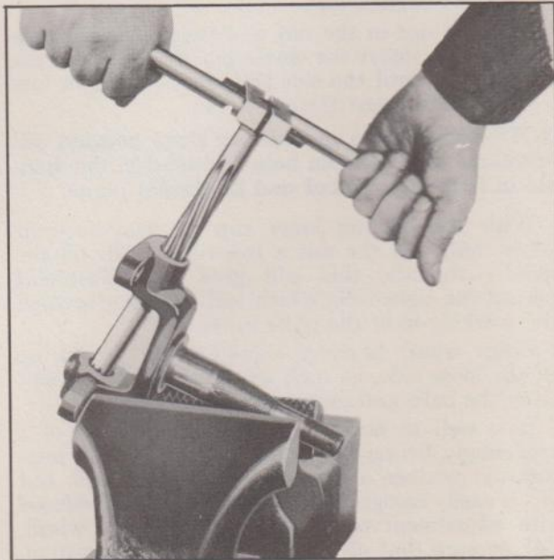
Fig. 11—Reaming Steering Knuckle Bushings
