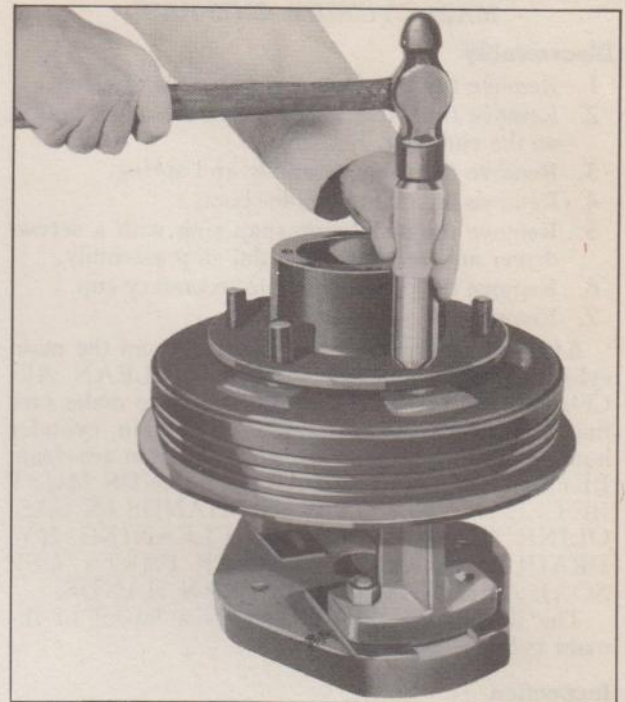
Fig. 22—Peening Hub and Drum Bolts
