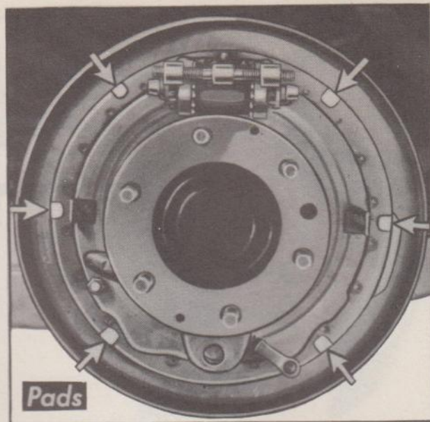
Fig. 20—Checking Alignment of Brake Shoes with Flange Plate
