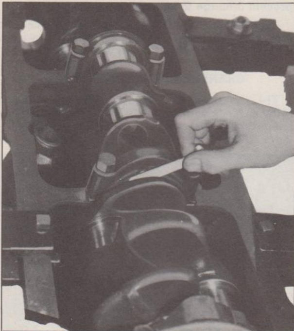
Fig. 13—Checking Crankshaft End Play
