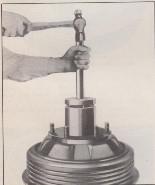
Fig. 18—Driving Outer Race into Contact with Snap Ring
