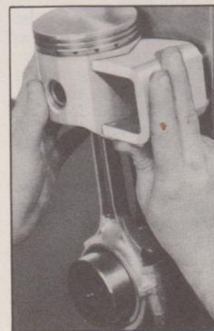
Fig. 31—Checking Piston and Connecting Rod Assembly
