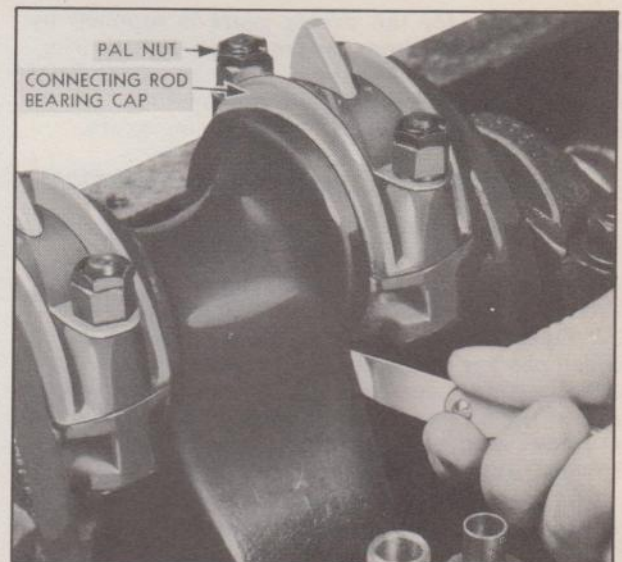
Fig. 34—Checking Connecting Rod Bearing Side Clearance
