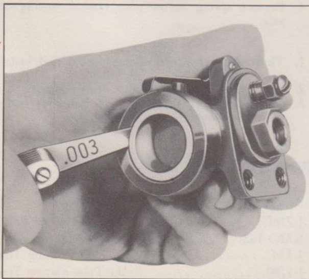
Fig. 27—Checking Wheel Cylinder Piston Fit
