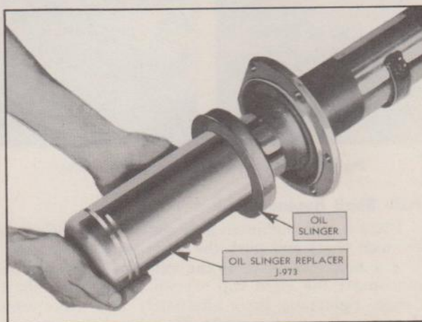
Fig. 20—Oil Slinger Replacer
