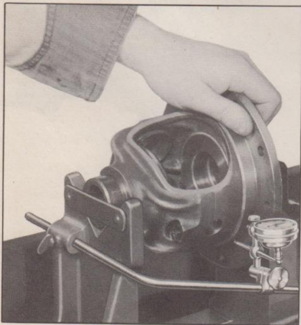
Fig. 9—Checking Run-Out of Differential Case
