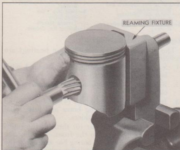
Fig. 4—Reaming Piston Pin Bushings
