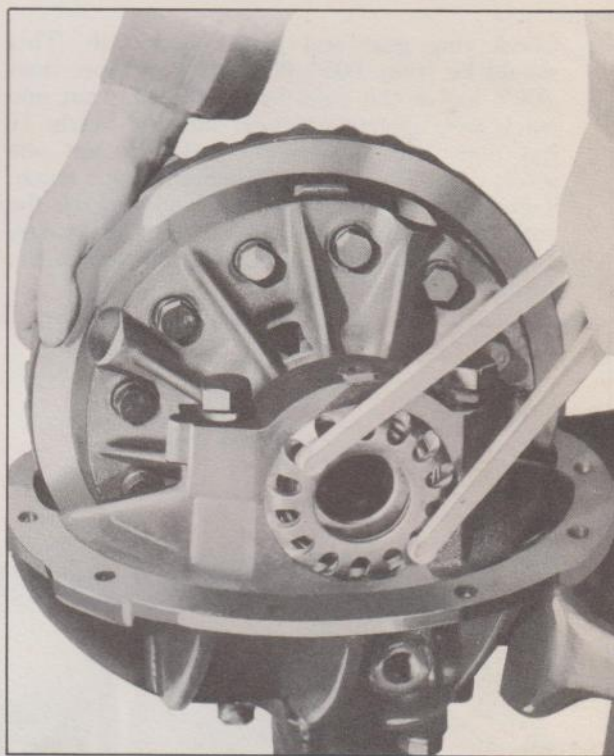
Fig. 28—Adjusting Ring Gear and Pinion Back Lash
