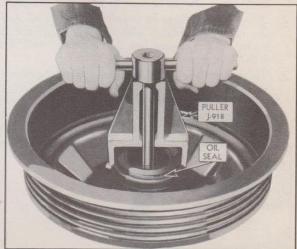
Fig. 16—Removing Inner Bearing and Oil Seal
