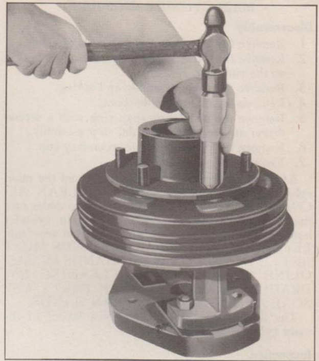
Fig. 22—Peening Hub and Drum Bolts
