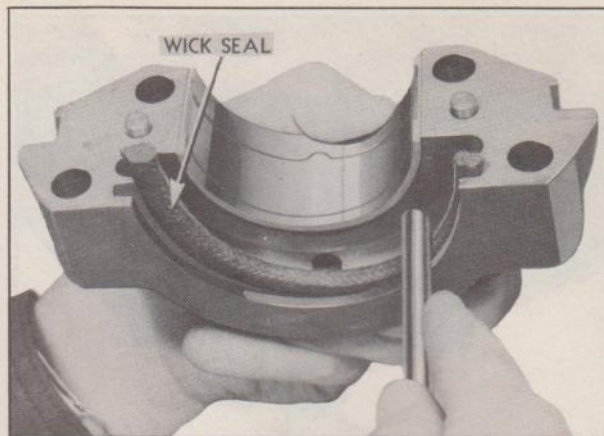
Fig. 12—Installing Rear Main Bearing Oil Seal
