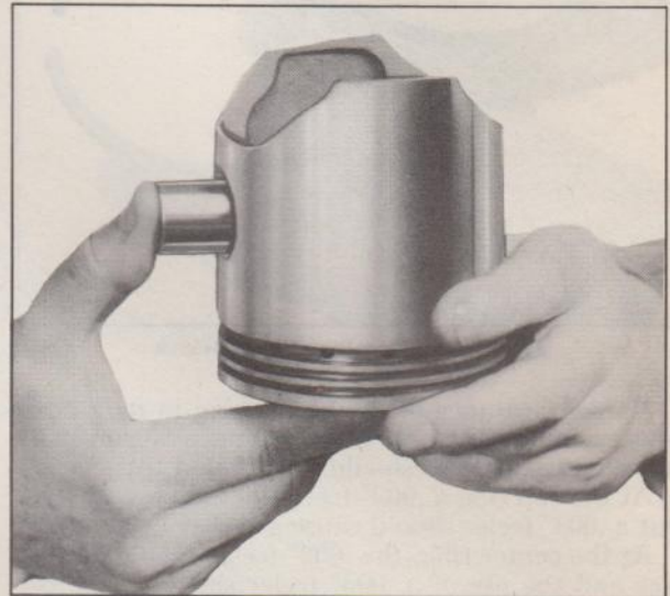
Fig. 5—Checking Piston Pin Fit
