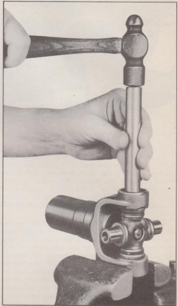
Fig. 42—Removing Trunnion Bearings from Joint Yoke
