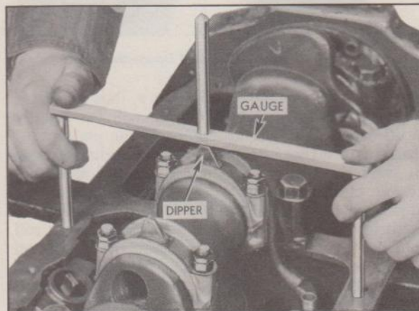
Fig. 36—Checking Connecting Rod Dipper Height
