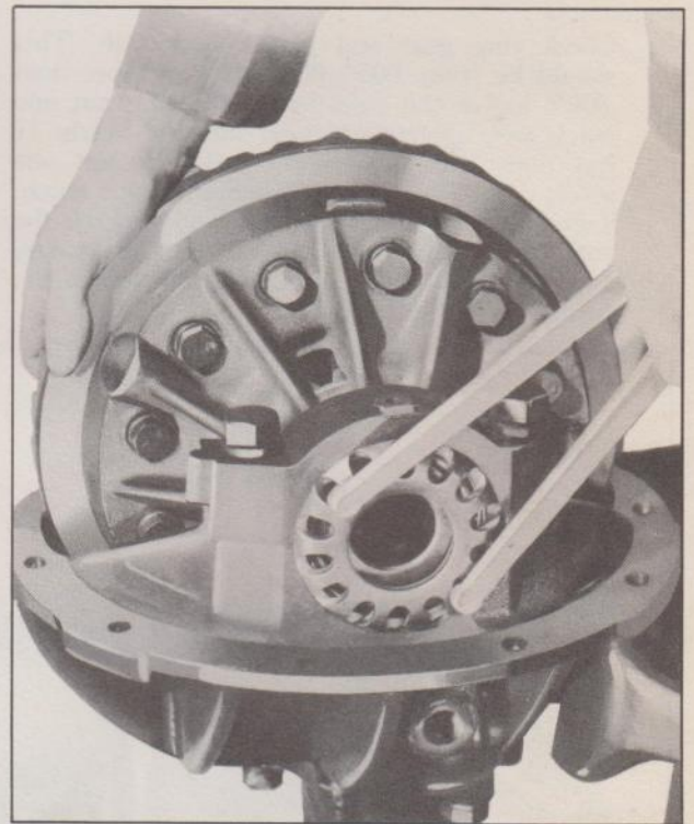
Fig. 28—Adjusting Ring Gear and Pinion Back Lash
