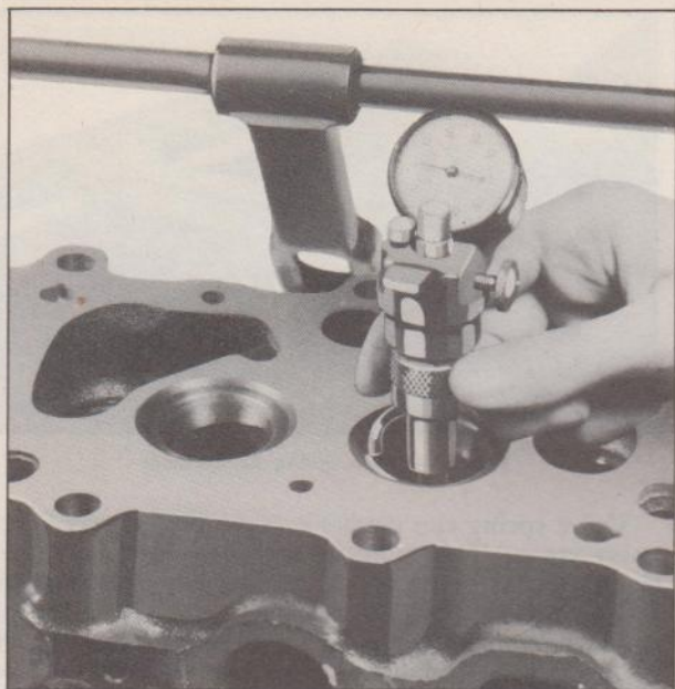
Fig. 49—Checking Valve Seat with Indicator Gauge
