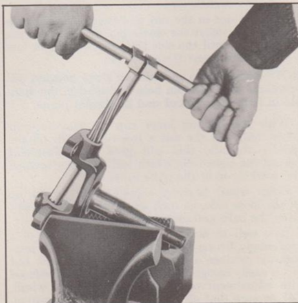
Fig. 11—Reaming Steering Knuckle Bushings
