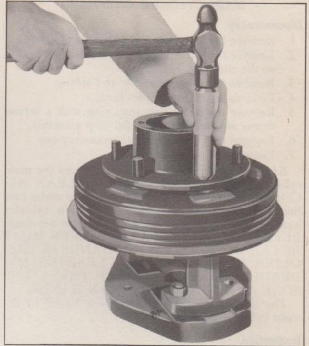
Fig. 22—Peening Hub and Drum Bolts
