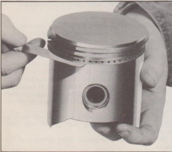
Fig. 7—Checking Piston Ring Clearance
