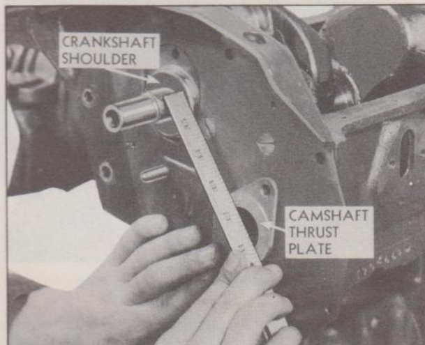
Fig. 16—Checking Alignment of Timing Gears
