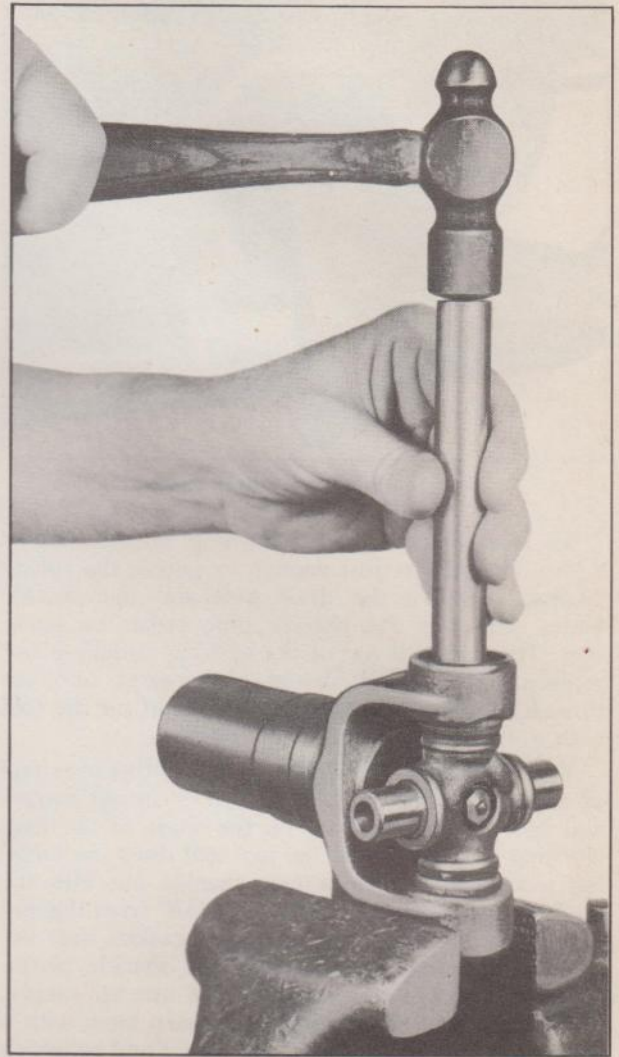
Fig. 42—Removing Trunnion Bearings from Joint Yoke
