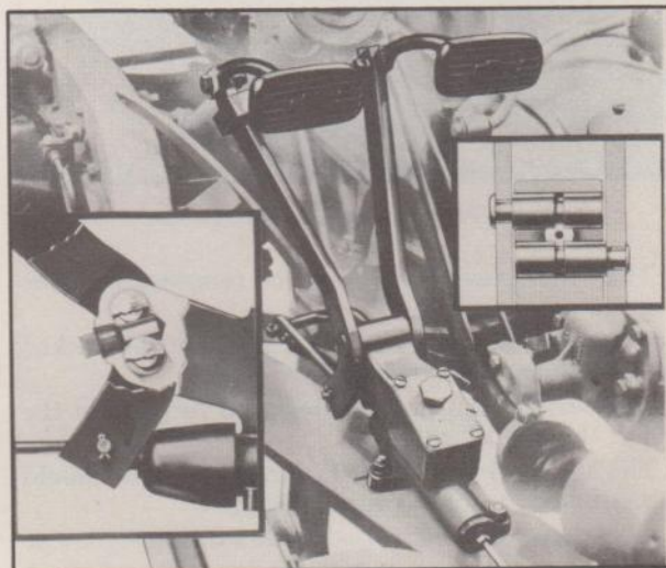
Fig. 14—Clutch and Brake Pedal Mounting—1/2-Ton Trucks
