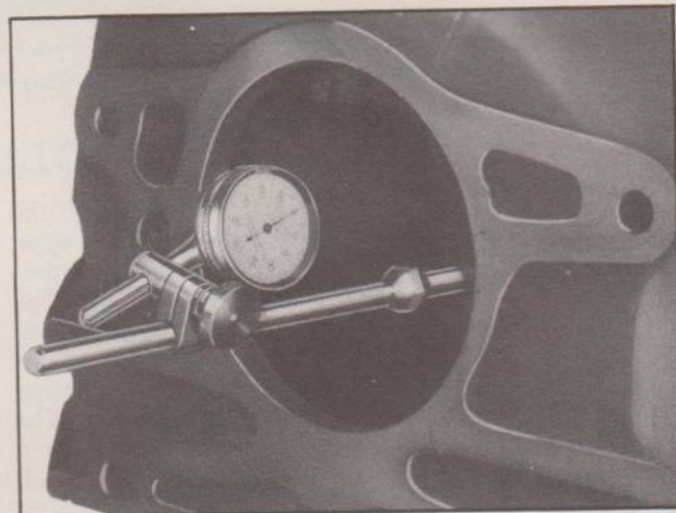
Fig. 6—Checking Transmission Pilot Hole Run-Out
