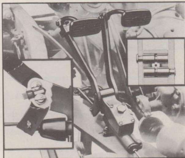
Fig. 14—Clutch and Brake Pedal Mounting— \frac{1}{2} -Ton Trucks
