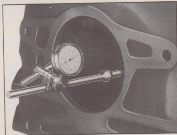
Fig. 6—Checking Transmission Pilot Hole Run-Out
