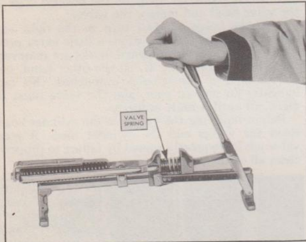
Fig. 52—Valve Spring Tension Gauge
