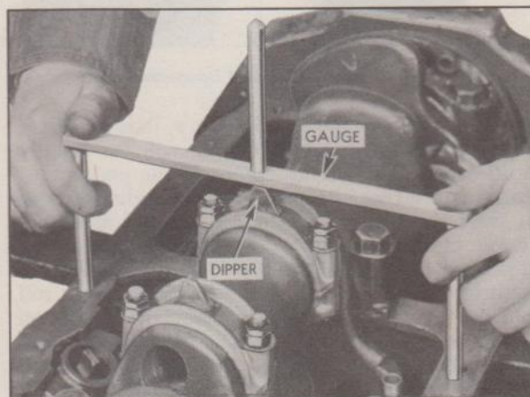
Fig. 36—Checking Connecting Rod Dipper Height
