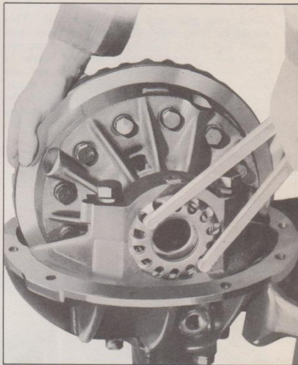
Fig. 28—Adjusting Ring Gear and Pinion Back Lash
