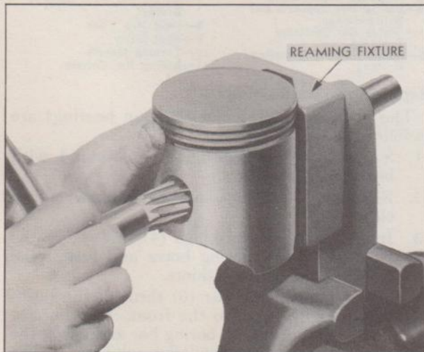
Fig. 4—Reaming Piston Pin Bushings
