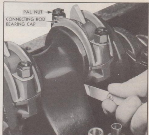
Fig. 34—Checking Connecting Rod Bearing Side Clearance
