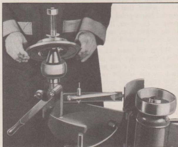
Fig. 9—Installing Leveling Plate
