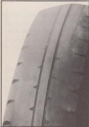
Fig. 3—Tire Wear Due to Under Inflation
