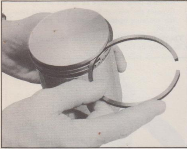
Fig. 6—Checking Ring Fit in Groove
