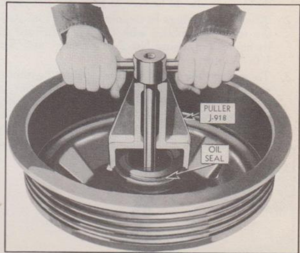
Fig. 16—Removing Inner Bearing and Oil Seal
