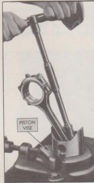
Fig. 30—Assembling Connecting Rod to Piston
