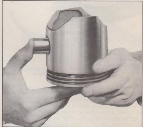
Fig. 5—Checking Piston Pin Fit
