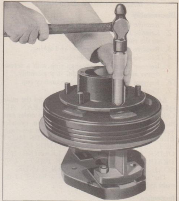
Fig. 22—Peening Hub and Drum Bolts
