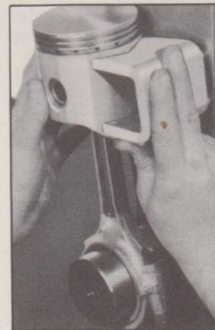
Fig. 31—Checking Piston and Connecting Rod Assembly
