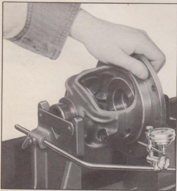
Fig. 9—Checking Run-Out of Differential Case
