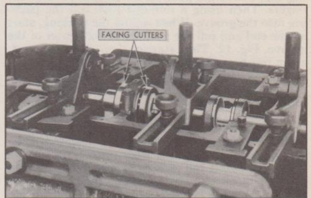
Fig. 10—Facing Rear Intermediate Bearing
