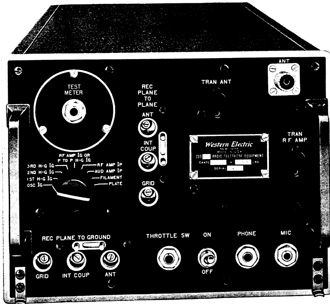
Figure 2—RT-19/ARC-4 Radio Transmitter-Receiver: External Front View
