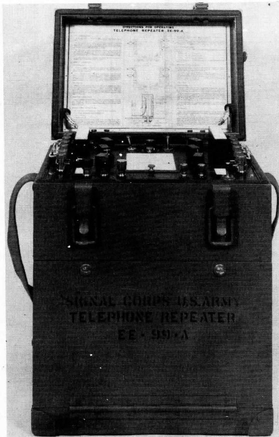
TELEPHONE REPEATER EE-99-A, PART OF REPEATER SET TC-29-( )
