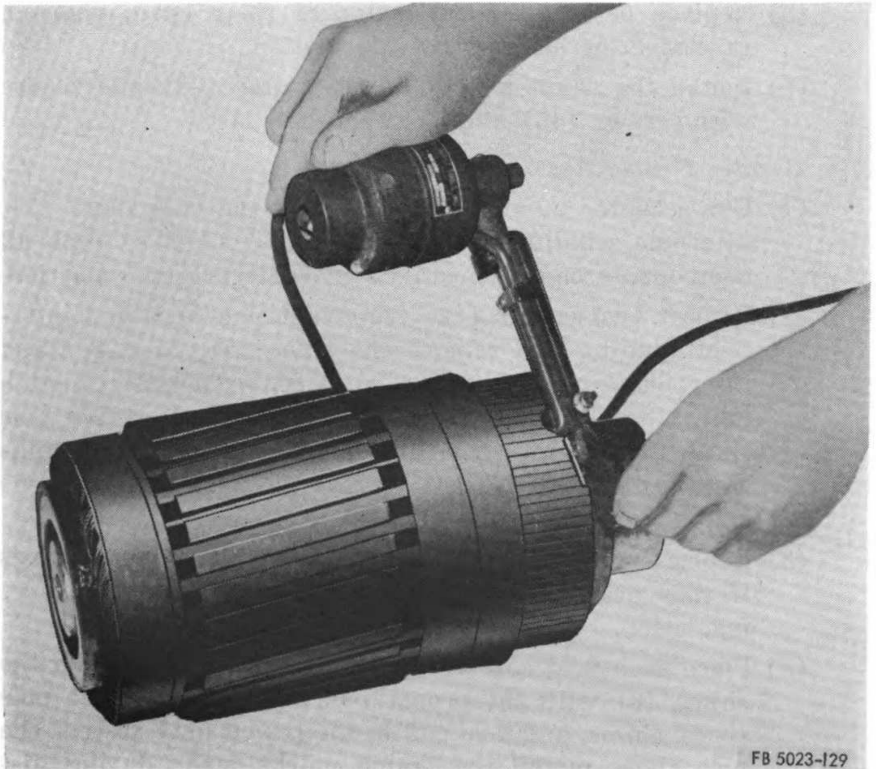
Figure 129. Undercutting commutator mica.
