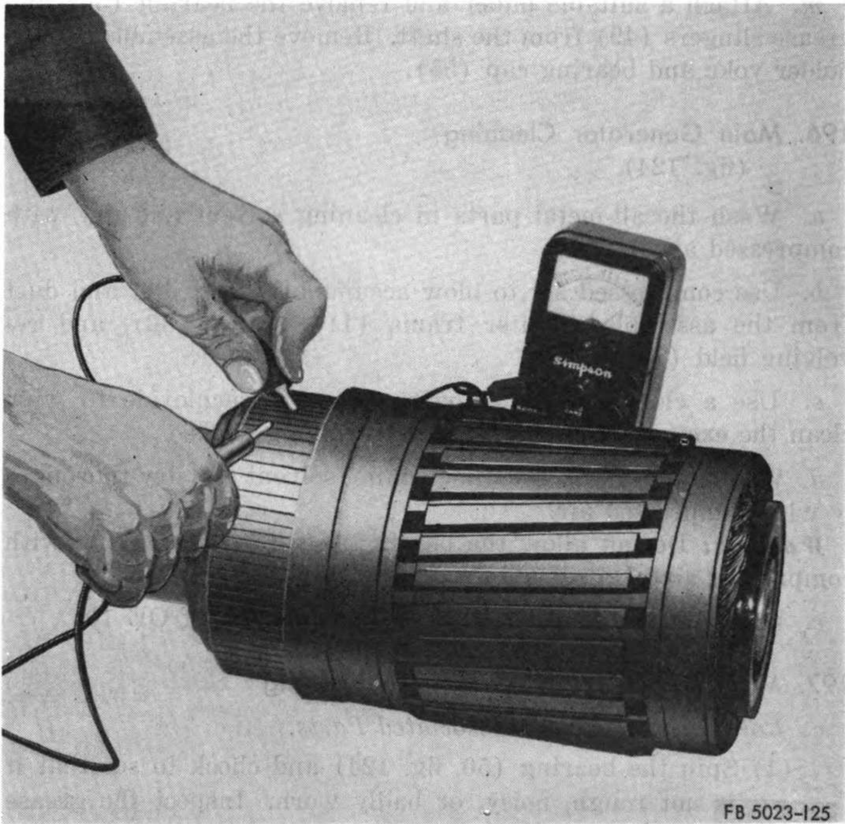
Figure 125. Testing exciter armature with ohmmeter.
