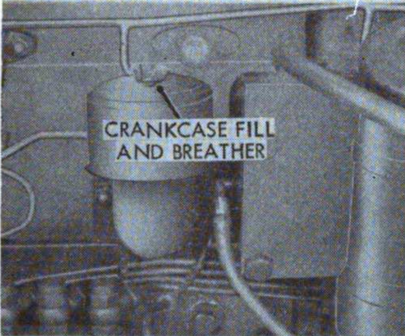
REFERENCE 3: Remove breather cap, clean and reoil.
