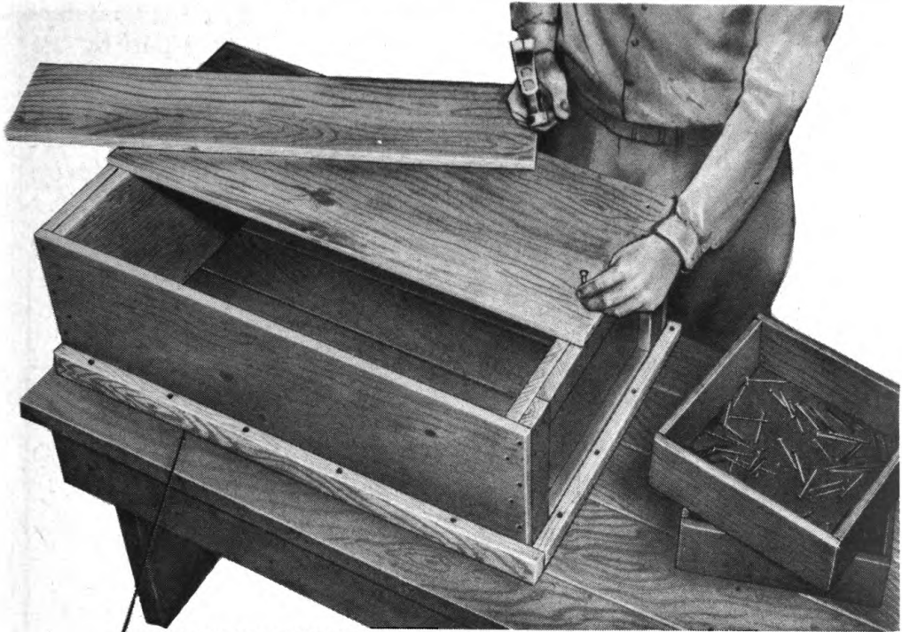
— TEMPLATE ON BENCH KEEPS BOX "SQUARED UP" DURING ASSEMBLY.
