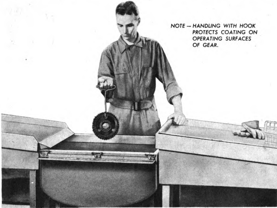
Figure 1 — Method of Dipping and Removing Gear From Bath of Heated Corrosion-preventive Compound
