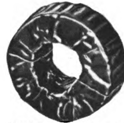
AFTER SECOND DIP OTHER HALF COATED WITH OVERLAP AT CENTER.
