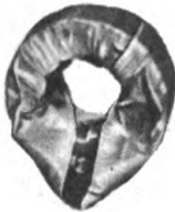
ONE END OF CYLINDER MOLDED TO INSIDE OF GEAR, THIS BEING REPEATED WITH OTHER END.
