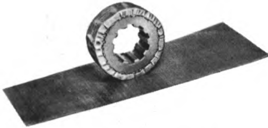
GEAR WITH EDGES CUSHIONED, PLACED ON SHEET OF GRADE C GREASEPROOF WRAPPING PAPER.
