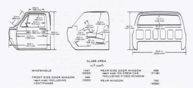
Note: Interior dimensions measured with front seat in rearmost position; seat travel is 5 inches.
