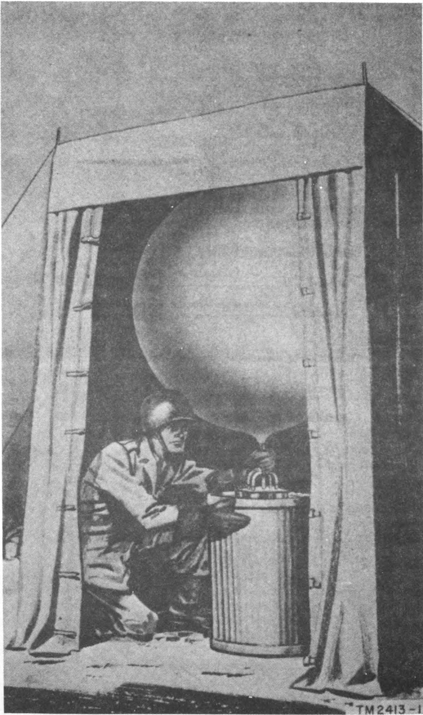
Figure 1. Hydrogen Generator Set AN/TMQ-3 in operation.
