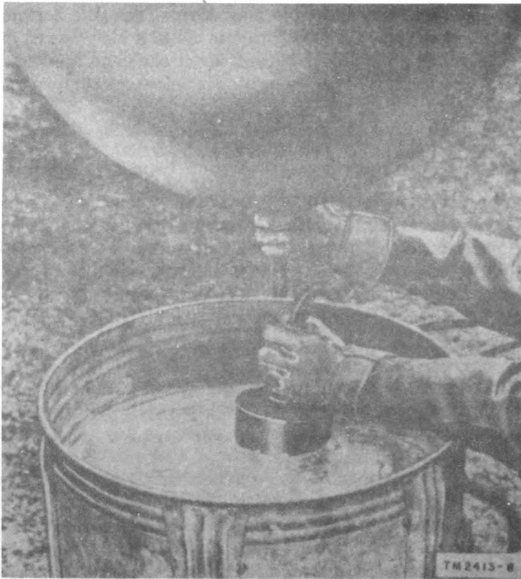
Figure 8. Hydrogen Generator ML-303/TM in operation.
