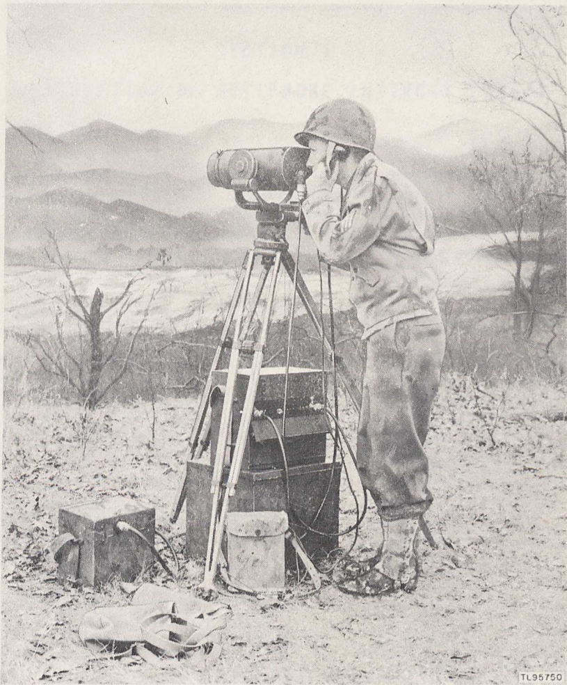
Figure 1. Aligning Optiphone AN/TVC-1 (XO-1).
