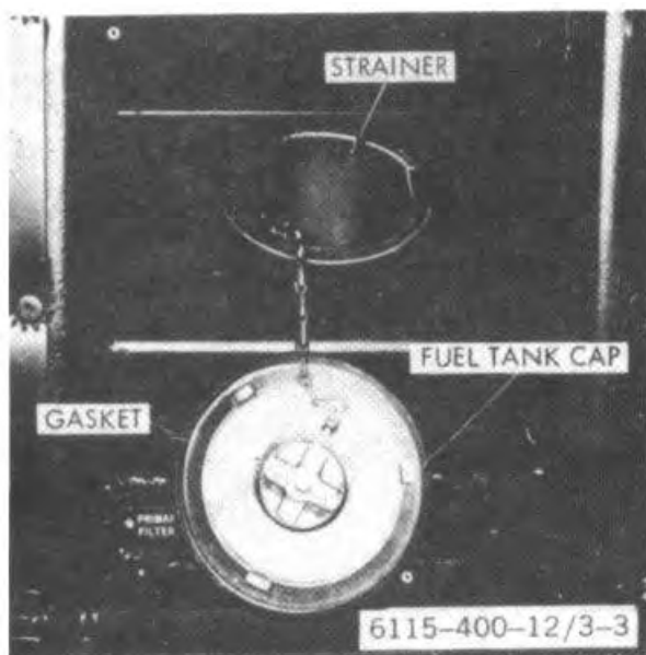
Figure 3-3. Fuel Tank service.
