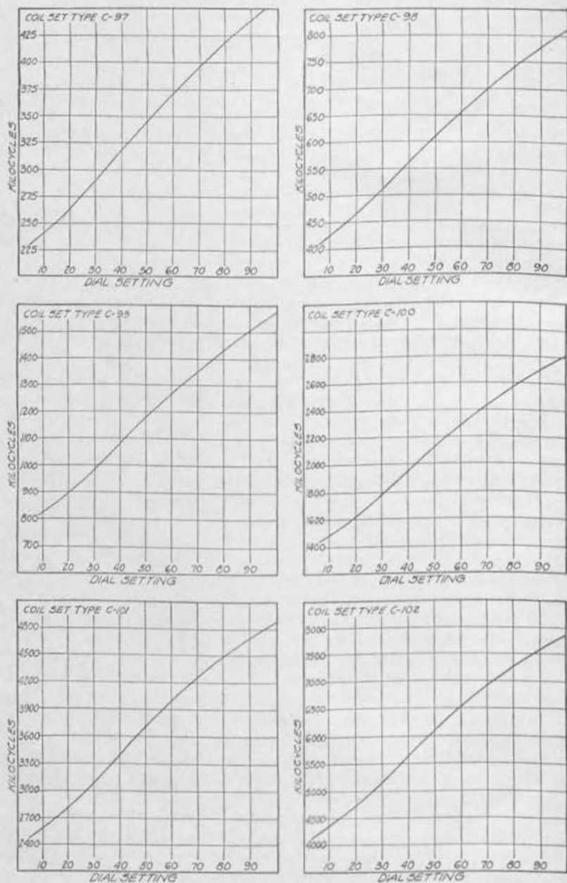
FIGURE 14.—Frequency calibration, radio receiver, type BC-AA-179.
