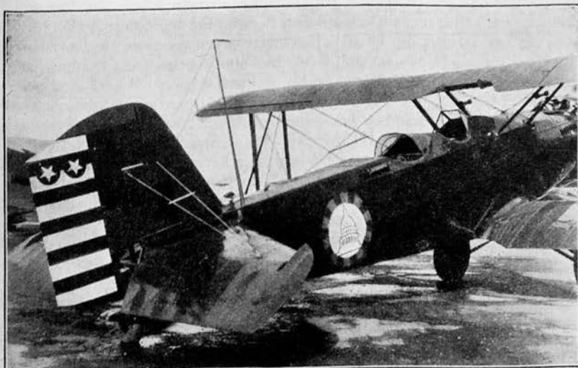
FIGURE 29.—Antenna installation on observation airplane.
