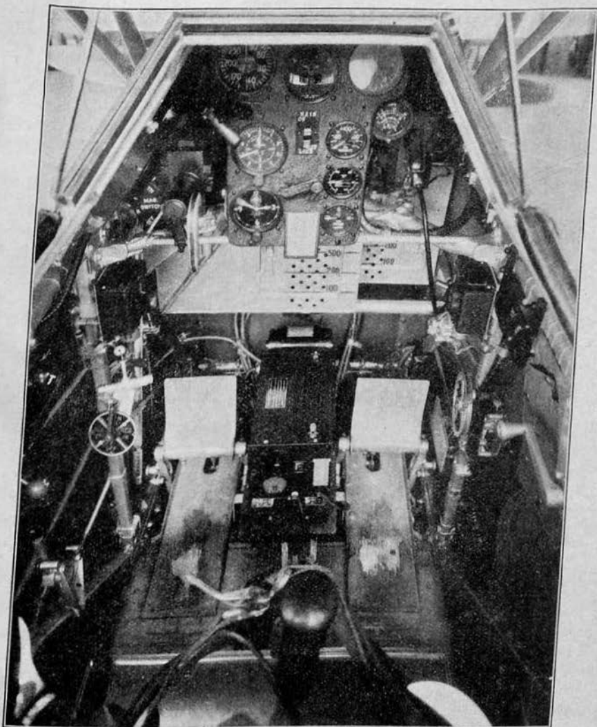
FIGURE 19.—Location of transmitter in pursuit airplane.
