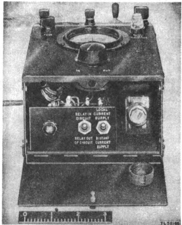
Figure 76. Line Unit BE-77-A, door open.
