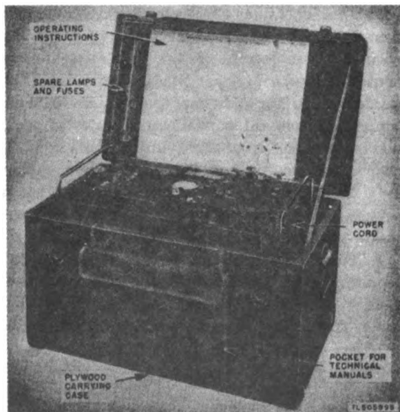
Figure 155. Repeater TG-30 (Terminal, Telegraph) ready for operation.
