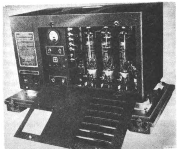
Figure 118. Rectifier RA-43-B, front view.
