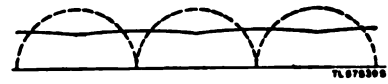
Figure 207. Output waveshapes of simplified rectifier circuit with choke coil and capacitors connected.
