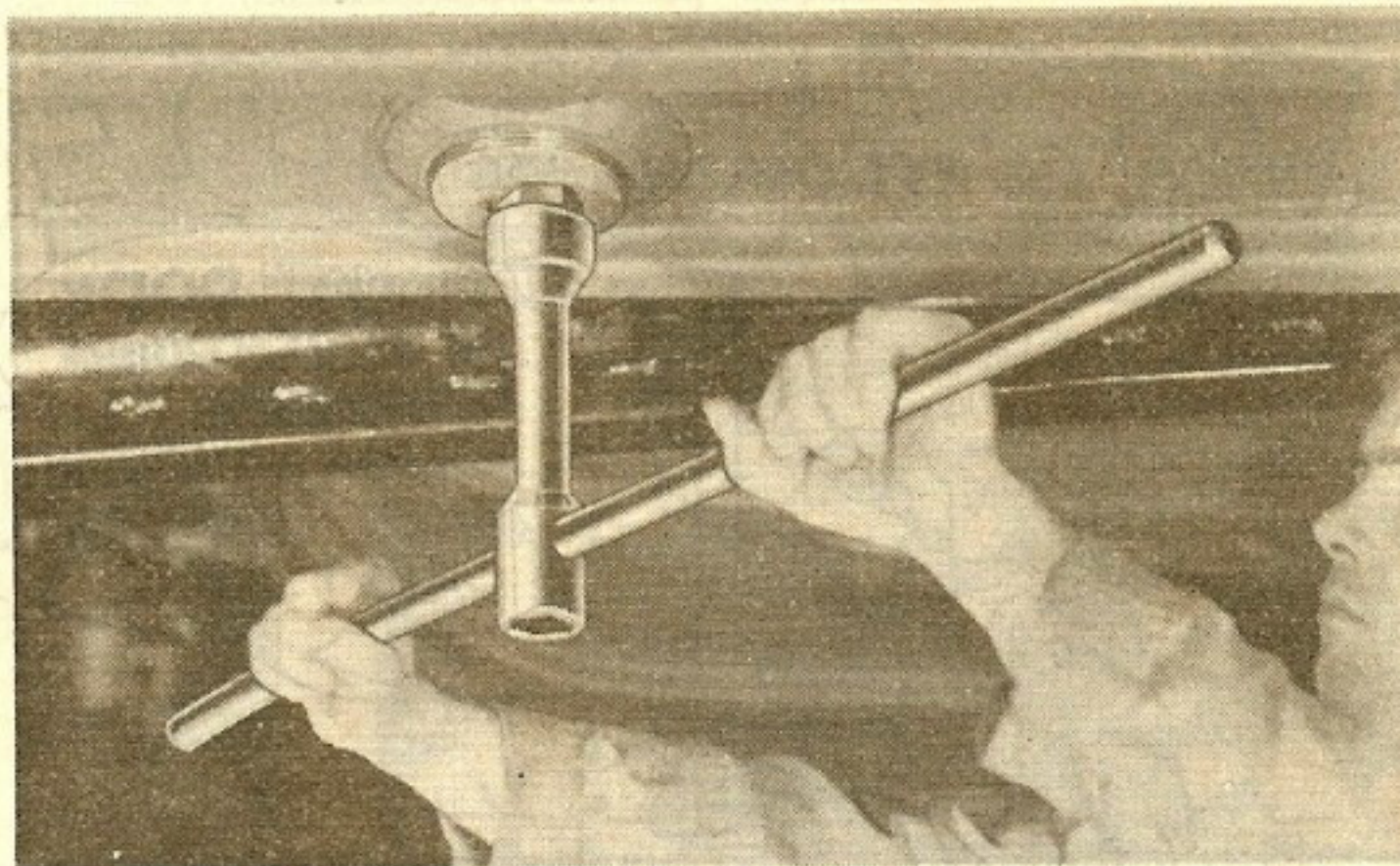
Fig. 3—The wheel wrench and adapter removes hull drain-plugs without trouble. Don't use an adjustable-end wrench.
