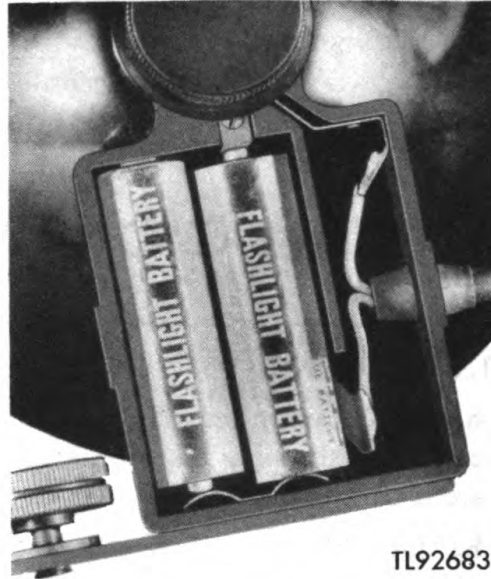
Figure 6. Batteries in place in battery case of synchronizer.
