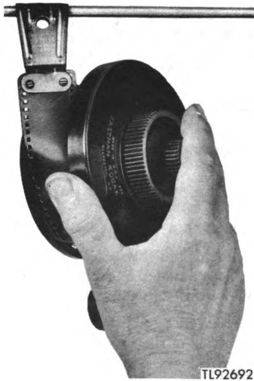
Figure 15. Removal of film from reel.
