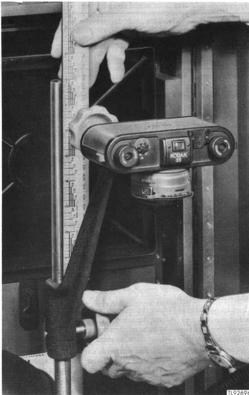
Figure 19. Measuring to set distance from lens to subject.
