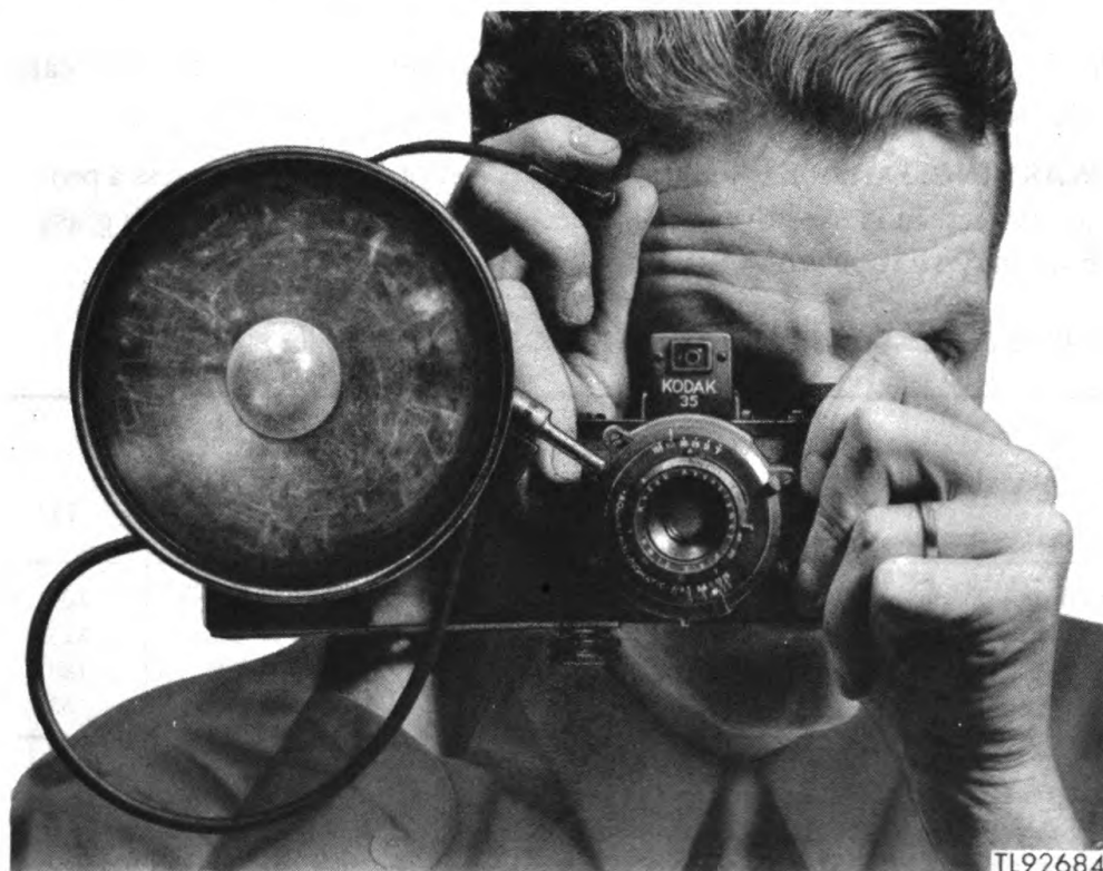
Figure 7. Camera PH-324 in operating position with synchronizer attached.
