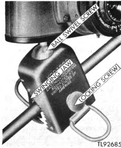
Figure 8. Clamp (Kodapod) in operating position with Camera PH-324 attached.
