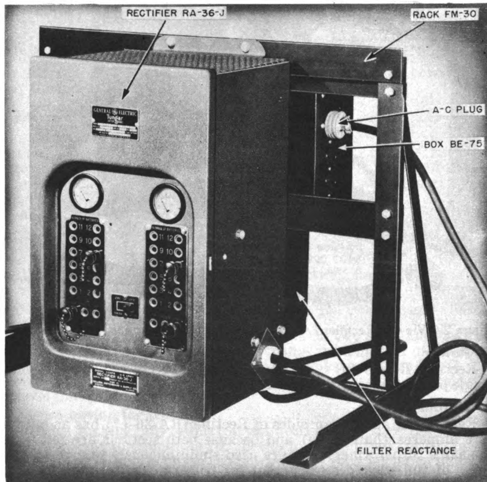
Figure 1—Exterior view of Rectifier RA-36-(* )
