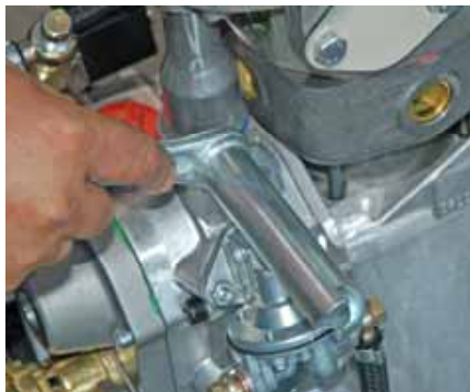
Fig. 32: Example: Adjusting the automatic decompression on the starting handle with the adjusting spanner
