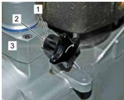
Fig. 29: Example: automatic decompression with star knob
