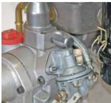
Fig. 30: Example: automatic decompression with lever
