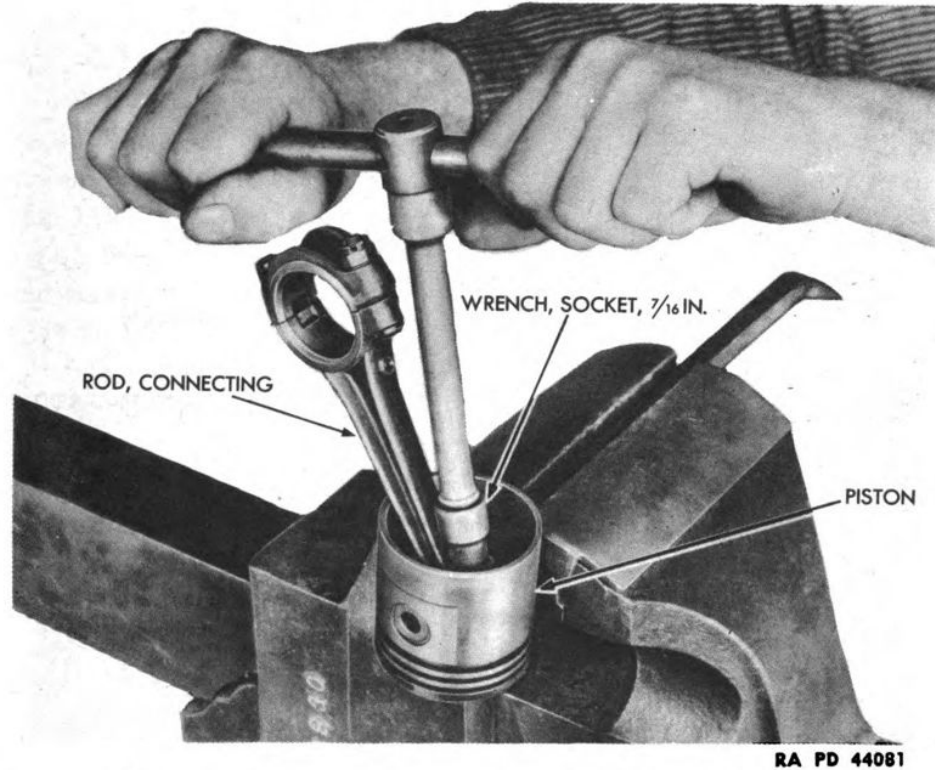
Figure 178 — Tightening Connecting Rod Piston Pin Lock Screw
