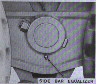
REFERENCE 81: Clean fittings (2) and apply lubricant through fittings.
