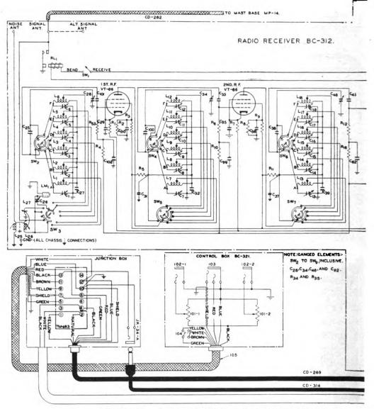
FIGURE 12.—Radio set SCR-210-A, schematic diagram, including
