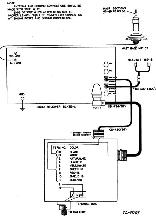
FIGURE 18.—Radio set SCR-210-G, cording diagram.
