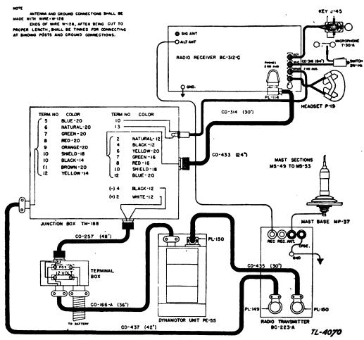
FIGURE 35.—Radio set SCR-245-L, cording diagram.
