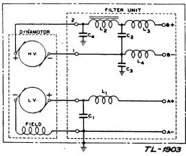
FIGURE 54.-Dynamotor DM-17-A, schematic diagram:
