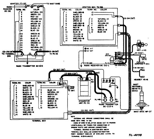
FIGURE 27.—Badio set SCR-245-E, cording diagram.
