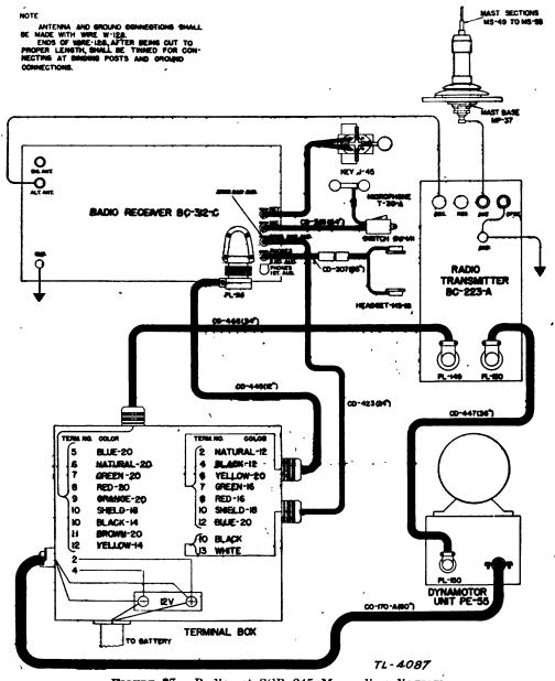
FIGURE 87.—Radio set SCR-245-M, cording diagram.
