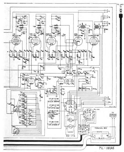
complete schematic diagram of radio receiver BC-312.
