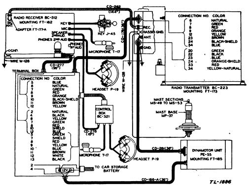
FIGURE 23.—Radio set SCR-245-C, cording diagram.
