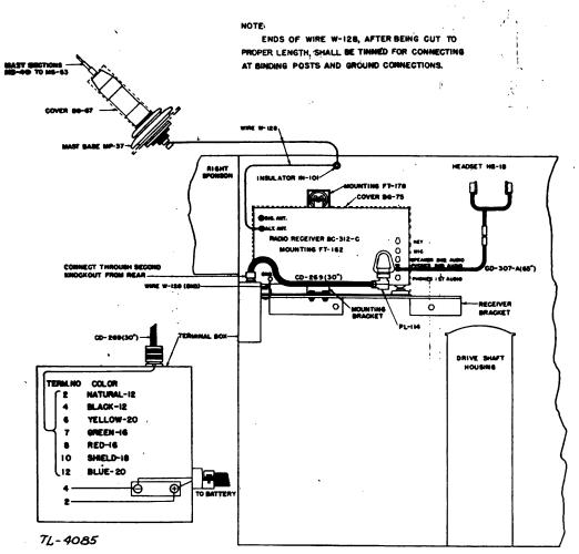
FIGURE 14.-Radio set SCR-210-C, cording diagram.
