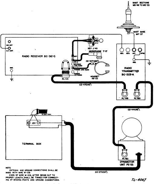
FIGURE 39.—Radio set SCR-245-P, cording diagram.
