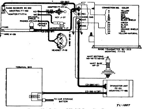
FIGURE 25.—Radio set SCR-245-D, cording diagram.
