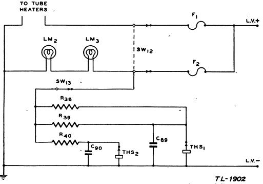
FIGURE 53.—Radio receiver BC-312, low-voltage circuits, functional diagram.
