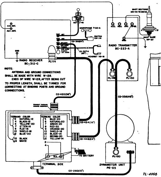
FIGURE 38.-Radio set SCR-245-N, cording diagram.
