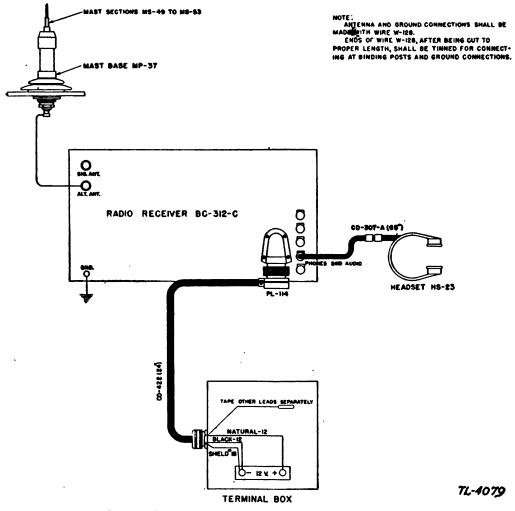
FIGURE 20.-Radio set SCR-210-J, cording diagram.
