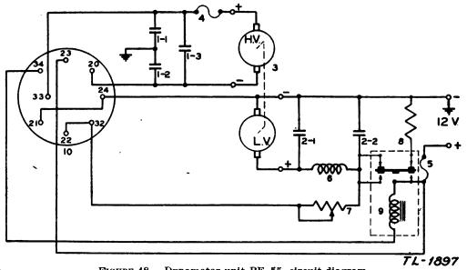
FIGURE 48.—Dynamotor unit PE-55, circuit diagram.
