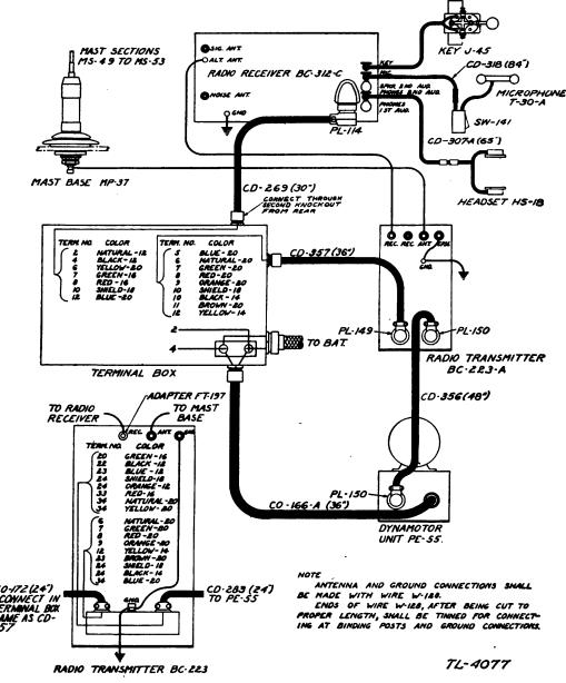
FIGURE 28.-Radio set SCR-245-F, cording diagram.
