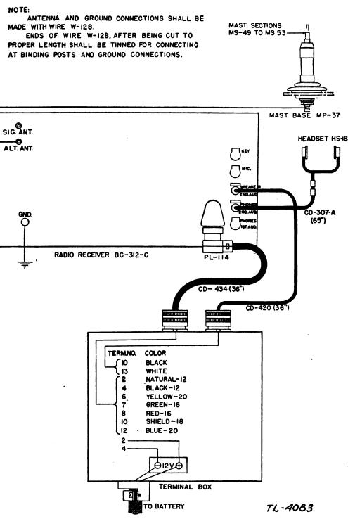
FIGURE 16.—Radio set SCR-210-E, cording diagram.
