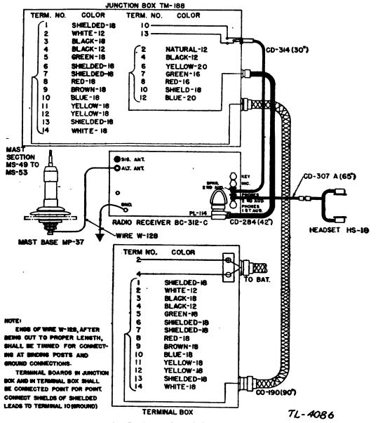
FIGURE 13.—Radio set SCR-210-B, cording diagram.
