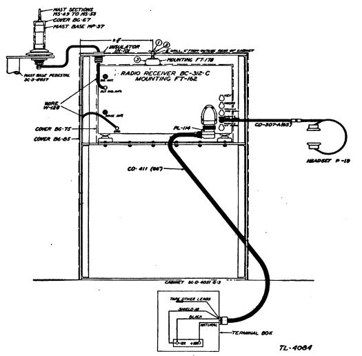
FIGURE 15.---Radio set SCR-210-D, cording diagram.
