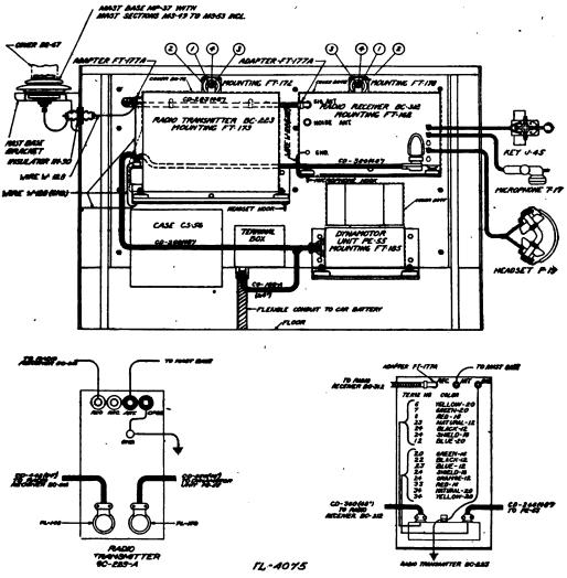
FIGURE 30.---Radio set SCR-245-H, cording diagram.
