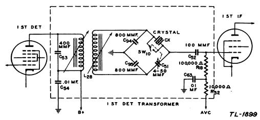
FIGURE 51.---Radio receiver BC-312, crystal filter operation, functional diagram.
