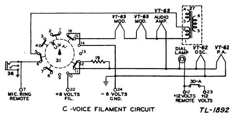
FIGURD 47.—Radio transmitter BC-223 or radio transmitter BC-223-A, filament circuit, cw, tone, voice.
