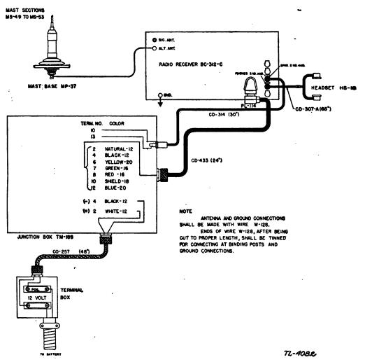
FIGURE 17.-Radio set SCR-210-F, cording diagram.
