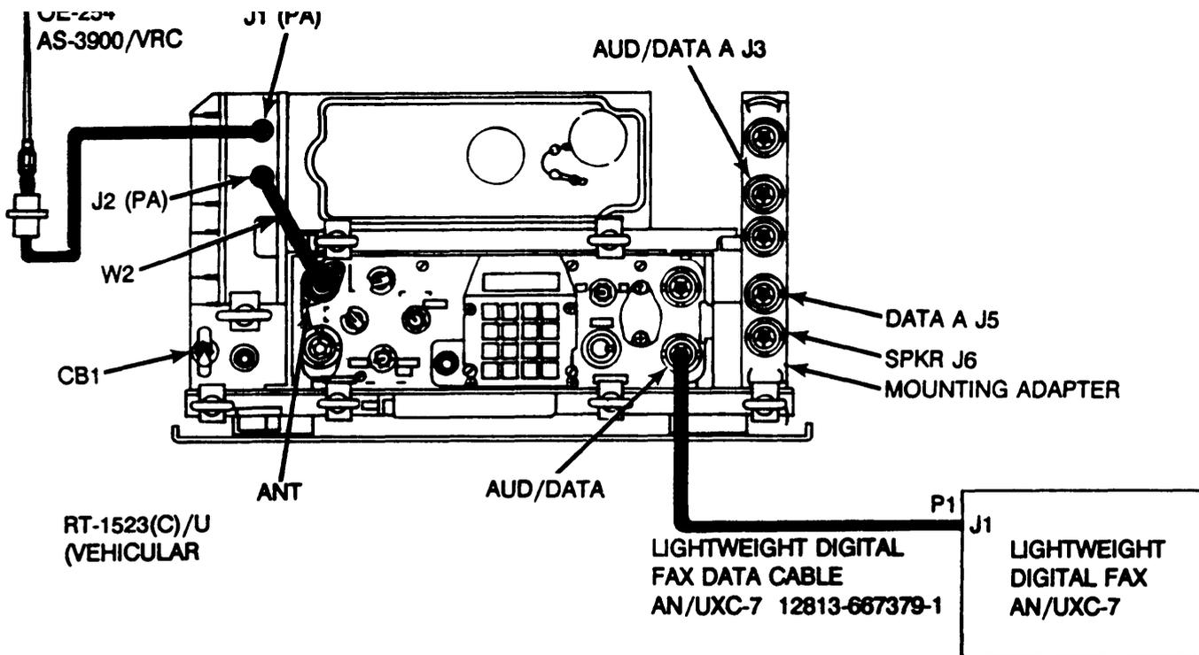
Figure 1. Cabling for Lightweight Digital FAX TO SINCGARS Radio Set
