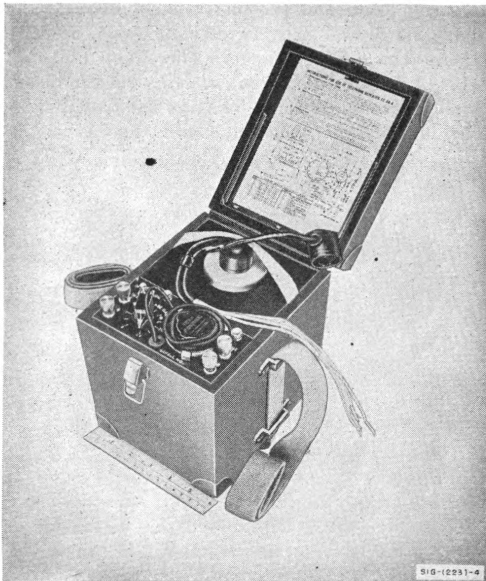
Figure 4. Telephone Repeater EE-89-A.
