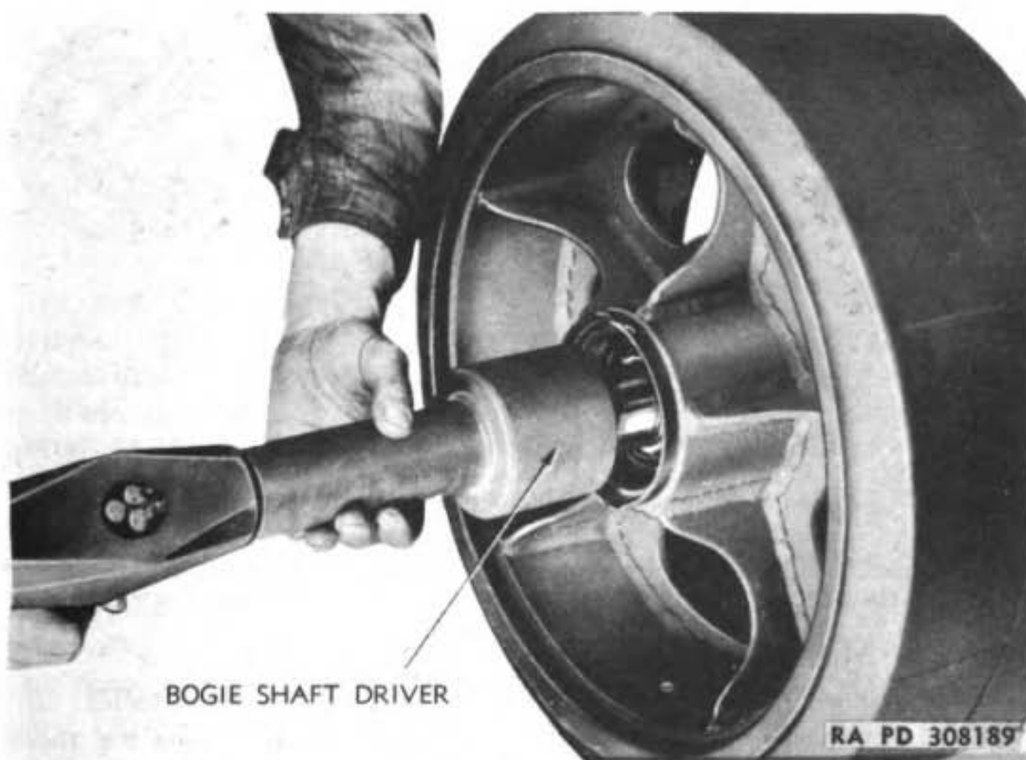
Figure 87 – Driving Shaft and Bearings From Bogie Wheel, Using Tool (41-R-2378-598)
