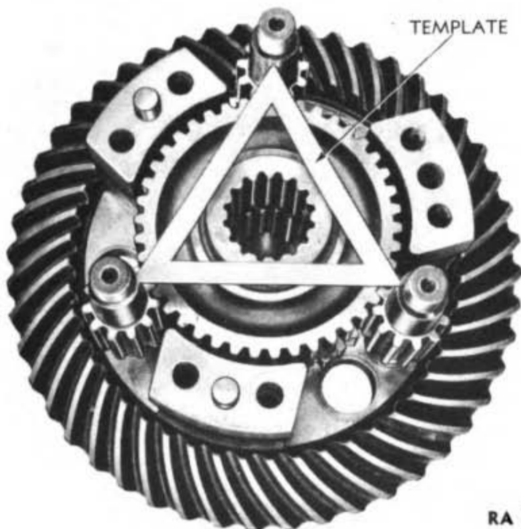
Figure 55 — Position of Differential Pinion Shafts
