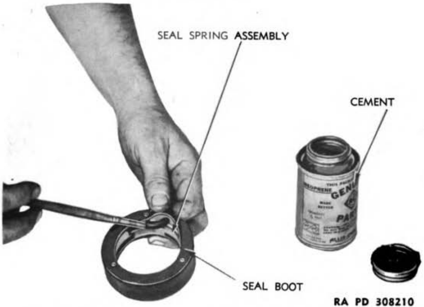
Figure 108 – Cementing Seal Boot to Spring Assembly
