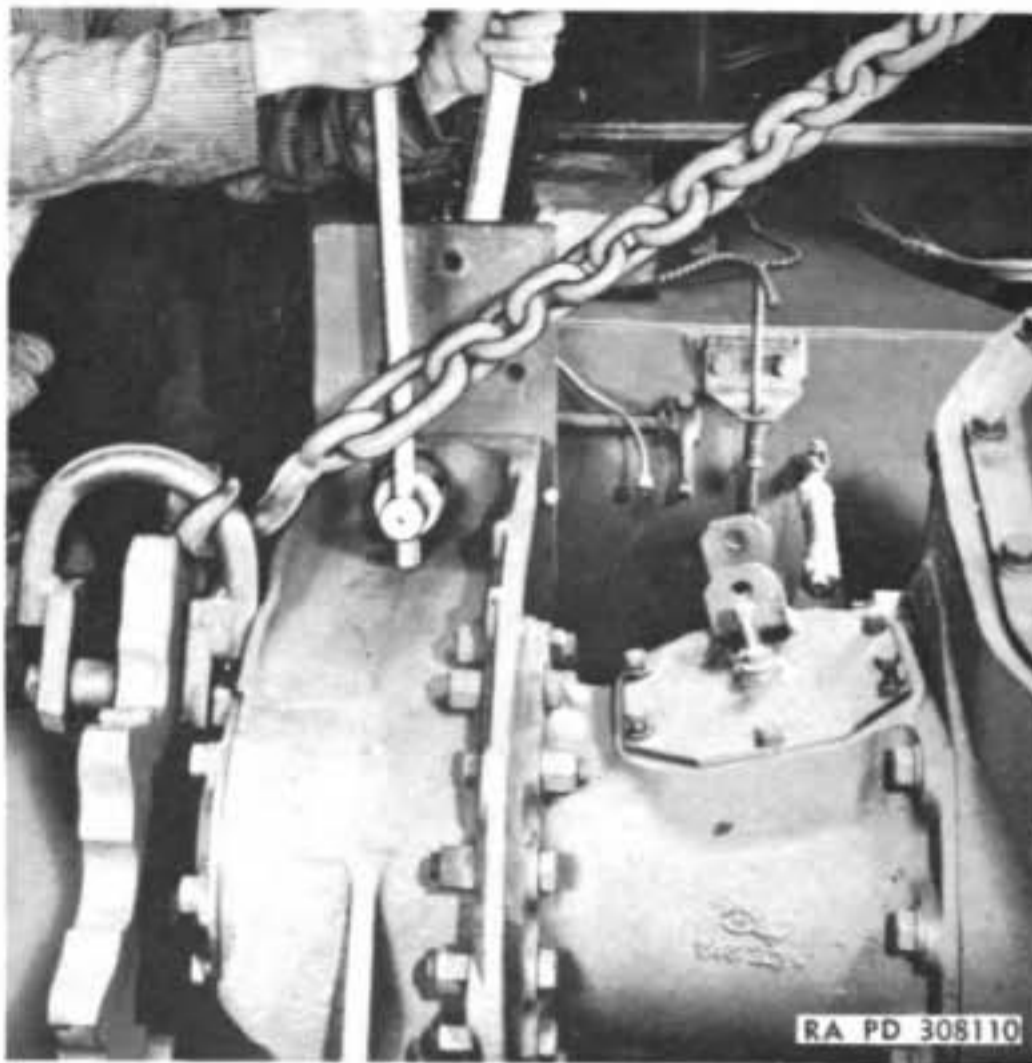
Figure 10—Removing Upper Attaching Bolts
