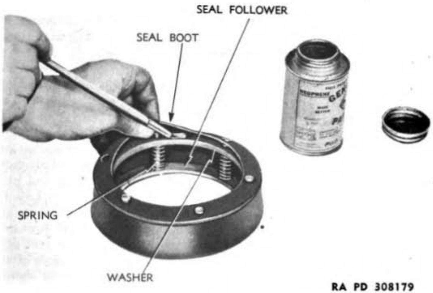
Figure 77 – Cementing Seal Boot to Follower
