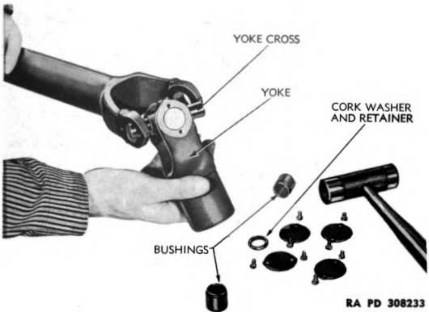
Figure 131 – Removing Yoke and Cross From Shaft
