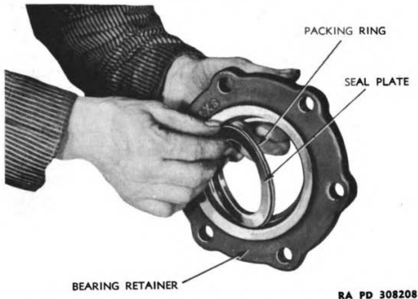
Figure 106 – Installing Oil Seal Plate in Bearing Retainer
