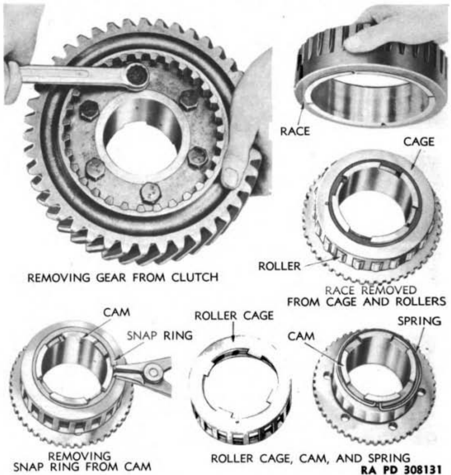
Figure 31 — Disassembly of Overrunning Clutch Assembly
