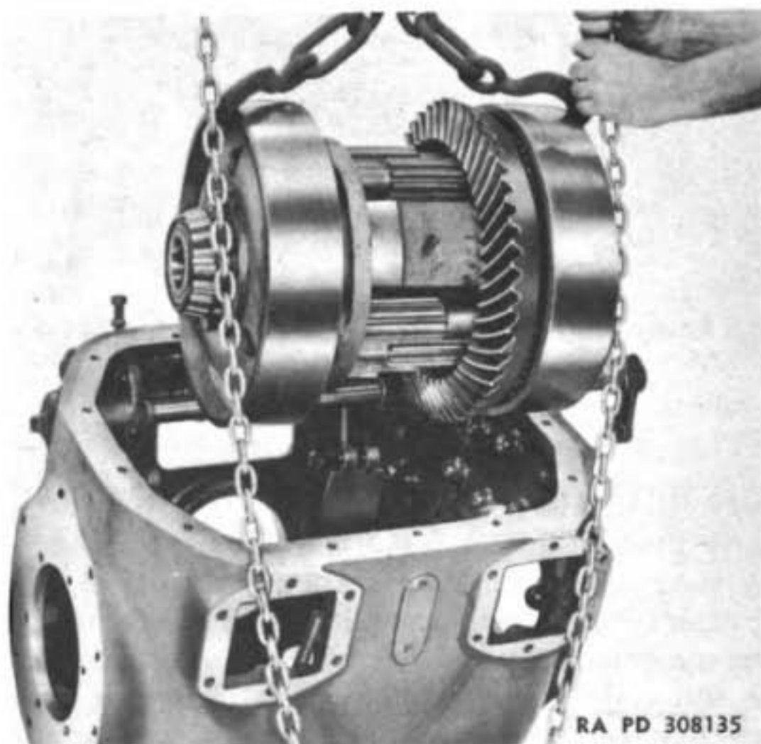
Figure 35 – Differential Assembly Removed
