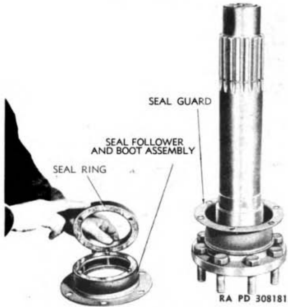
Figure 79 – Installing Inner Seal Ring on Follower
