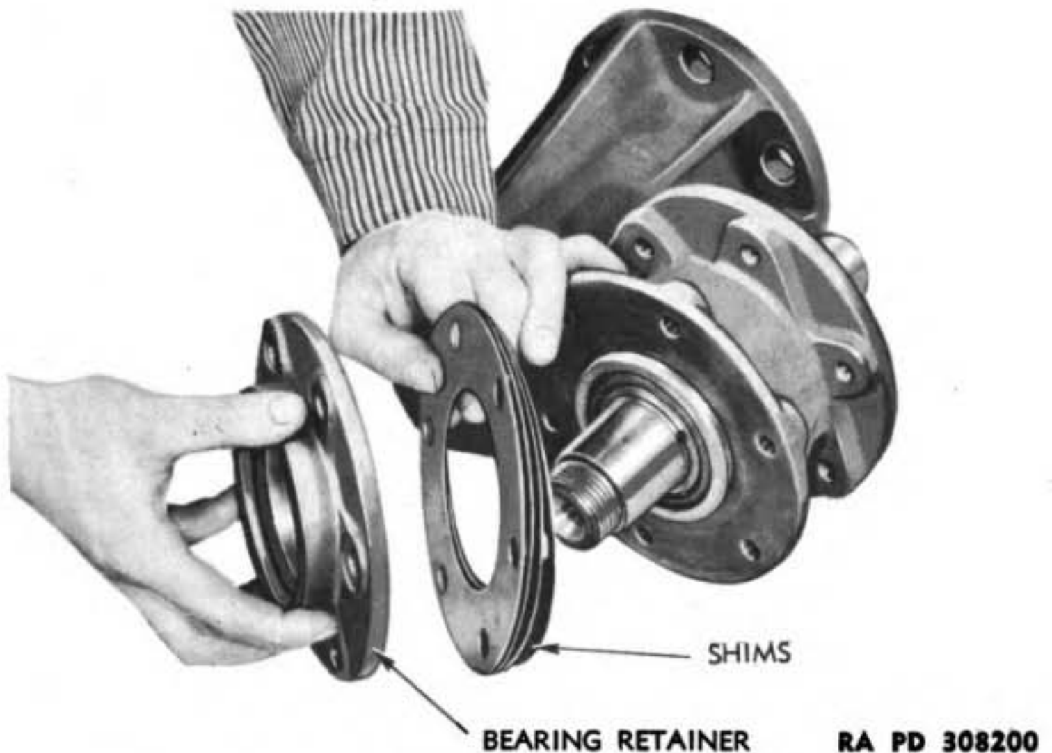
Figure 98 – Installing Shims and Bearing Retainers
