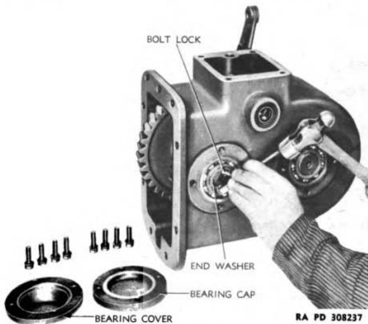
Figure 135 – Straightening Bolt Lock To Remove Drive Shaft
