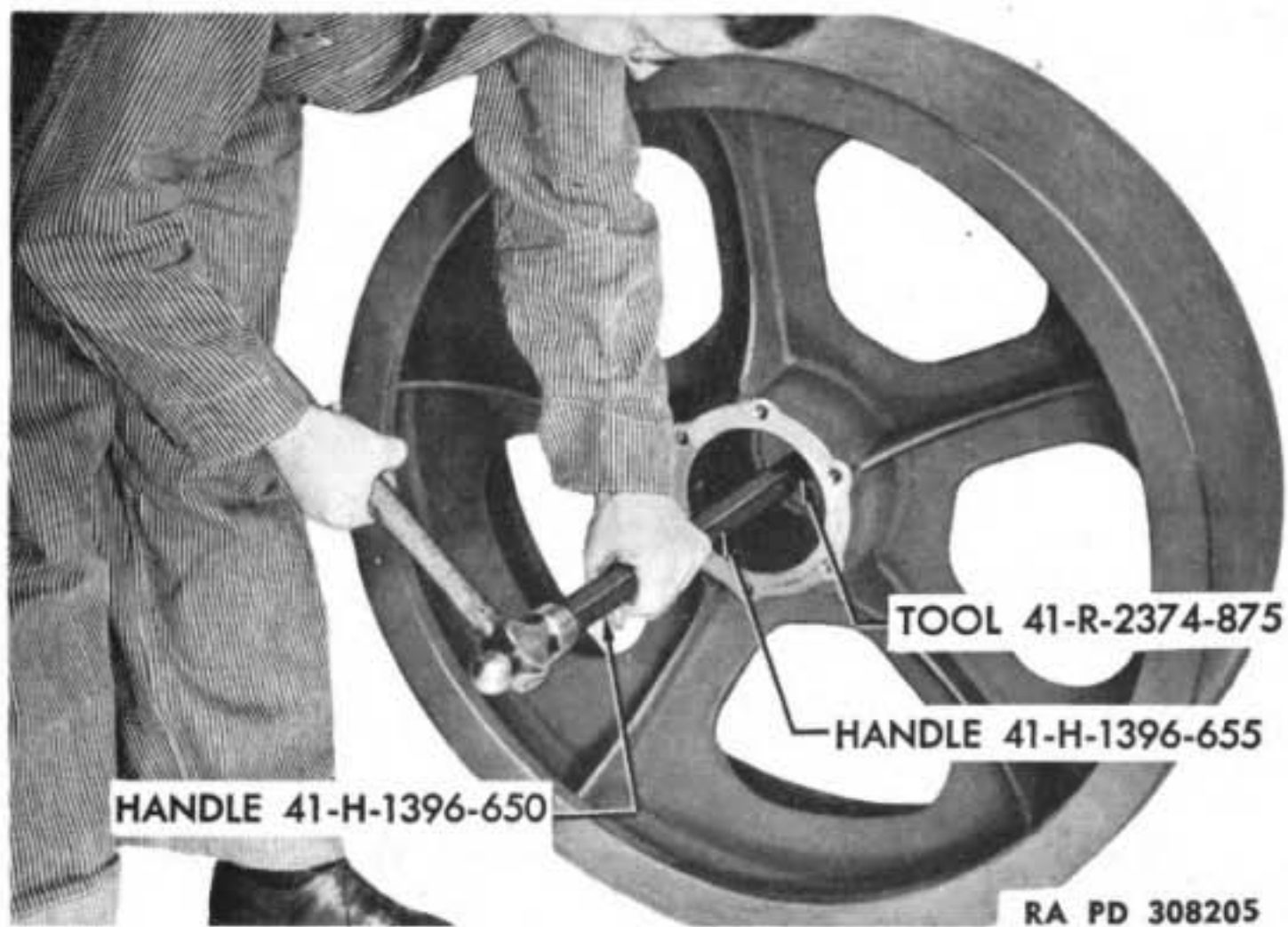
Figure 103 – Removing Second Idler Shaft Bearing Cup
