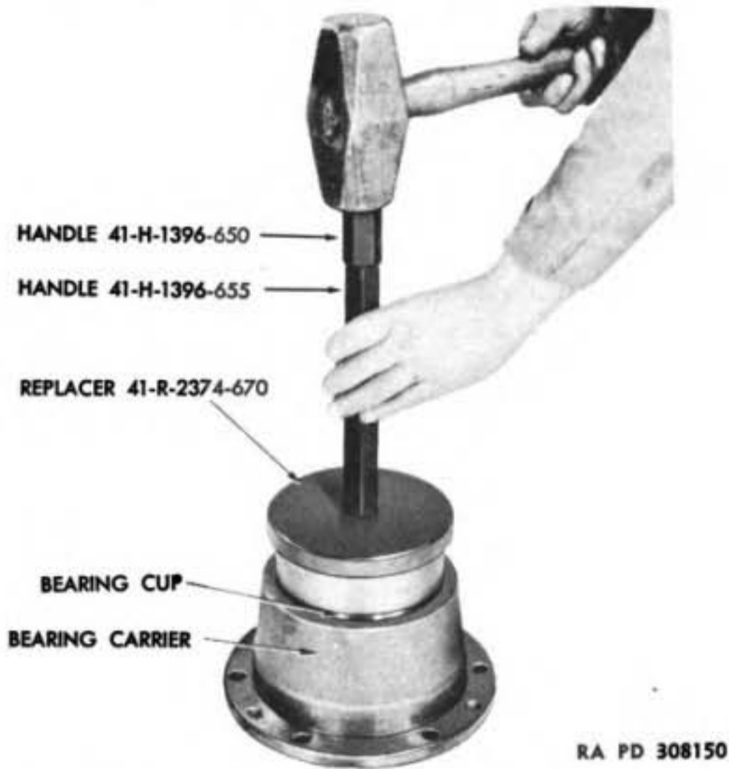
Figure 50 – Installing Differential Bearing Cup
