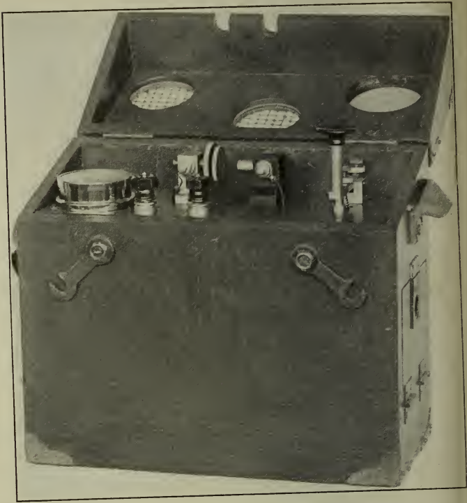
Fig. 1—Type BC-18 Set Box and Operating Panel of the Type SCR-74 Set
