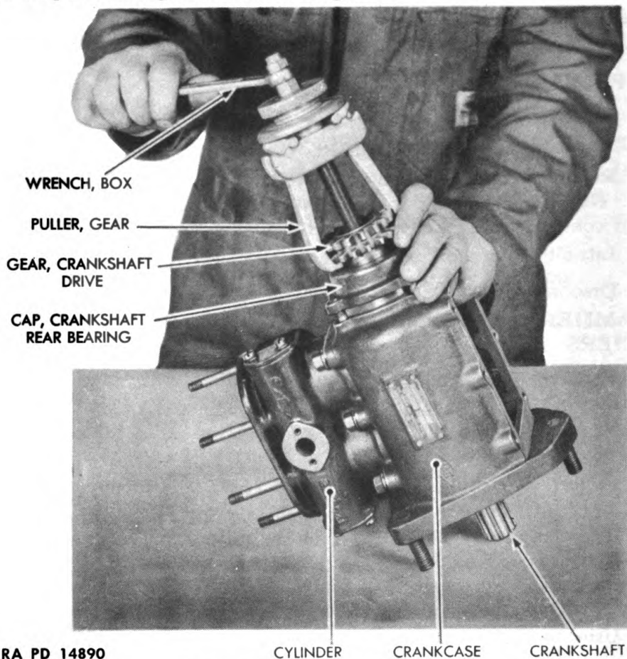
Figure 36—Removing Crankshaft Drive Gear
