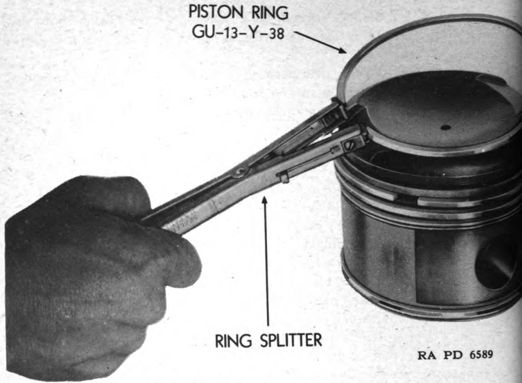
FIGURE 74—Removing piston rings.
