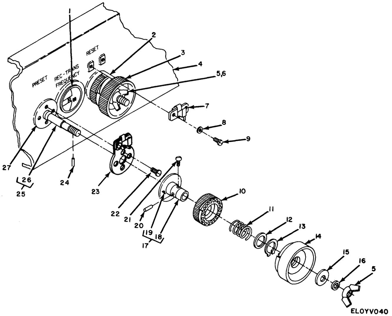
Figure 3. Panel Assembly (A30), Knob Assembly.
