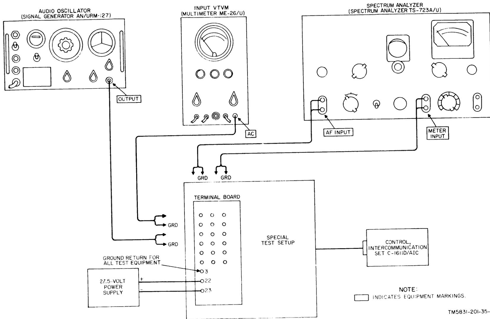
Figure 5-1. Frequency response, a/c, and distortion test setup.
