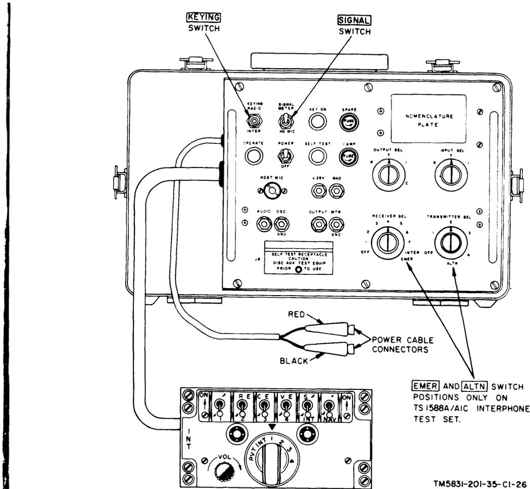
Figure 3.1-1. Control, Intercommunication Set C-1611D/AIC and Test Set, Radio TS-1588A/AIC control panels
