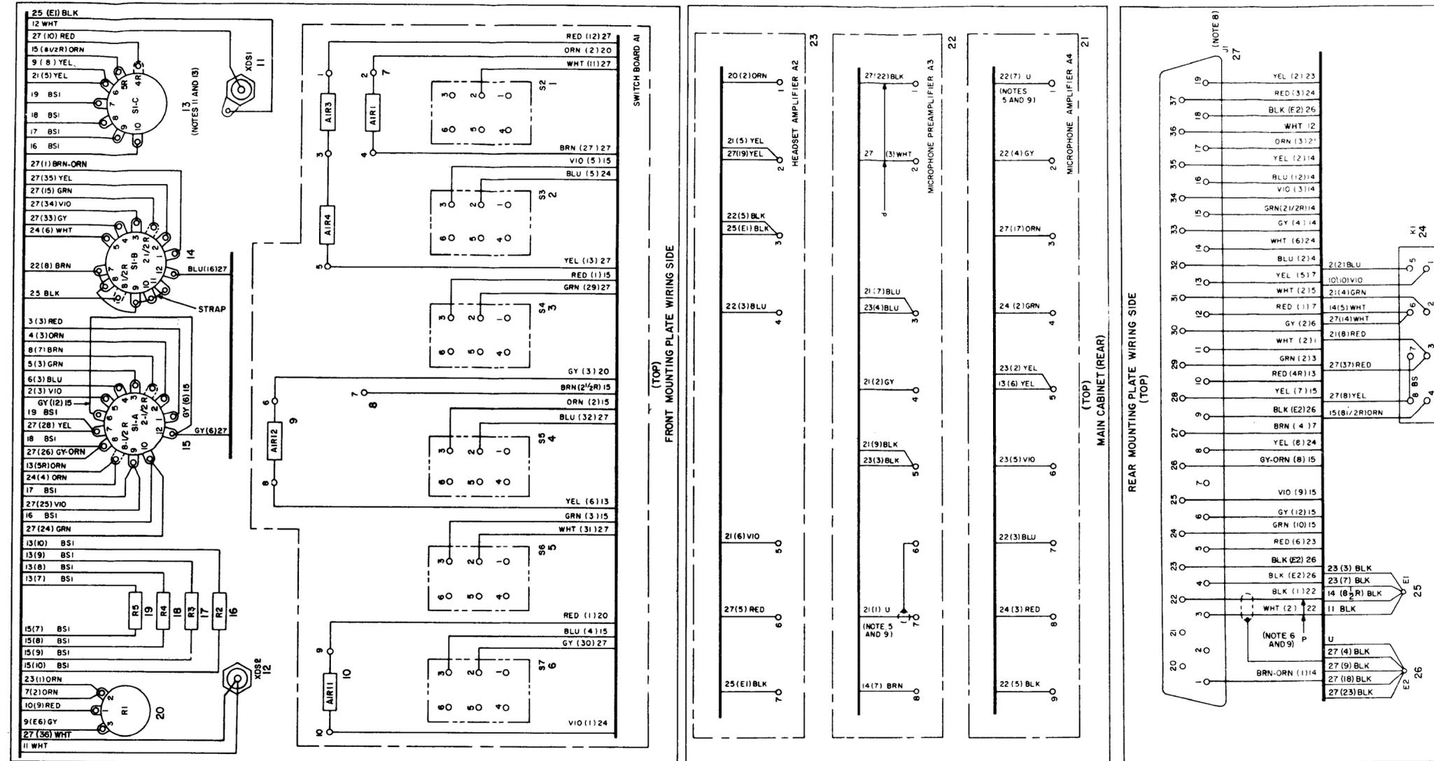
Figure 7-4. Control, Intercommunication Set C-1611D/AIC wiring diagram, less printed wiring and circuit elements for boards A1, A2, A3, and A4.
