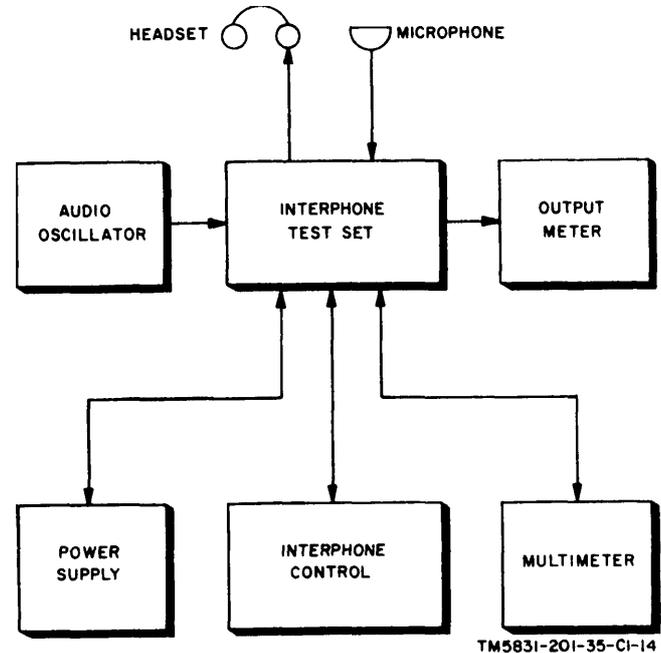
Figure 3.1-2. Control, Intercommunication Set C-1611D/AIC test setup, block diagram.
