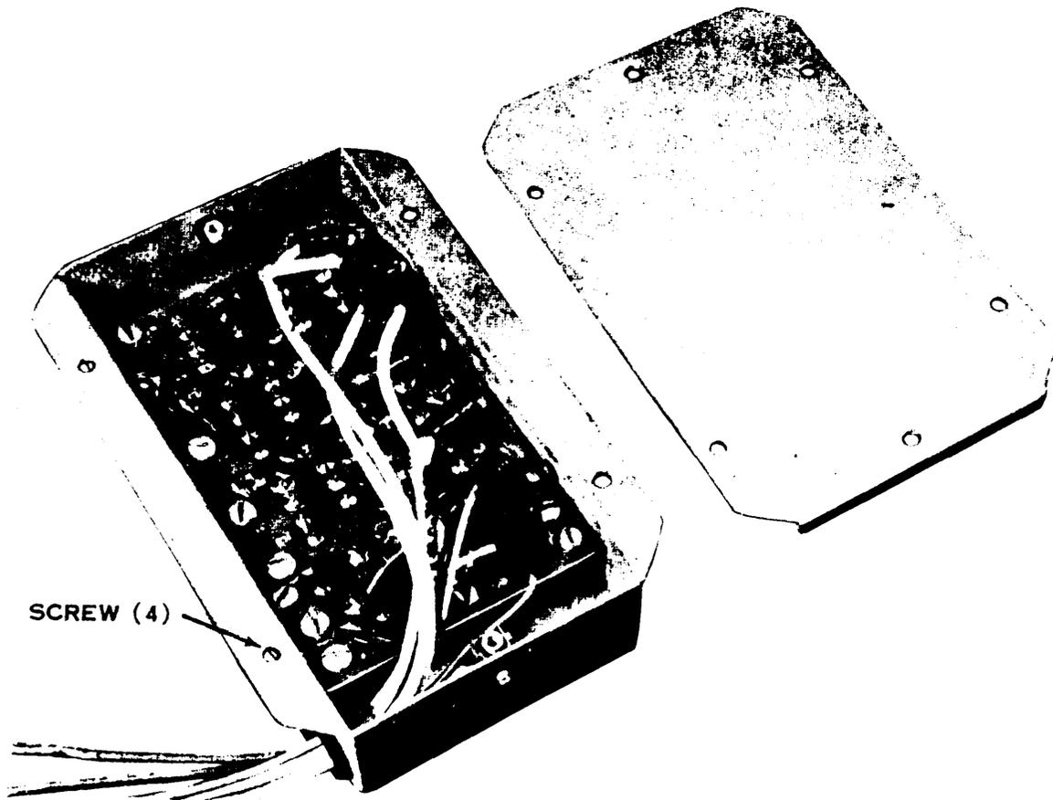
Figure 6-1. Discriminator, Discrete Signal MD-736/A cover removed.
