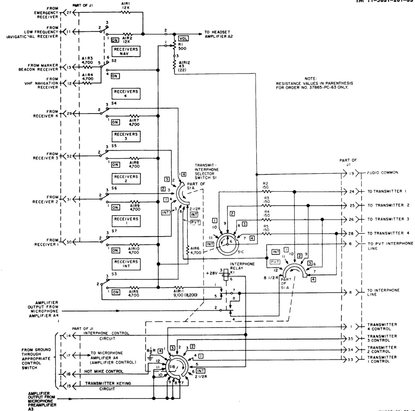
Figure 7-2. Control, Intercommunication Set C-1611D/AIC control circuits, simplified schematic diagram.
