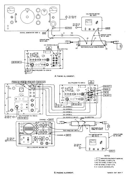
Figure 5-1. Panel 7A1, timing circuit alignment test setup.
