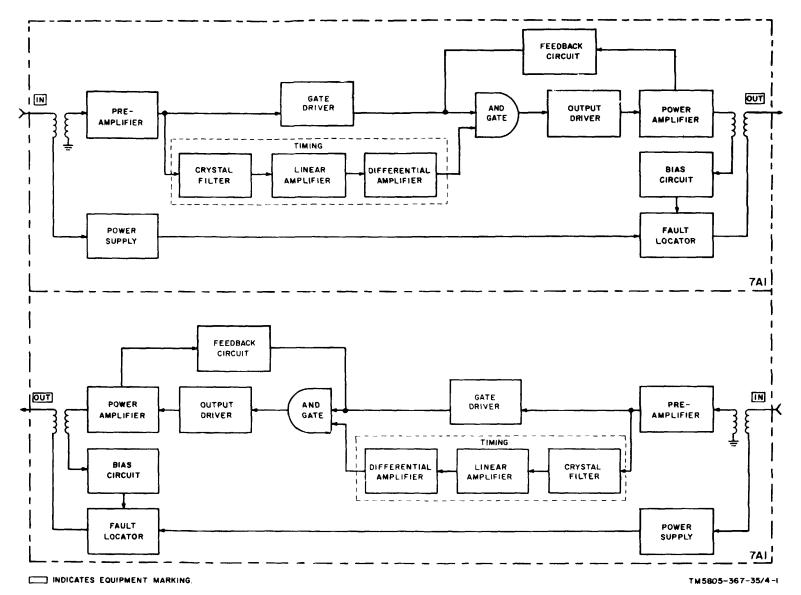
Figure 2-1. Restorer, Pulse Form, TD-206/G, block diagram.
