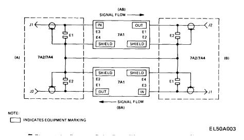
Figure 2-2. Restorer, Pulse Form TD-206/G, schematic diagram.
