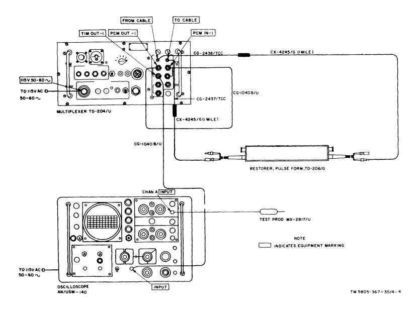
Figure 3-3. Panel 7A1, troubleshooting test setup.
