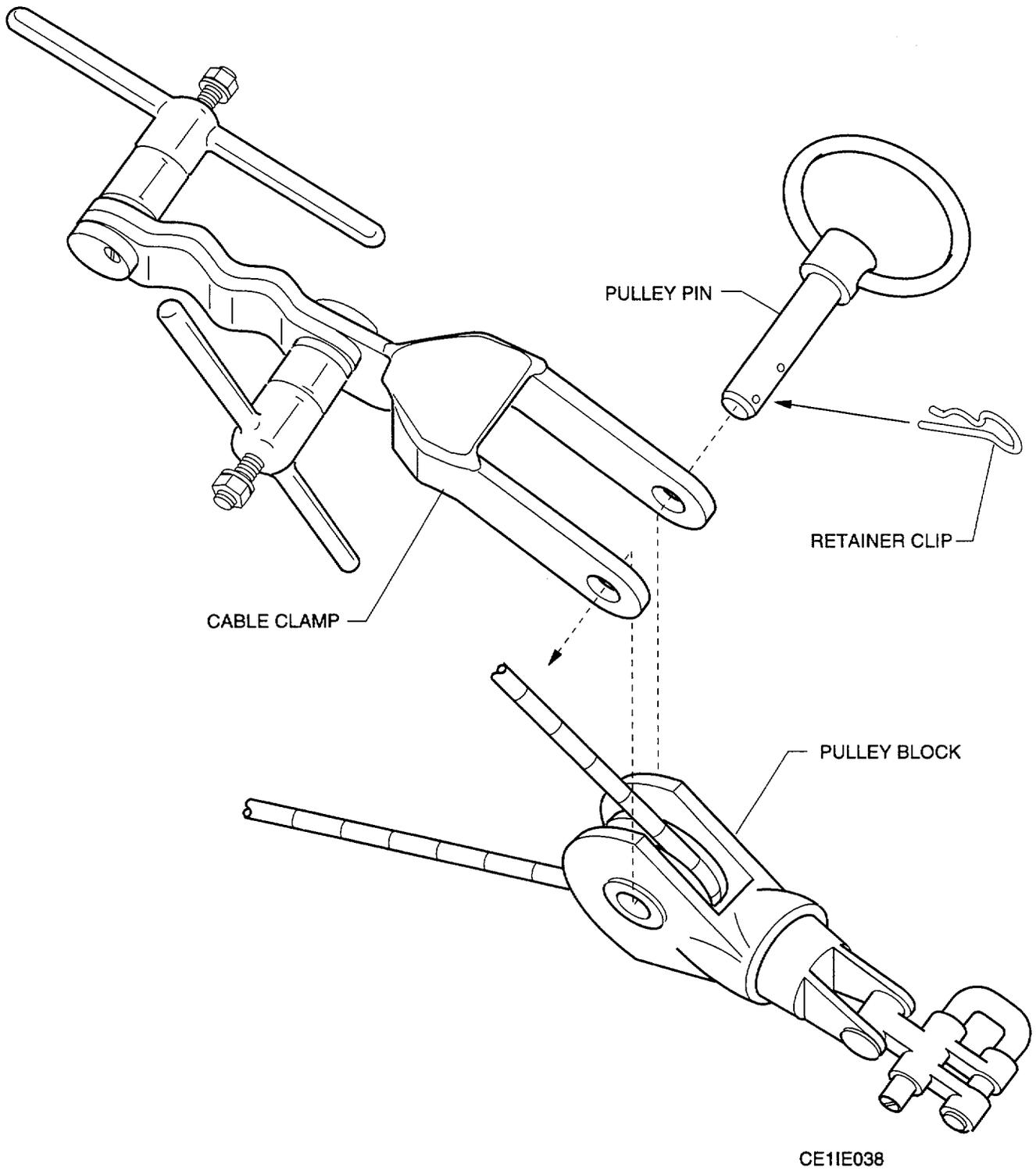
Figure 5-2. Cable Clamp Replacement
