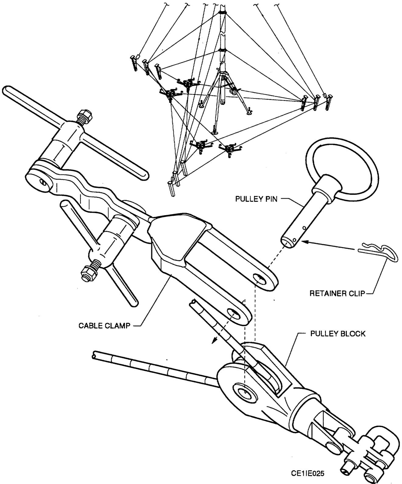
Figure 2-13. Pulley Block and Cable Clamp Installation
