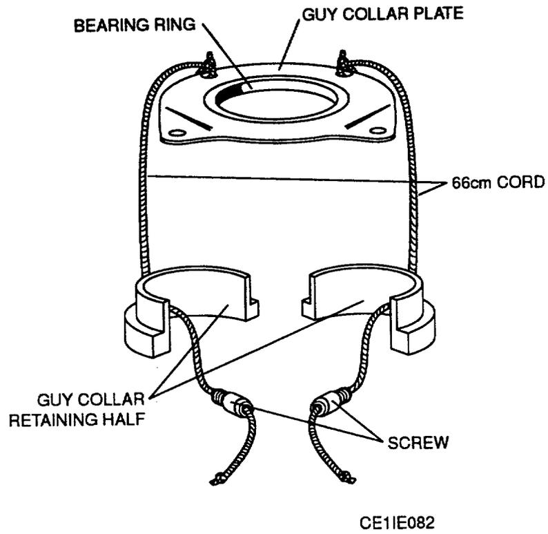
Figure 6-5. Guy Collar Removal and Replacement
