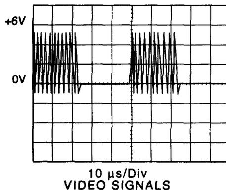
11. Set the oscilloscope Mode to AUTO and connect the probe to ICU1, pin 9.
