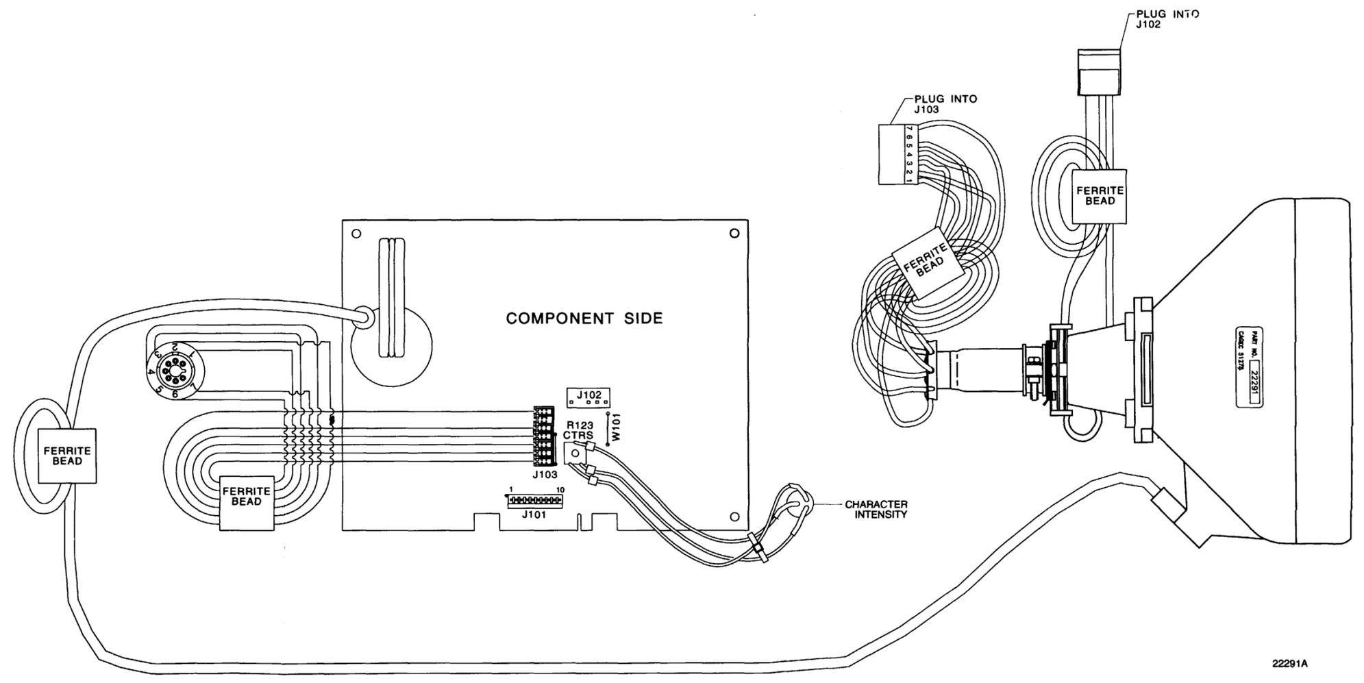
Figure FO-11. 1A2A9 Electron Tube Assembly Component Locator Diagram.
