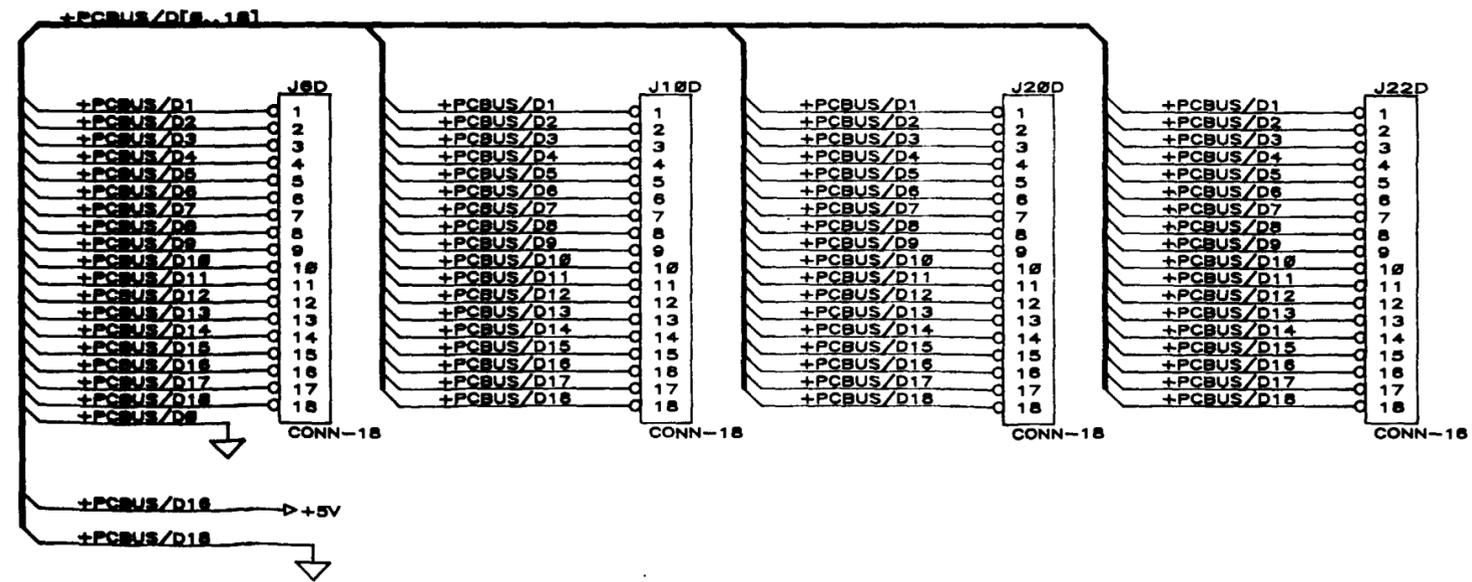
Figure FO-13. 1A2A11 CCA Backplane Component Locator & Schematic Diagram (Sheet 4 of 6)
