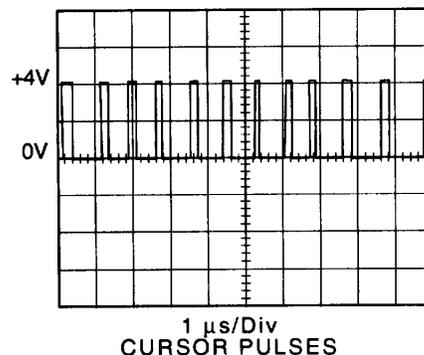
11. Refer to FO-13, sheet 1 of 6. Connect oscilloscope probe to output pins J26E-1 and J26E-2 in turn. Turn the B CURSOR knob and observe a pulse stream as shown.
