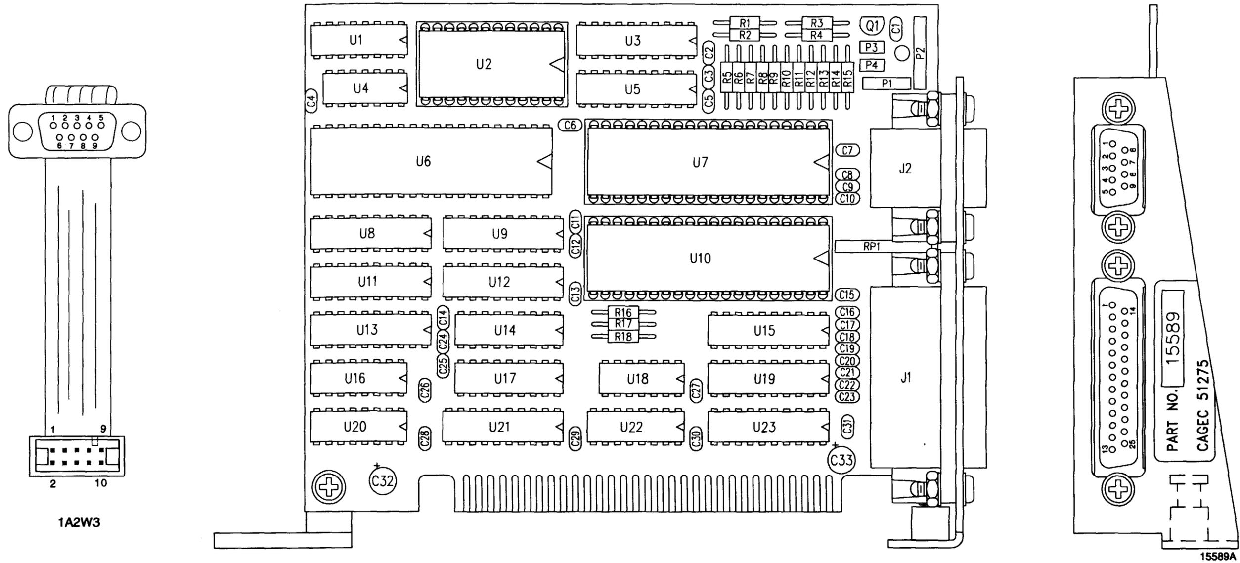
Figure FO-9. 1A2A7 Color Graphic Adapter CCA Component Locator Diagram.
