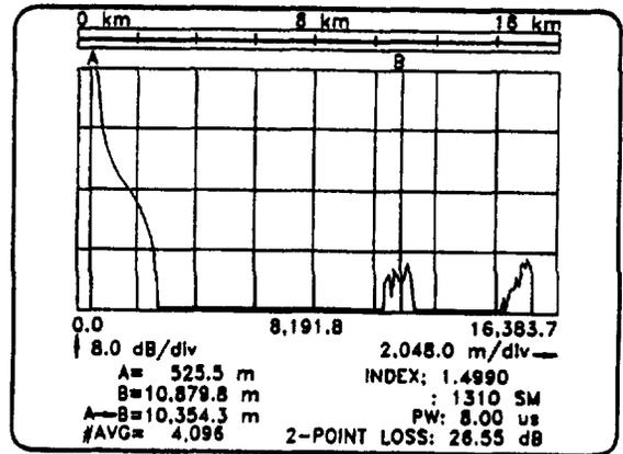
FOCUS GENERATED PULSE ABOVE NOISE FLOOR AFTER FAST SCAN
