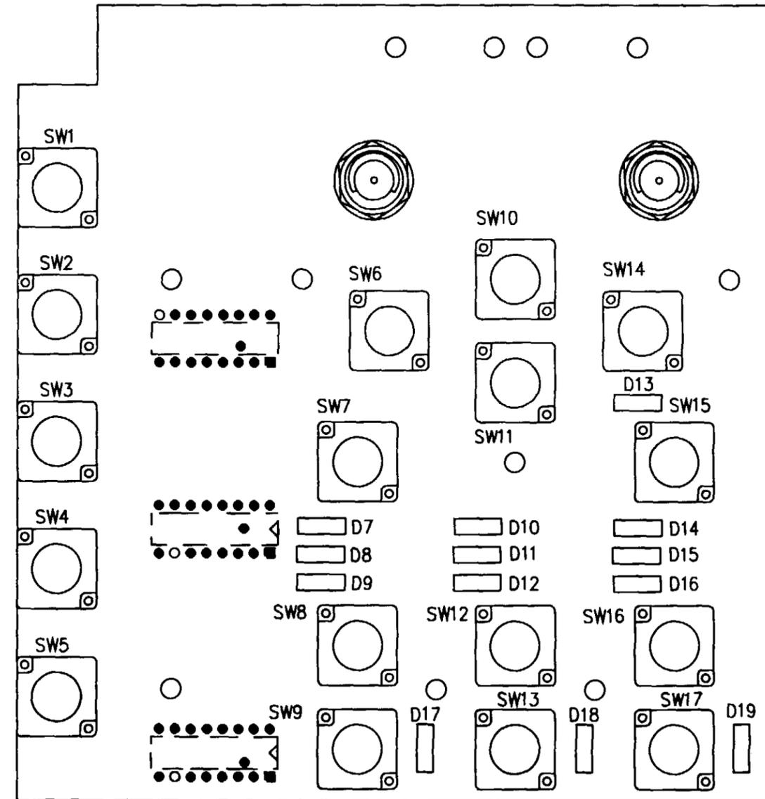
Figure FO-3. 1A2A1 Front Panel Interface CCA Component Locator Diagram.
