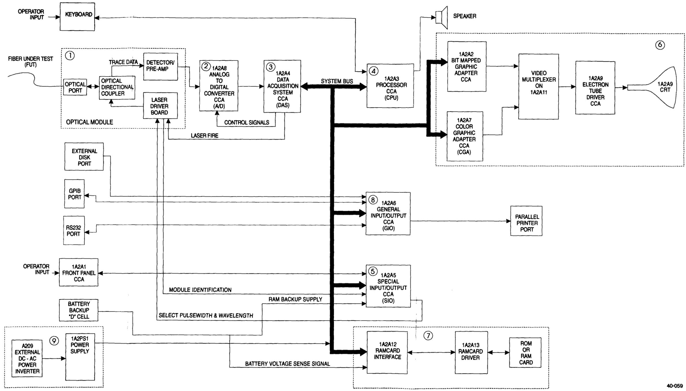
Figure FO-1. TS-4320 Functional Diagram.
