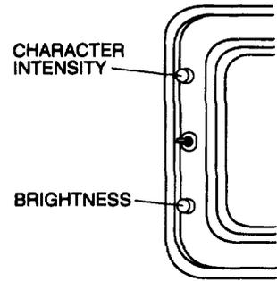
7. Adjust the Master Brightness trim pot R165, so the raster is just visible in a well lit room.
