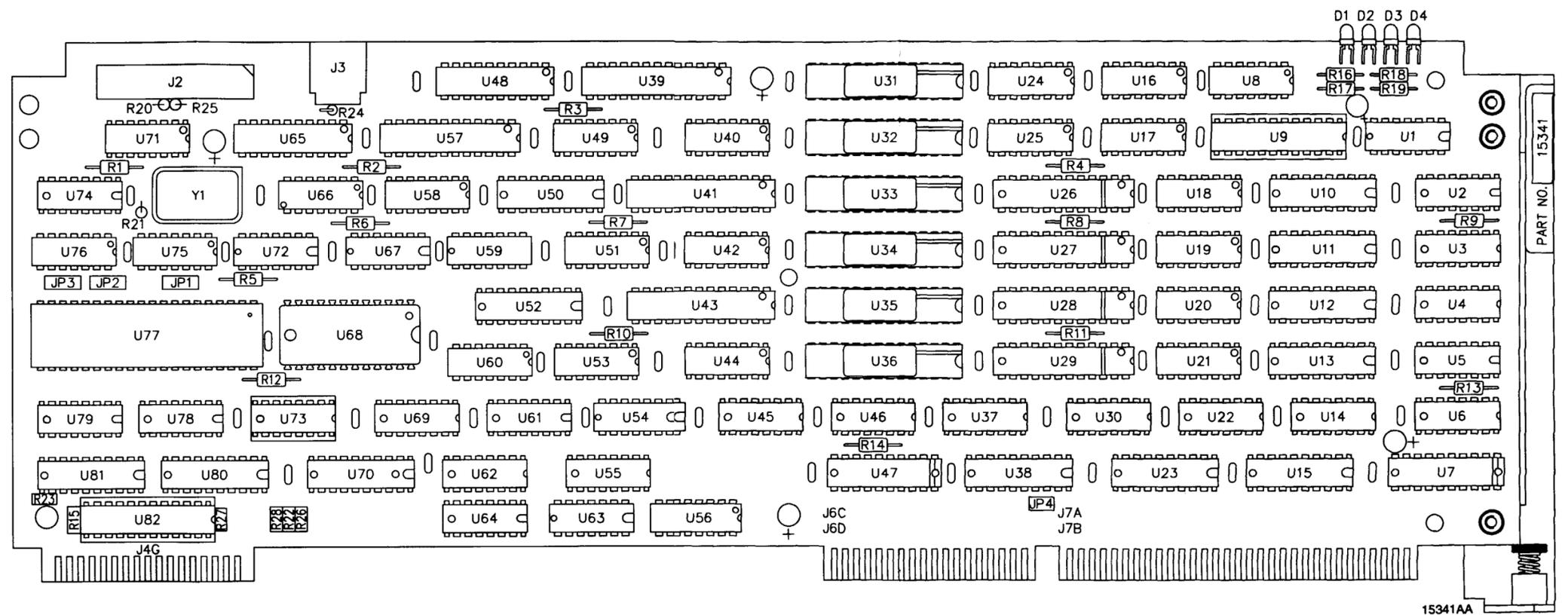
Figure FO-6. 1A2A4 DAS CCA Component Locator Diagram.
