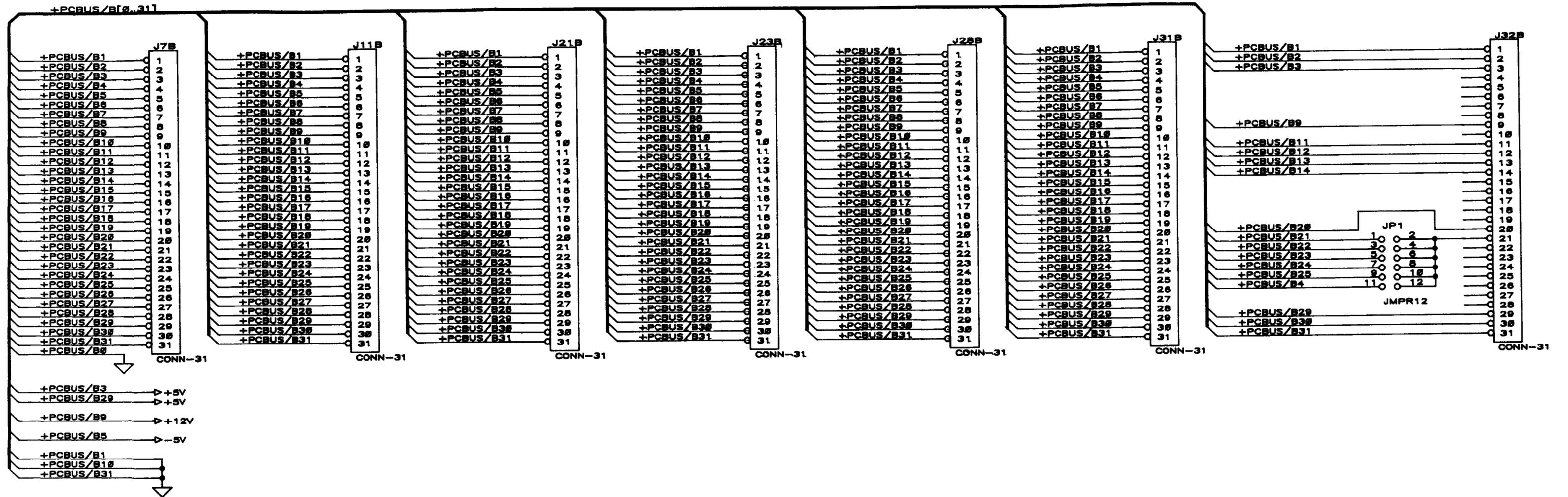
Figure FO-13. 1A2A11 CCA Backplane Component Locator & Schematic Diagram (Sheet 3 of 6).
