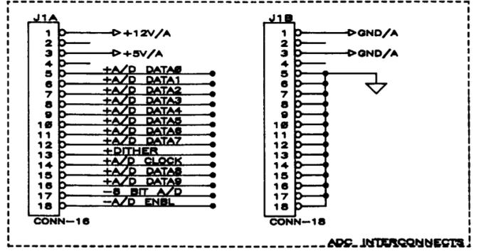
Figure FO-13. 1A2A11 CCA Backplane Component Locator & Schematic Diagram (Sheet 5 of 6).
