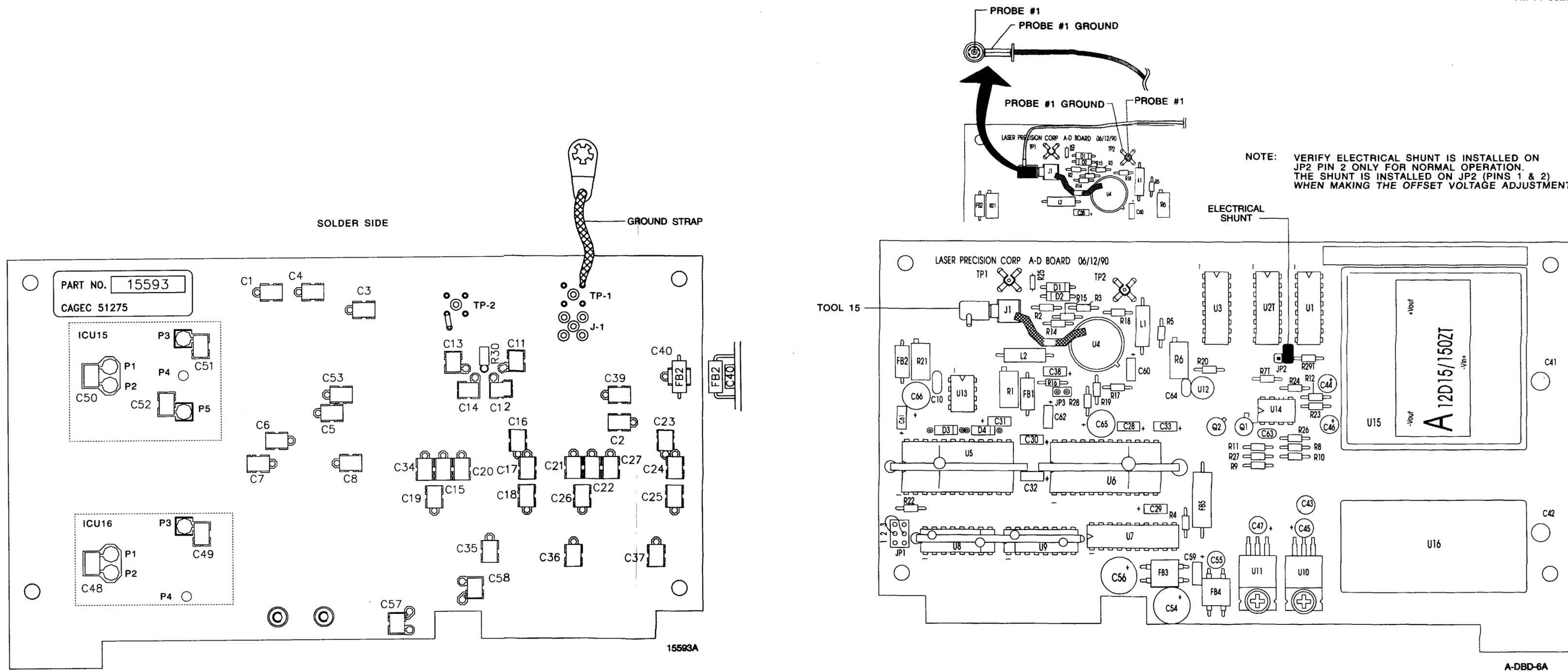
Figure FO-10. 1A2A8 A to D Converter CCA Component Locator Diagram.
