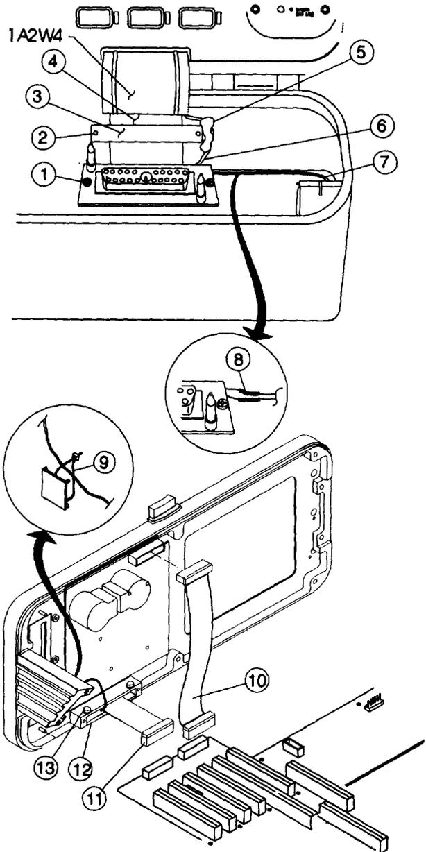
7. Form coax cable (6) to prevent damage to cable and install mounting screws (1). Connector should be able to float.
