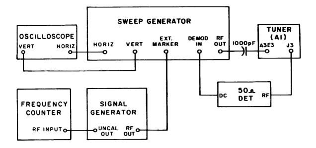
Figure 4-7. Test Setup, Tuner IF Output Amplifier Alignment
