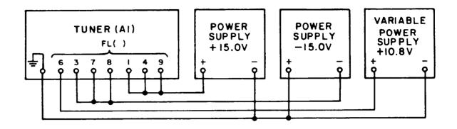
Figure 4-6. Test Setup, Tuner Power Connections
