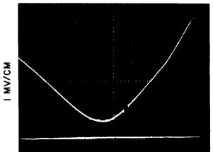
Figure 4-12. Typical Response, 500 MHz VSWR Alignment
