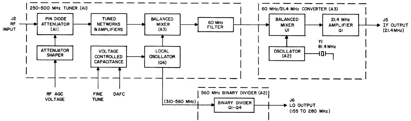
Figure 3-1. Type WJ-9124 Tuner Assembly Functional Block Diagram
