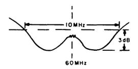
Figure 4-5. Typical Response, 60 MHz to 21.4 MHz Converter
