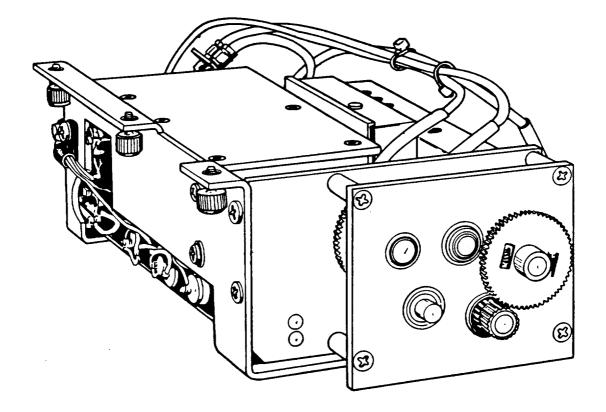
Figure 1-1. WJ-9124 250-500 MHz Tuner Assembly
