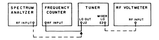
Figure 4-9. Test Setup, Oscillator Stage Alignment
