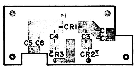
Figure 5-7. Part 17083 Pin Diode Attenuator (A1A1), Location of Components
