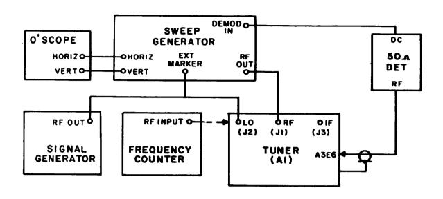
(6) Set the signal generator to 60 MHz at a level sufficient to produce a marker.
