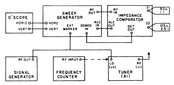
Figure 4-10. Test Setup, Tuner VSWR Alignment Circuit
