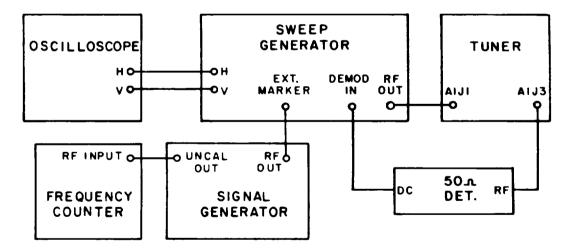
Figure 4-2. Test Setup, Overall Tuner Gain
