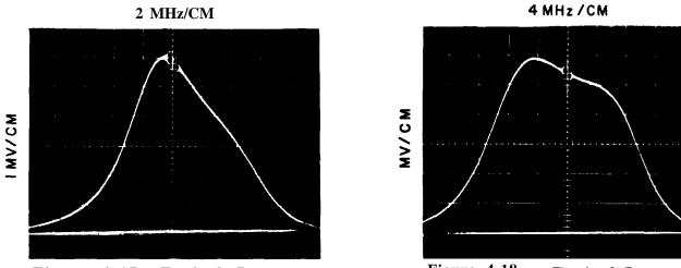
Figure 4-17. Typical Response, 250 MHz Interstage Response
