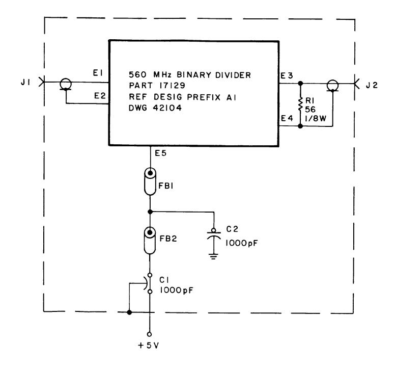
Figure 6-3. Type 791834 560 MHz Binary Divider (A2), Schematic Diagram 34957
