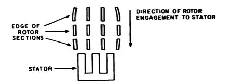
Figure 4-14. Rotor Plate Adjustment
