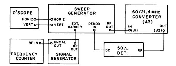
Figure 4-20. Test Setup, 60 MHz/ 21.4 MHz Converter Assembly Alignment
