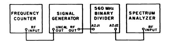
Figure 4-3. Test Setup, 560 MHz Binary Divider Performance Test
