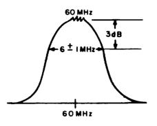
Figure 4-8. Typical Response, IF Output Amplifier Alignment
