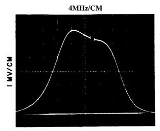
Figure 4-19. Typical Response, 500-475 MHz Interstage Response
