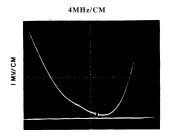
Figure 4-15. Typical Response, 475-425 MHz VSWR Alignment
