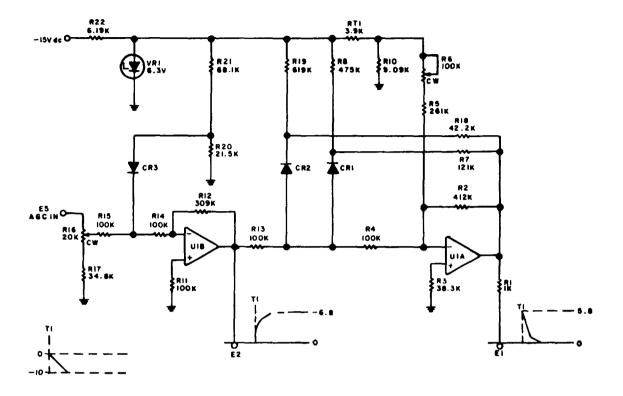
Figure 3-2. Simplified Schematic Diagram, Attenuator Shaper
