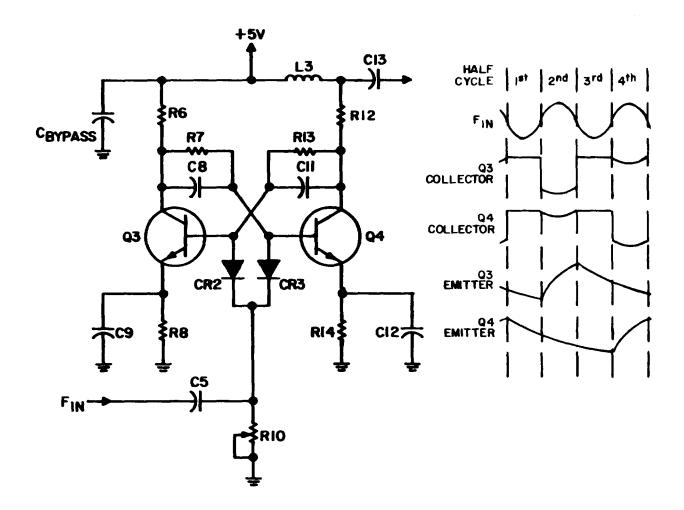
Figure 3-3. Simplified Schematic Diagram, Dynamic Frequency Divider
