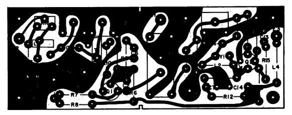
Figure 5-13. Part 16697-2 60/21. 4 MHz Converter (A3A1), Location of Components
