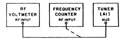
Figure 4-1. Test Setup, LO Performance Test
