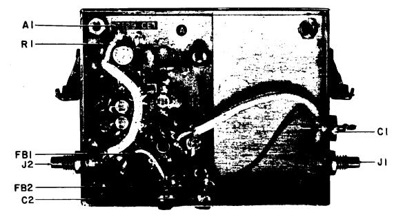
Figure 5-10. Type 791834 560 MHz Binary Divider Assembly (A2), Location of Components
