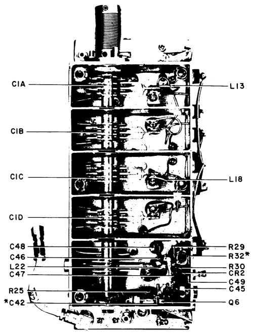
Figure 5-6. Type 71376-6 250-500 MHz Tuner, (A1), Location of Components
