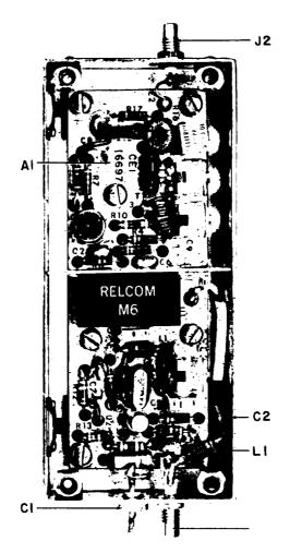
Figure 5-12. Type 71347-4 60/21. 4 Converter Assembly (A3), Location of Components
