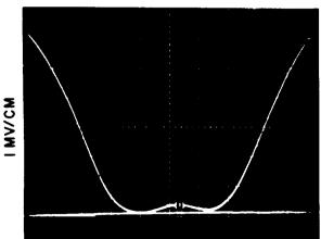
Figure 4-11. Typical Response, 250 MHz VSWR Alignment
