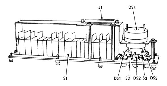
• Remove component: connector J1 is mounted to the bracket with two standoff screws, washers, and nuts; Rate/Mode assembly S1 is mounted to the front panel with four screws, nuts and washers (two have already been removed); switches S2 and S3 are mounted to the front panel with nuts and washers on the outside of the panel; and lamps DS1, DS2, and DS3 are mounted to the front panel with nuts and washers on the inside of the panel.
