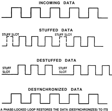
ORIGINAL STATE AFTER STUFFED SLOTS HAVE BEEN REMOVED.
