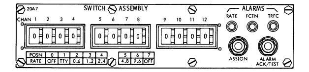
a. <u>Thumbwheel Switches</u>. The Switch Assembly thumbwheel switch is a printed circuit rotary type switch. Each switch uses three isolation diodes to prevent coding interference from the other unselected thumbwheels. The positions dialed on the 12 thumbwheel switches are encoded onto a 3-bit bus and buffered by the DCPG card. This allows the Common Control to read the selected data rates. Buffered output codes are defined as follows:
