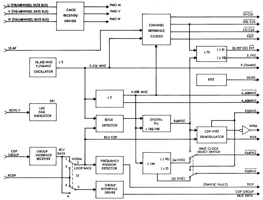
d. <u>CDP Demodulator</u>. The conditioned diphase demodulator processes RCDP into NRZ format using the regenerated R64 kHz for timing. The demodulated data is designated WDR and is output from the board.
