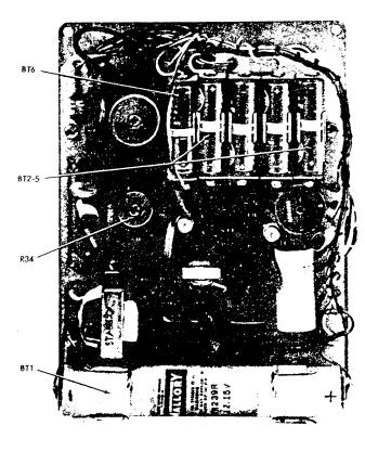
Figure 4–1. Rear of Front Panel Components
