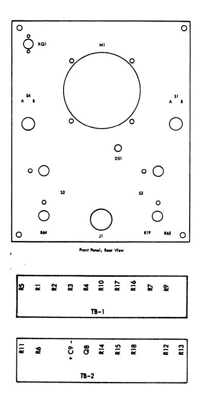
Flgure 4-3. Component Location, Terminal Boards and Rear of Front Panel 4-3
