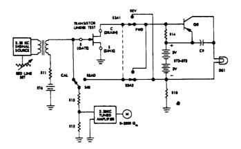
Ffgure 3-6. Field Effect Transistor Test
