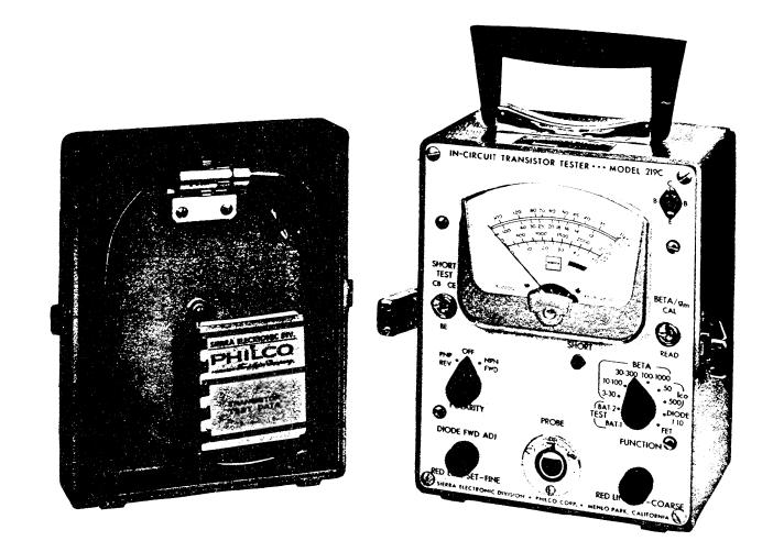
Figure 1-1. Model 219C In-Circuit Transistor Tester
