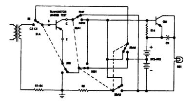
Figure 3-3. BE Short Test, PNP Transistor
