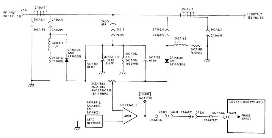
Figure 2-6. Simplified Phasing Discriminator Circuit Diagram
