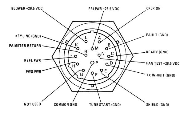
Figure 1-9. Connector 2A1J2 Pin/Functional Identification
