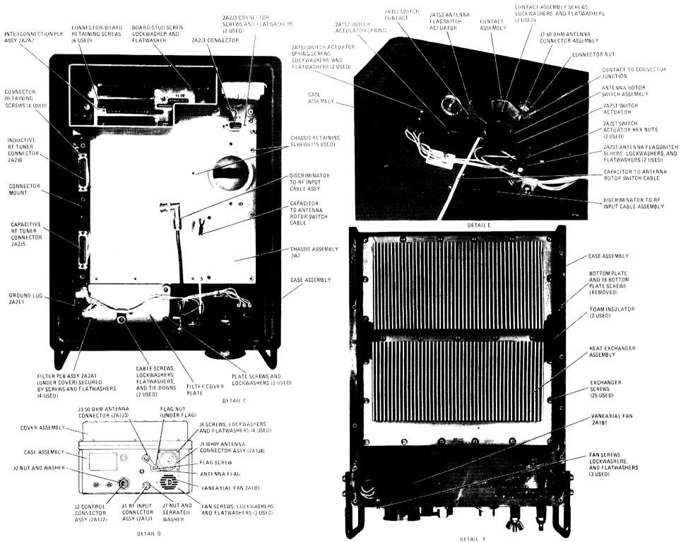
Figure 3-2. Antenna Coupler CU-2064/GRC-193 Disassenlbly/Reassembly Details (Sheet 2 of 2)
