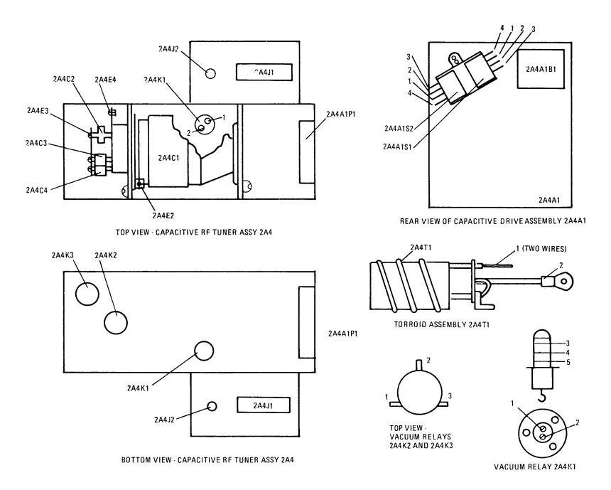
Figure 3-30. Capacitive RF Tuner Assembly 2A4 Component Lead Identification Details
