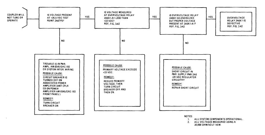
Figure 3-5. Dc Power Fault Logic Diagram
