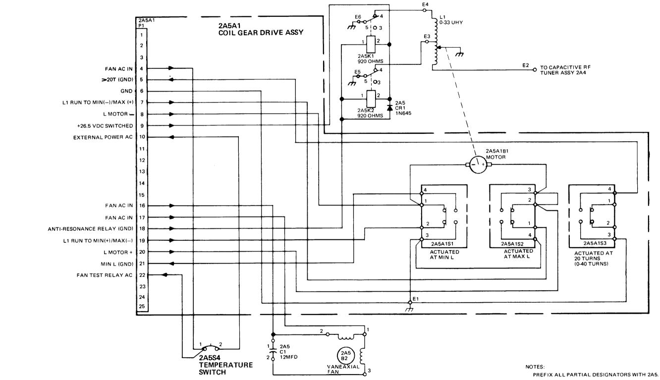
Figure 3-41. Inductive RF Tuner Assembly 2A5 Schematic Diagram
