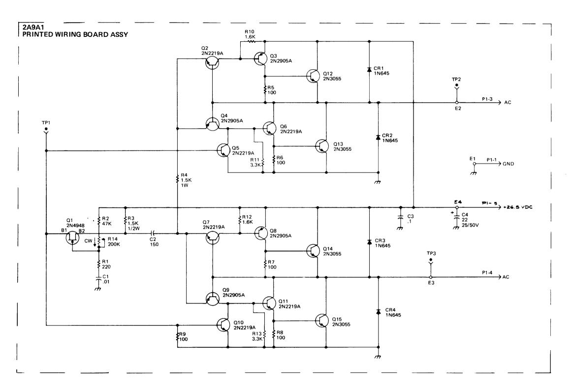
Figure 3-45. Static Inverter Power Assembly 2A9 Schematic Diagram
