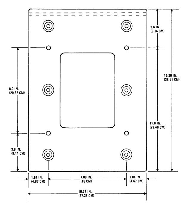
Figure 1-7, Antenna Coupler Mount MT-4495/GRC-193 Lower Tray Assembly Dimensional Data
