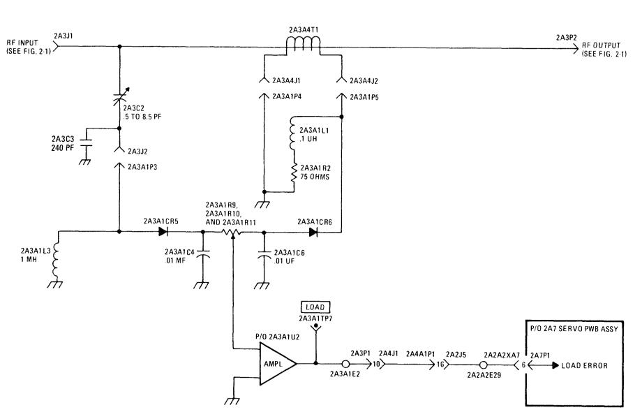
Figure 2-7. Simplified Loading Discriminator Circuit Diagram
