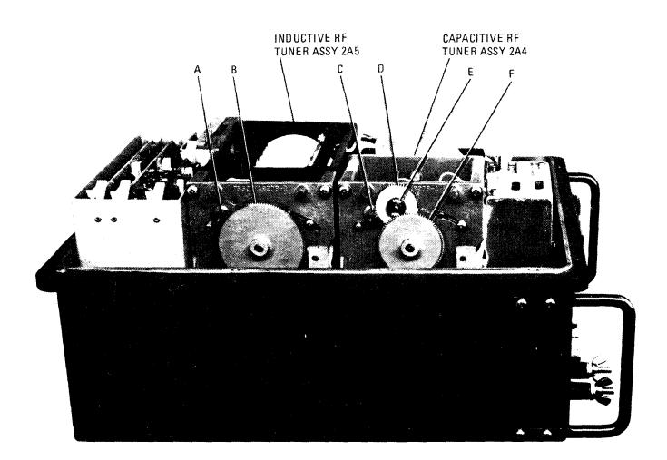
Figure 3-3. RF Tuner Assemblies Lubrication Points
