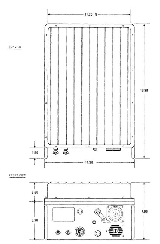
Figure 1-8. Antenna Coupler CU-2064/GRC-193 Dimensioned Views
