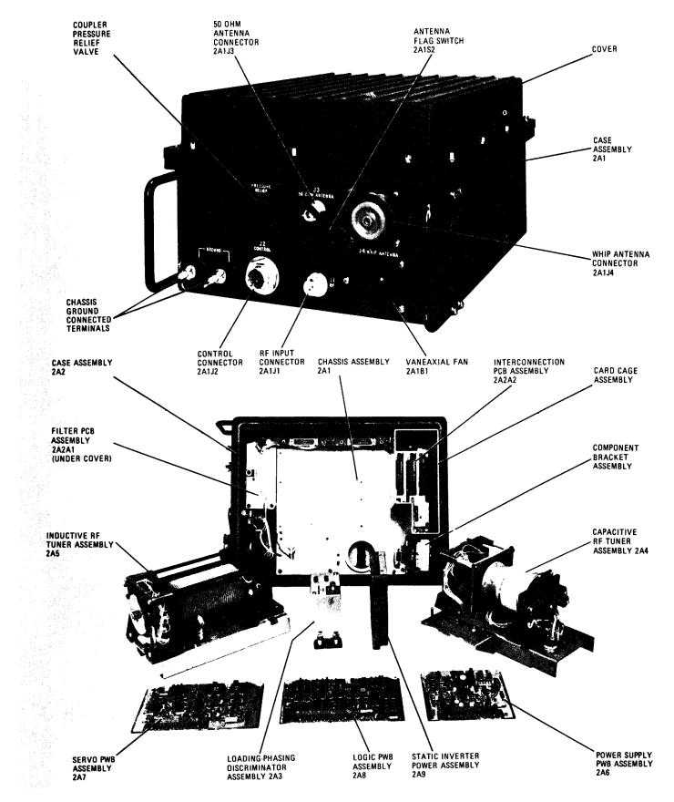
Figure 14. Antenna Coupler CU-2064/GRC-193, Major Assembly and Component Identification
