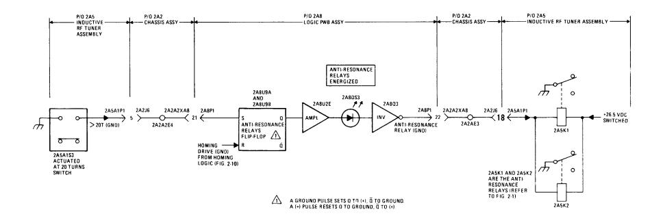
Figure 2-17. Simplified Anti-Resonance Relay Logic Diagram
