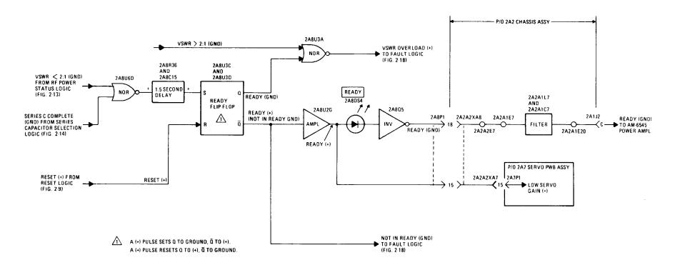
2-88. When the coupler is tuned and the VSWR is <2:1, both inputs of U6D are low, sending its output high. This level, applied to U3D-13, sets ready flip-flop U3C/U3D. With the flip-flop set, a low signal is placed on U3A, placing a low on the VSWR overload line. A high is applied to U2G13, causing the low servo gain line to be high, READY LED DS4 to go on, and Q5 to be biased on. With Q5 on, the ready (GND) line is low.
