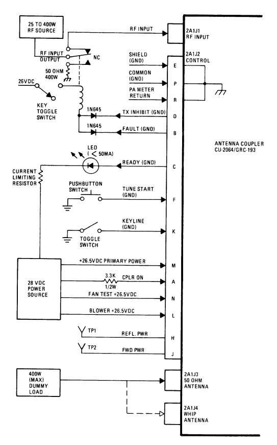
Figure 3-1. Special Test Setup for Testing Coupler
