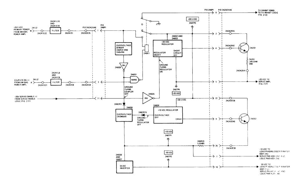
Figure 2-20. Simplified Power Supply PWB 2A6 Circuit Diagram
