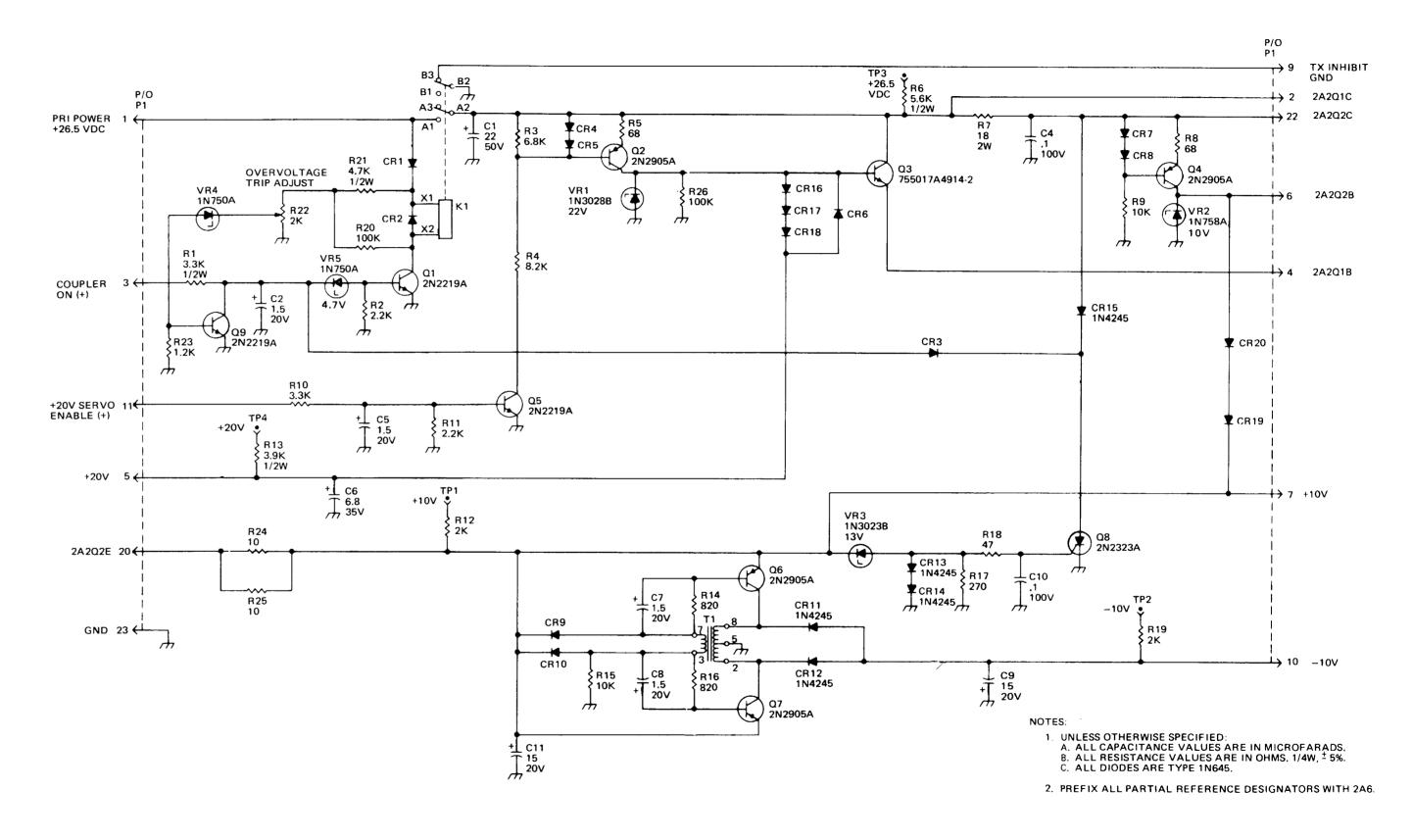
Figure 3-42. Power Supply Pwb Assembly 2A6 Schematic Diagram
