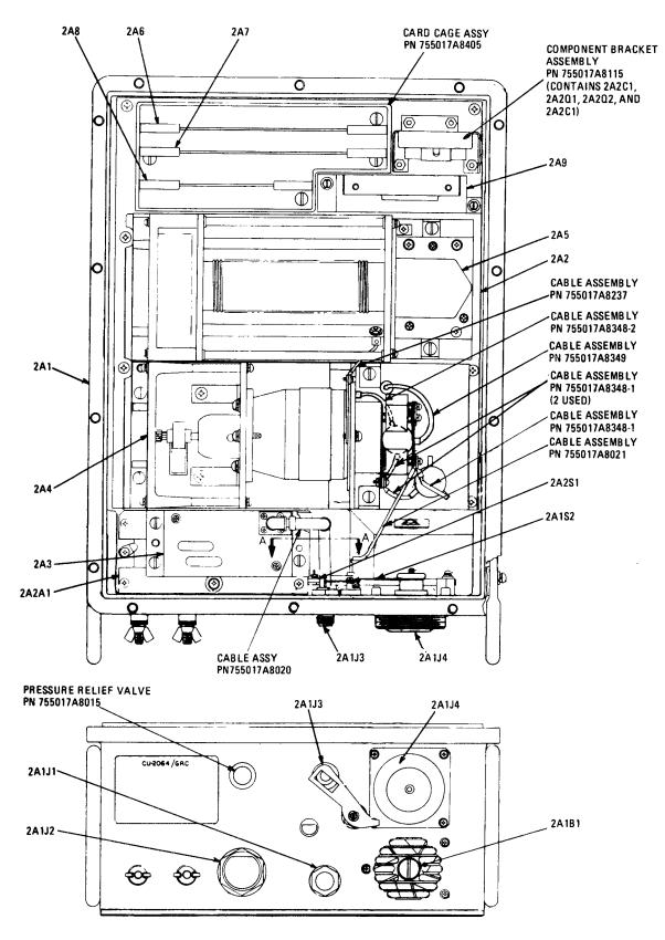
Figure 3-21. Antenna Coupler CU-2064/GRC-193 Component Locations
