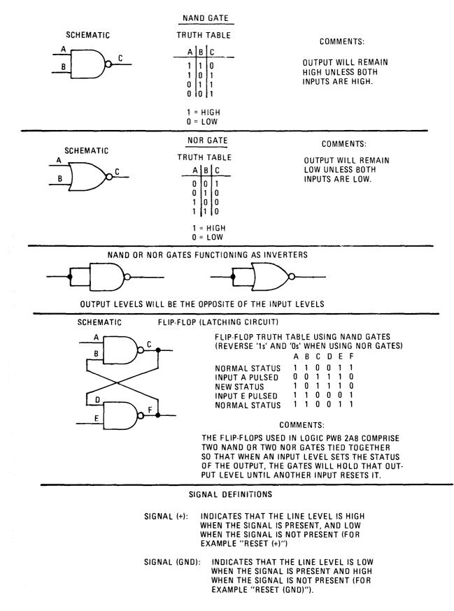
Figure 2-8. Logic Representations and Definitions - Logic PWB Assembly 2A8
