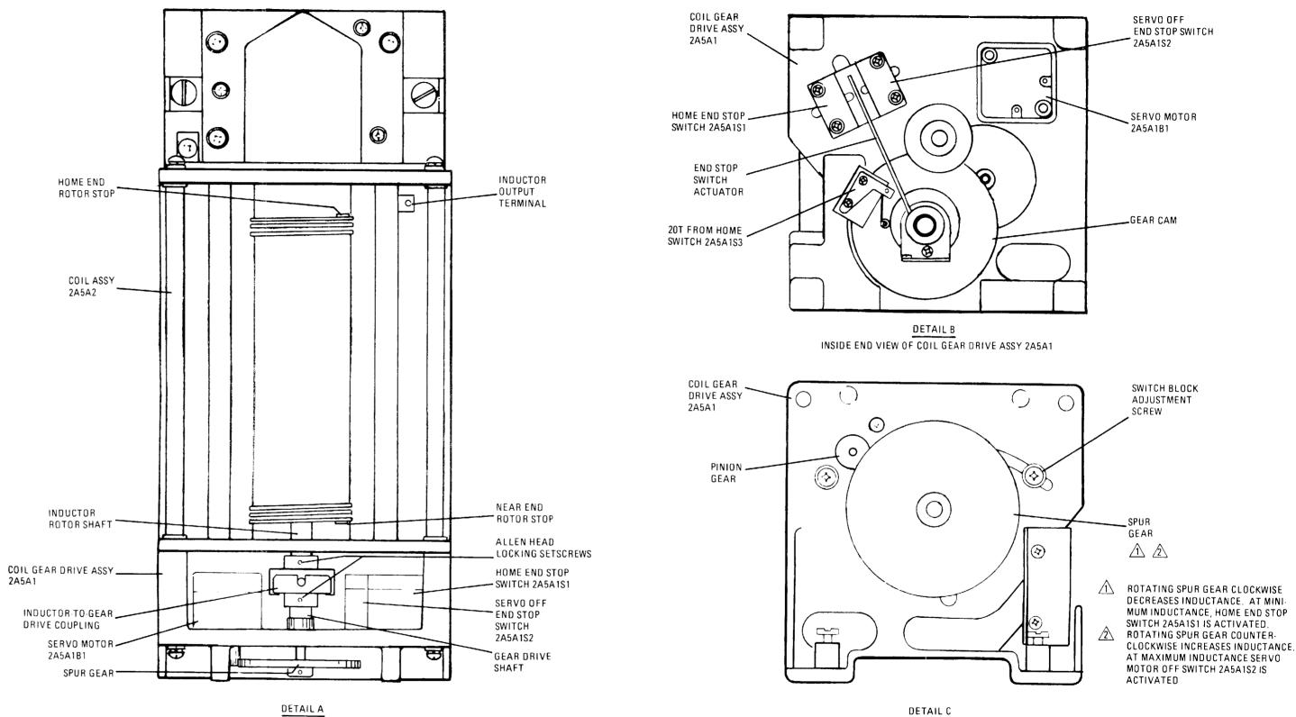
TOP VIEW OF COIL GEAR DRIVE ASSY 2A5A1
