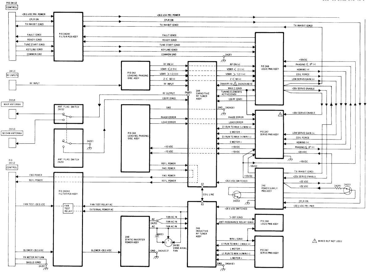
Figure 2-2. Overall Functional Interconnection Diagram
