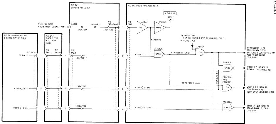
Figure 2-13. Simplified RF Power Status Logic Diagram
