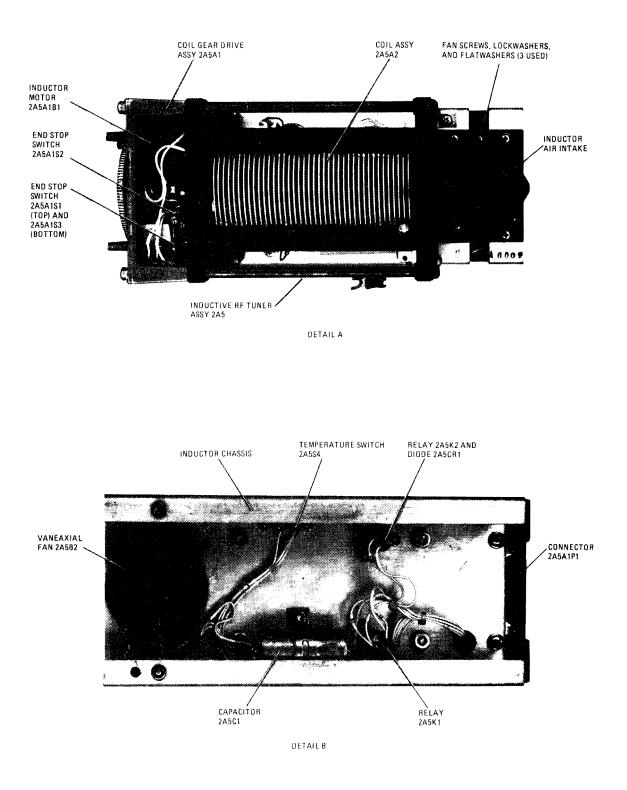
Figure 3-20. Inductive RF Tuner Assembly 2A5 - Component Details
