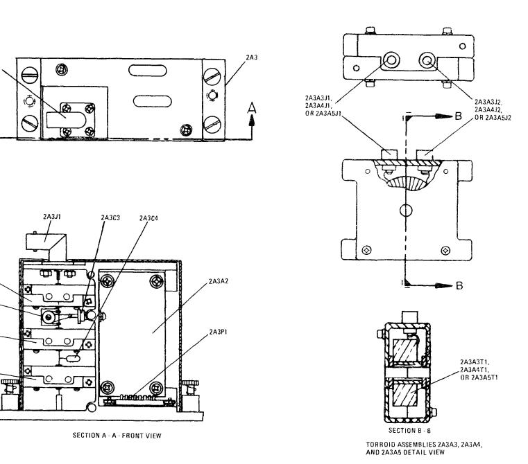
Figure 3-26. Loading-Phasing Discriminator Assembly 2A3 Component Locations
