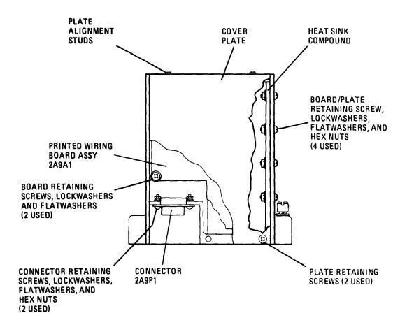
Figure 3-18. Static Inverter Power Assembly 2A9 - Disassembly Details
