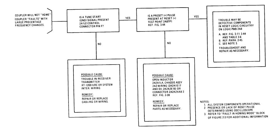
Figure 3-8. Coupler Tune Start/Reset Logic Fault Logic Diagram
