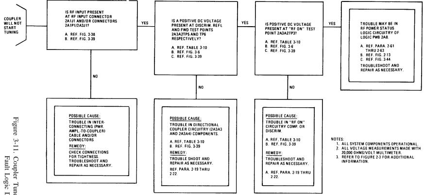
Figure 3-11. Coupler Tune Start Fault-Fault Logic Diagram
