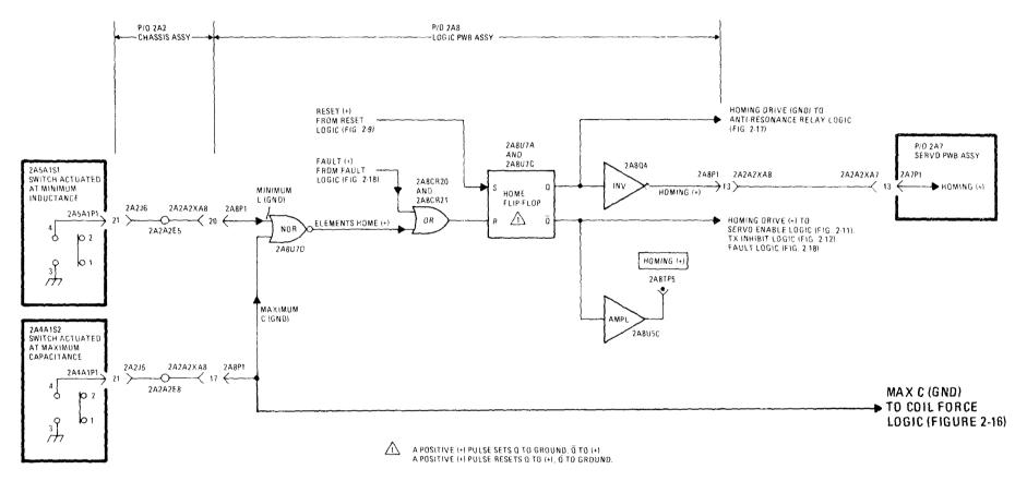
Figure 2-10. Simplified Homing Logic Diagram
