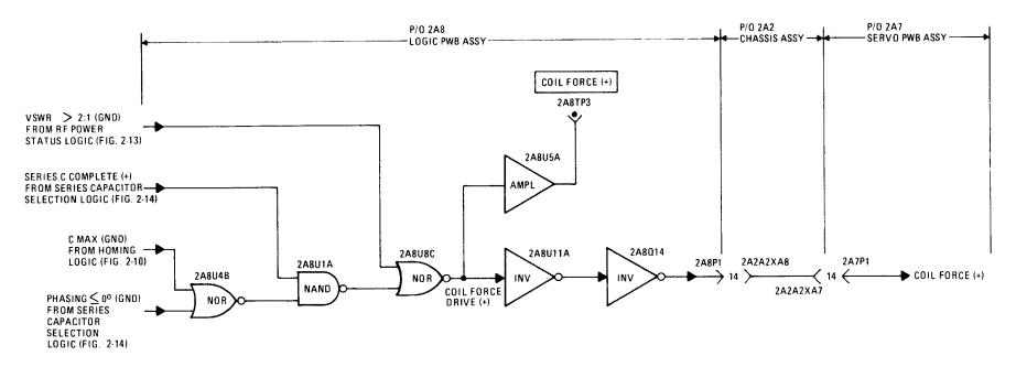
Figure 2-16. Simplified Coil Force Logic Diagram
