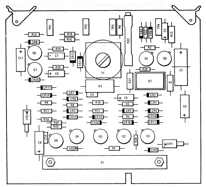
Figure 3-33. Power Supply Pwb Assembly 2A6 Component Locations
