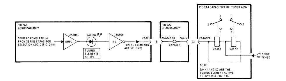
Figure 2-15. Simplified Tuning Elements Active Logic Diagram
