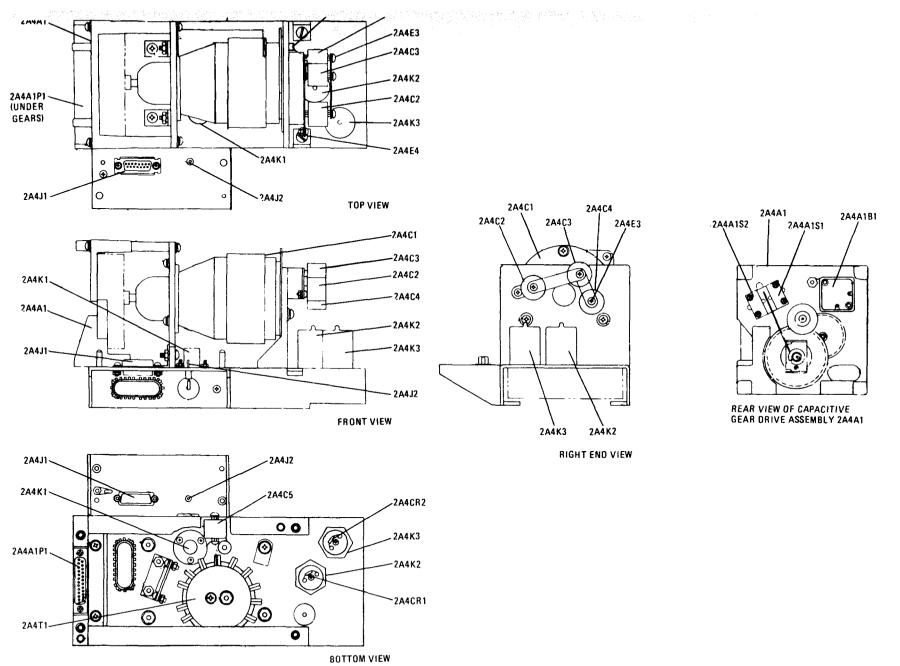
Figure 3-29. Capacitive RF Tuner Assembly 2A4 Component Locations
