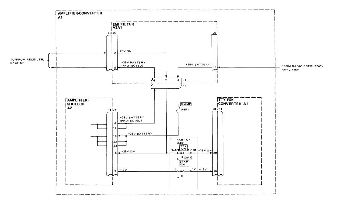
Figure 4-3. Amplifier-Converter A1 Power Distribution
