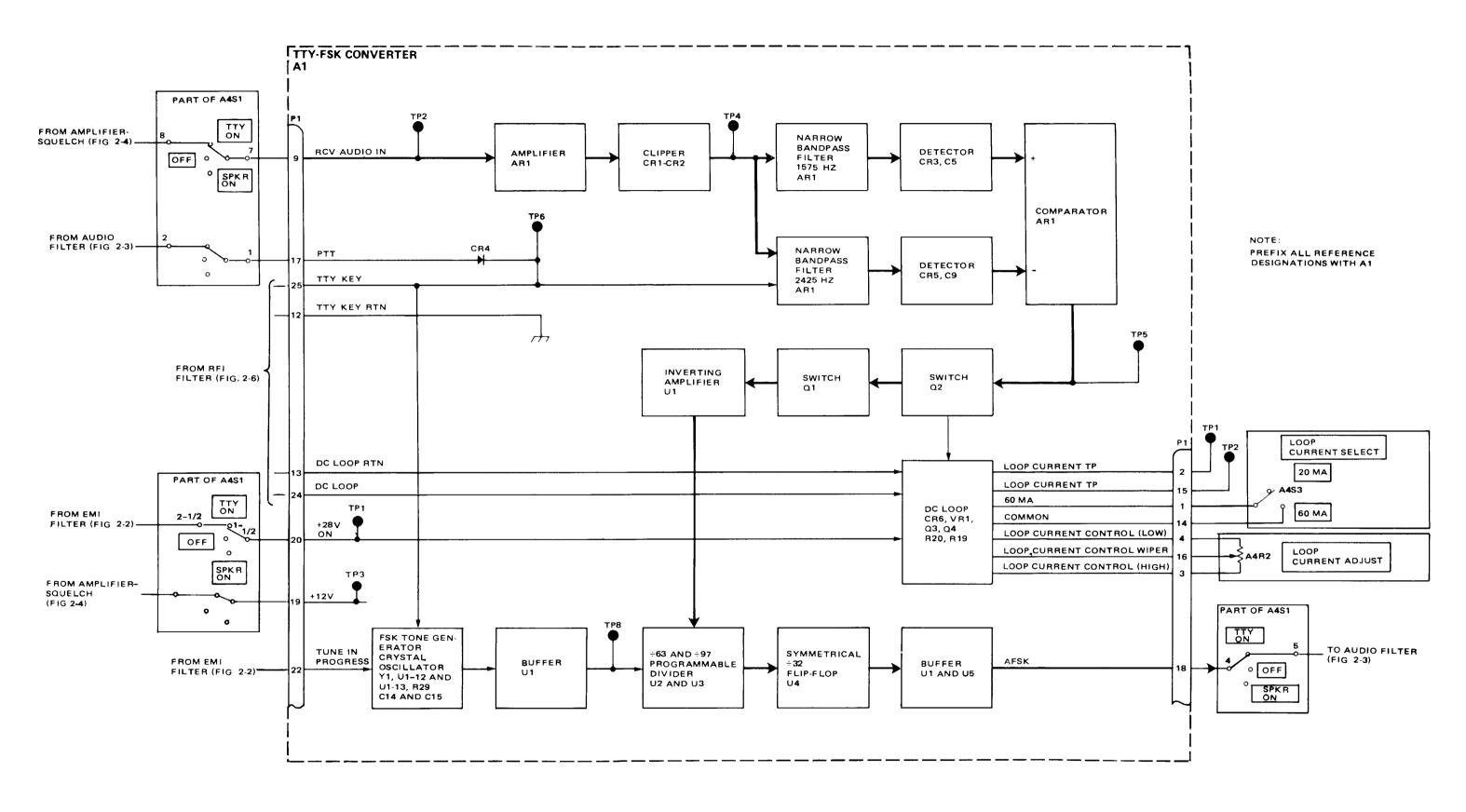
Figure 2-5. TTY-FSK Converter A1A1 Detailed Block Diagram.
