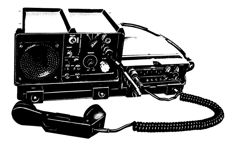
Figure 1-0. Amplifier-Converter AM-6879/URC, Receiver/Exciter RT-1209/URC, and Electrical Equipment Mounting Tray MT-4874/URC
