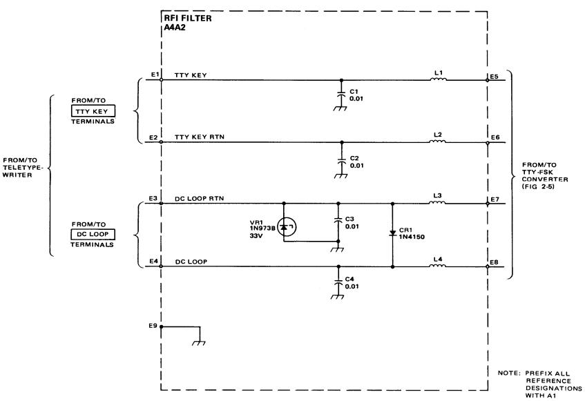
Figure 2-6. RFI Filter AlA4A2 Detailed Block Diagram
