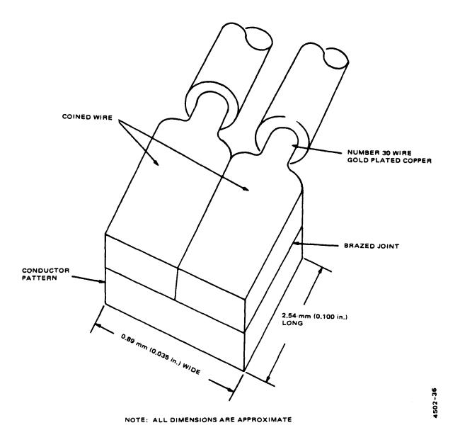
Figure 3-8. Double-Wire Attachment to Printed Circuit Pad
