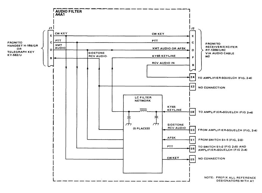
Figure 2-3. Audio Filter AlA4Al Detailed Block Diagram
