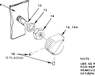
USE AS REFERENCE FOR REPLACING AND REMOVING BOTH TTY ON/ OFF/SPKR ON SWITCH (S1) AND SQUELCH SWITCH (R1/S2)
