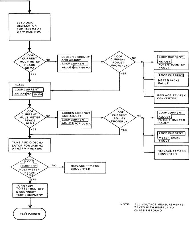
Figure 4-7. Amplifier-Converter A1 Performance Test
