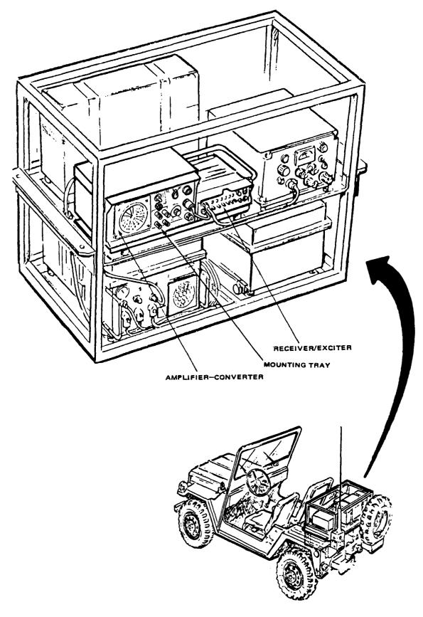
Figure 1-1. Typical Amplifier-Converter and Receiver/Exciter Vehicle-Mounted Configuration
