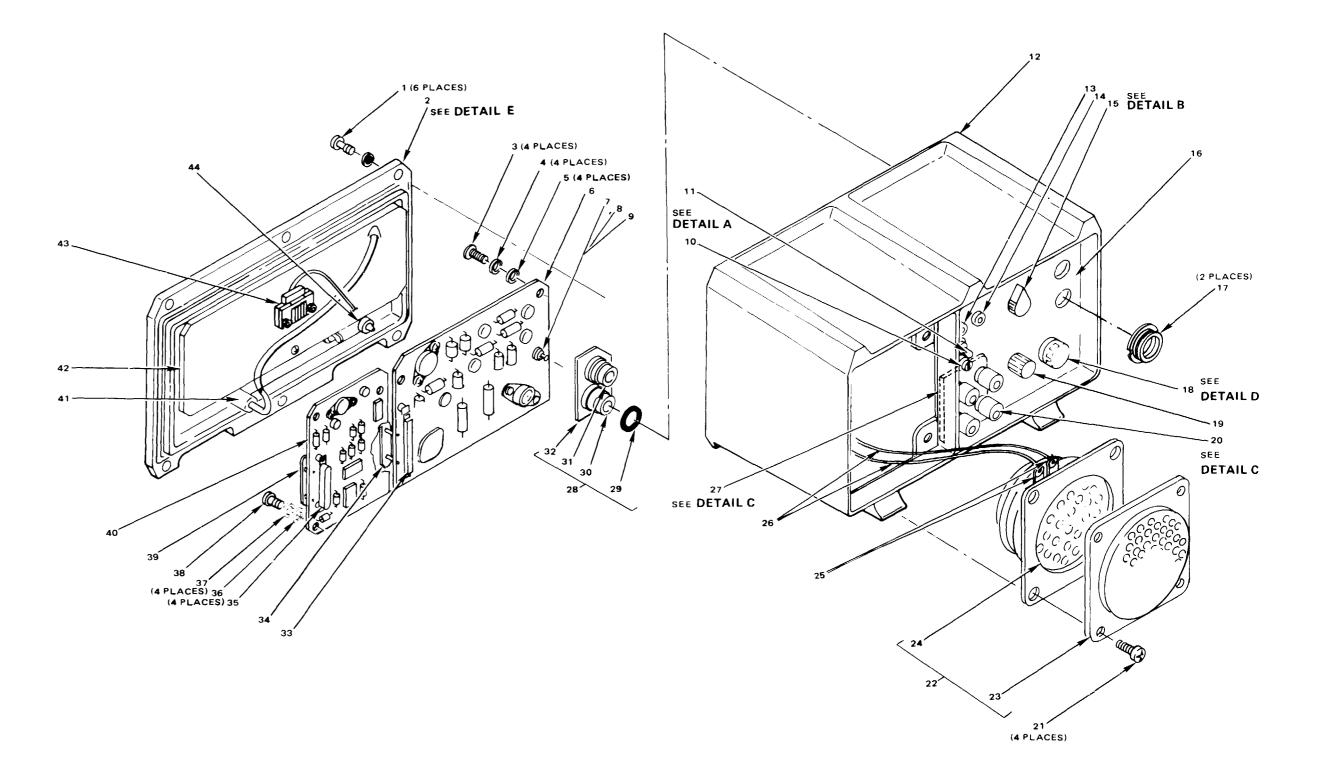
Figure 4-4. Amplifier-Converter Component Location (Rear Cover Assembly A1A3, Circuit Cards, Switches and Fuse) (Sheet 1 of 3)
