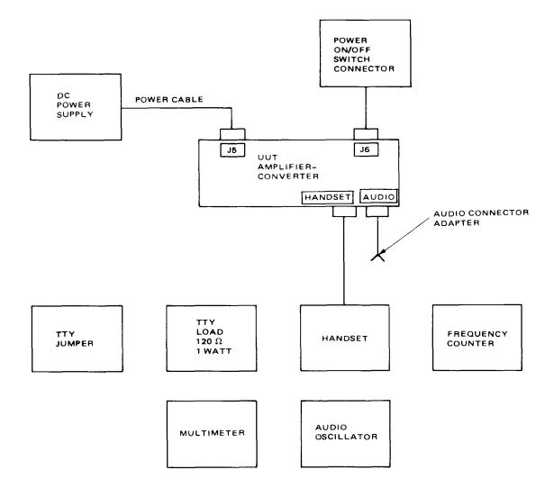
Figure 4-6. Amplifier-Converter A1 Test Setup
