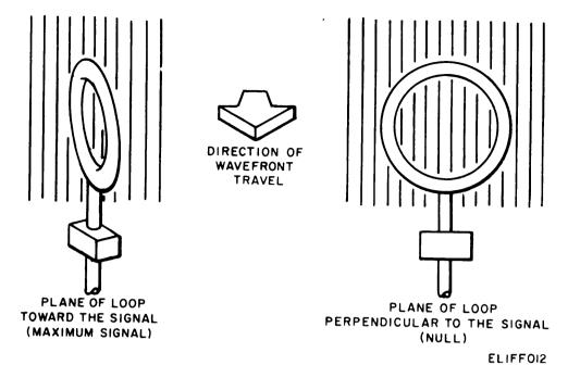
Figure 5-3. Loop antenna planes.
