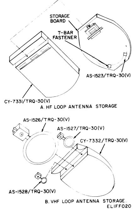
Figure 3-3. Storage of loop antennas.
