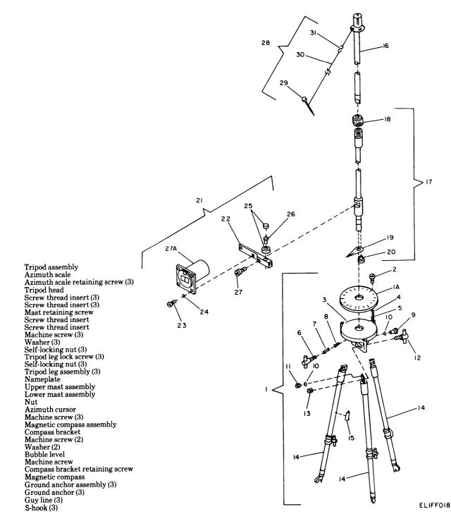
Figure 6-4. Antenna pedestal assembly, exploded view.
