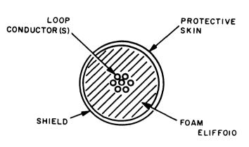
Figure 5-1. Cross-section of typical loop antenna.
