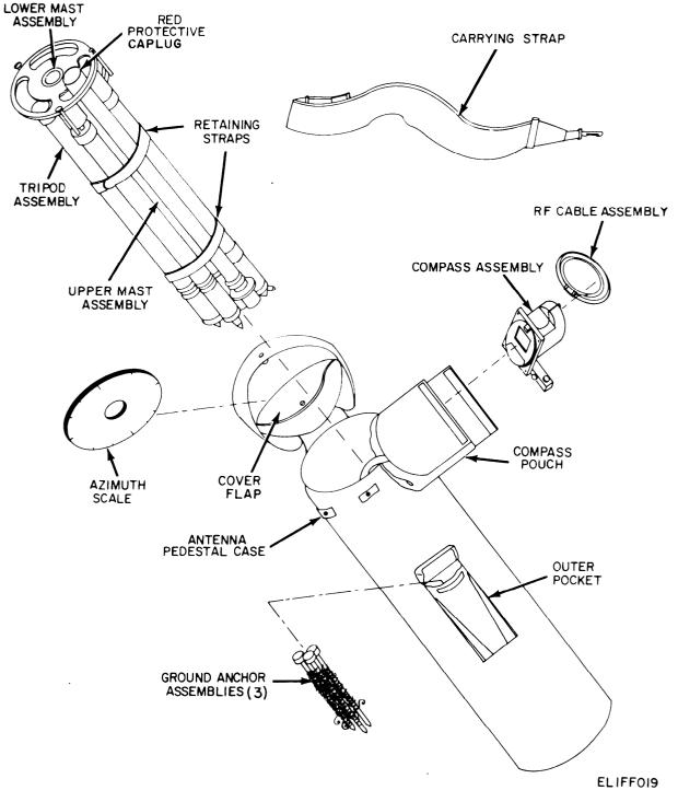
Figure 3-4. Storage of AB-1110/TRQ-30(V) components.
