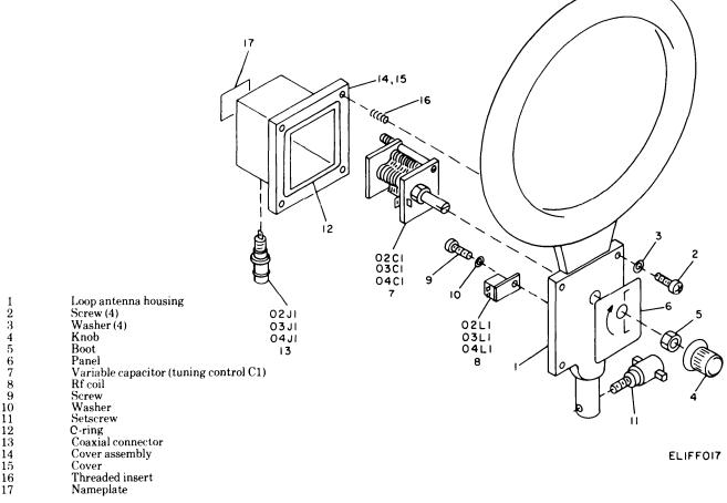
Figure 6-3. Typical vhf loop antenna, exploded view.
