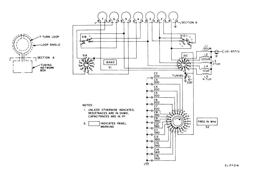
Figure 5-5. Hf loop antenna, schematic diagram.
