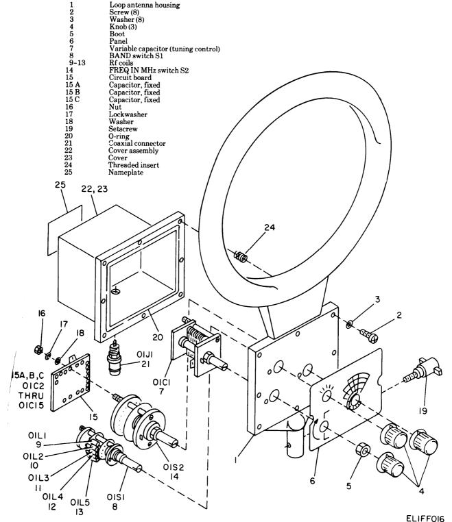
Figure 6-2. Hf loop antenna, exploded view.
