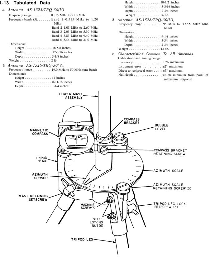
Figure 1-6. Tripod assembly, upper section.
