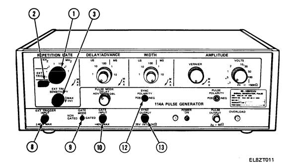
*c.* Sync Output. A sync output pulse is provided to synchronize another piece of equipment with the signal generator.
