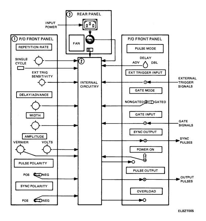
Figure 1-2. Pulse Signal Generator SG-1205(V)1/U Block Diagram
