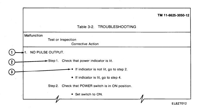
${f D}$  Malfunctions are those that cause symptoms seen or heard at the equipment without using test equipment.
