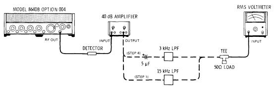
Figure 4-8. Residual AM Test Setup
