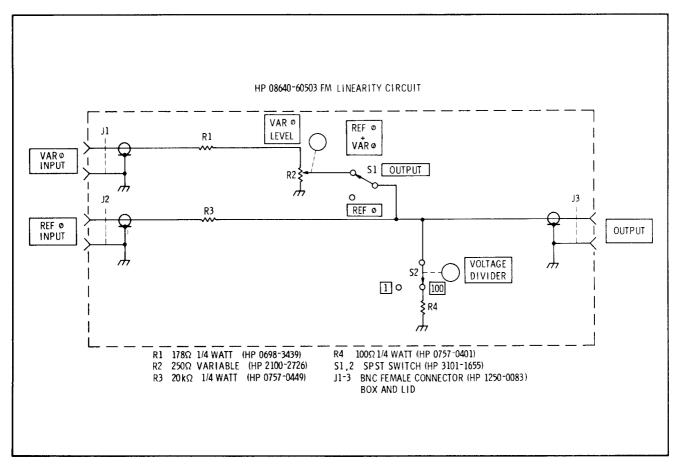
Figure 1-8. FM Linearity Circuit
