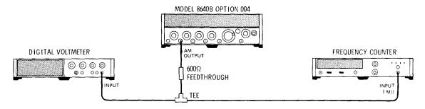
Figure 4-16. Internal Modulation Oscillator Test Setup
