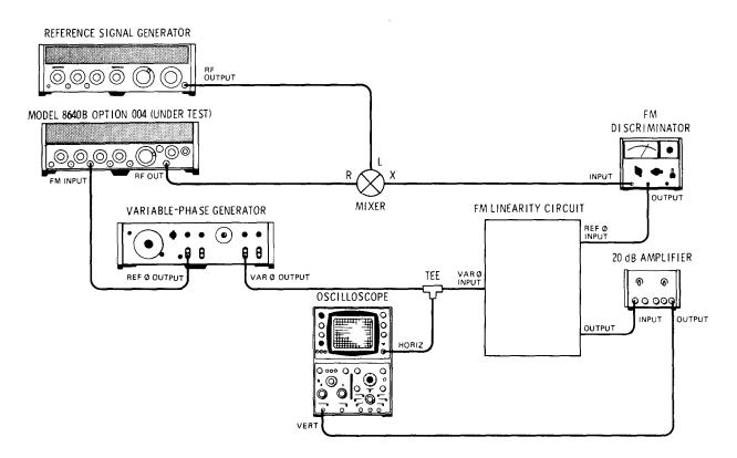
Figure 5-11. FM Linearity Adjustment Test Setup
