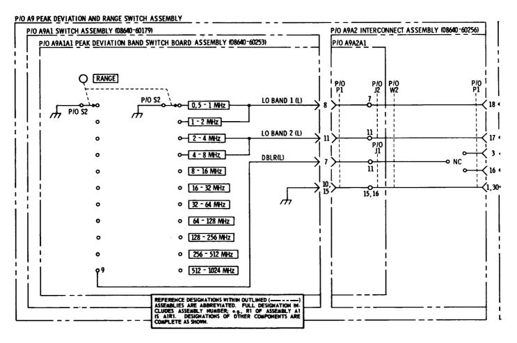
P/O Figure 8-53. AM Interconnections and RF ON/OFF Switch Schematic Diagram (P/O Change 7)
