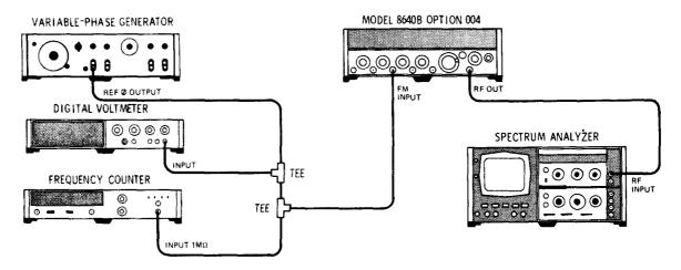
Figure 5-14. FM Sensitivity Adjustment Test Setup
