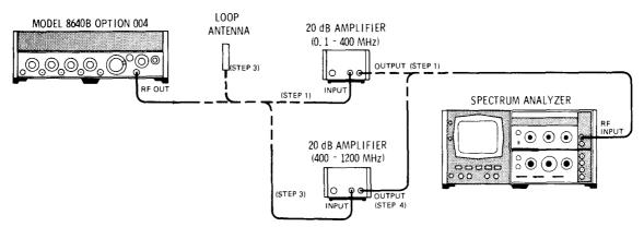
Figure 4-15. Output Leakage Test Setup
