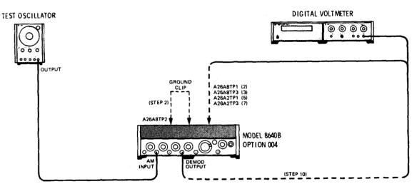
Figure 5-3. Preliminary AM Adjustments
