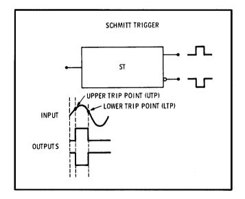
Figure 8-7. Schmitt Trigger
