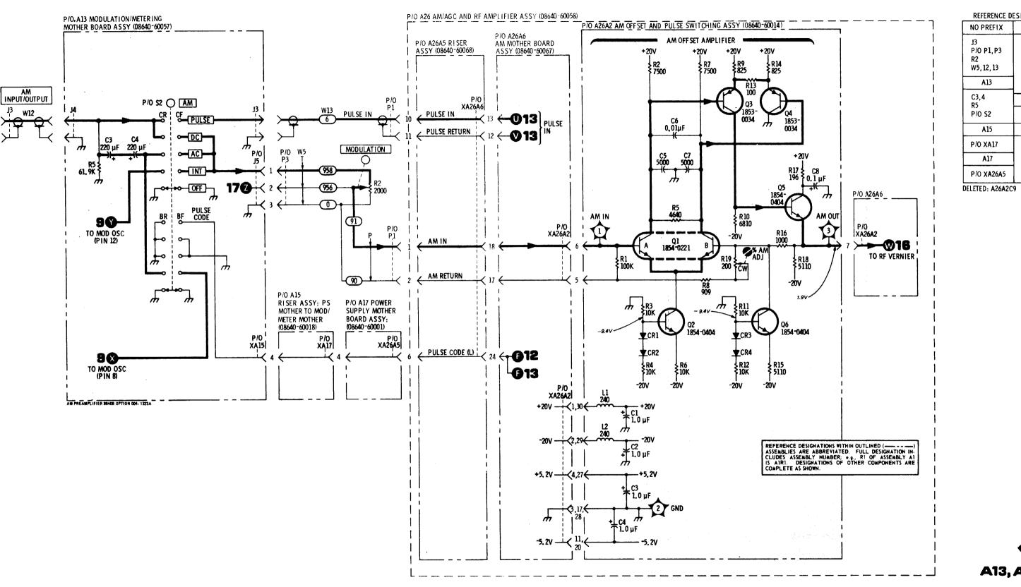
Figure 8-51. AM Preamplifier Schematic Diagram
