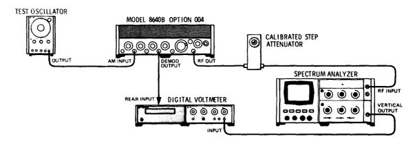
Figure 5-4. AM Accuracy Adjustment Test Setup
