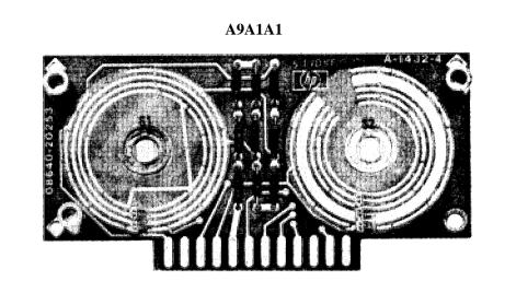
Figure 8-31A. A9A1A1 Peak Deviation Band Switch Board Assembly Component Locations (P/O Change 7)
