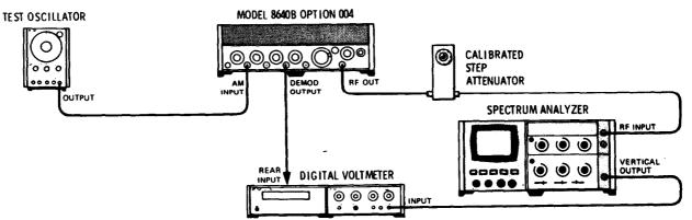
Figure 4-22. Demodulated Output Accuracy Test Setup
