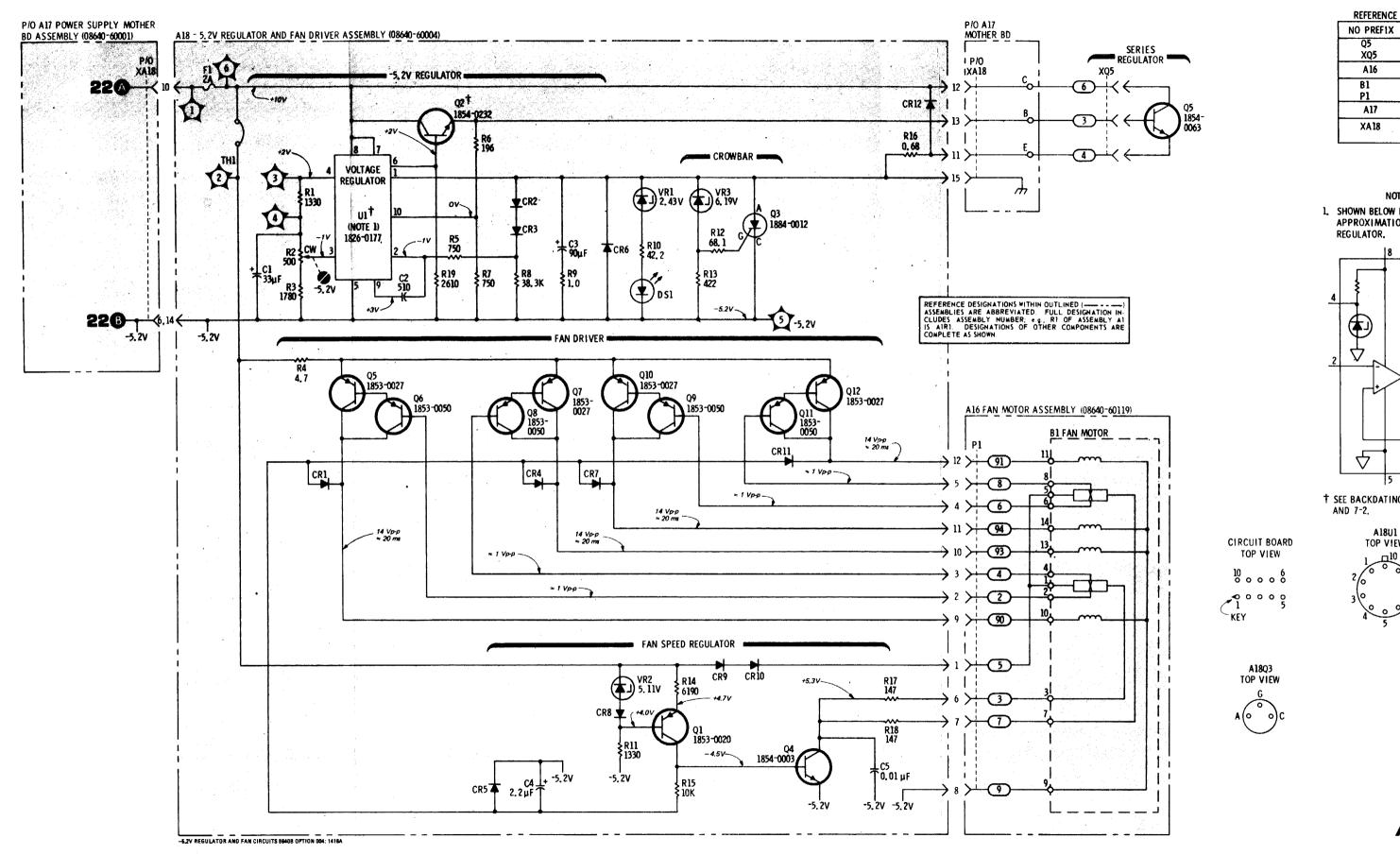
Figure 8-75. A18-5.2V Regulator and Fan Driver Assembly Component Locations
