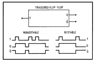
Figure 8-5. Triggered Flip-Flop
