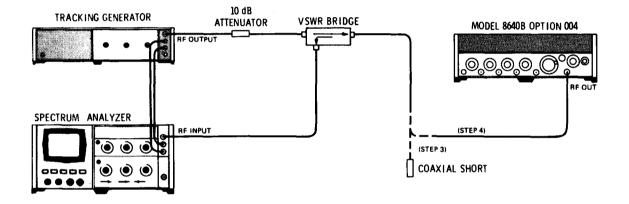
Figure 4-14. Output Impedance Test (Broadband)
