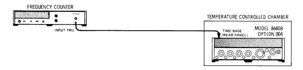
Figure 4-33. Internal Reference Accuracy Test Setup
