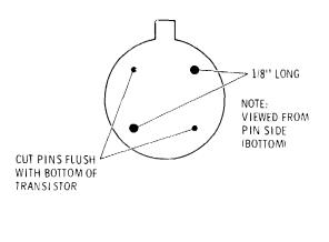
Figure 8-82. RF Oscillator Transistor Preparation
