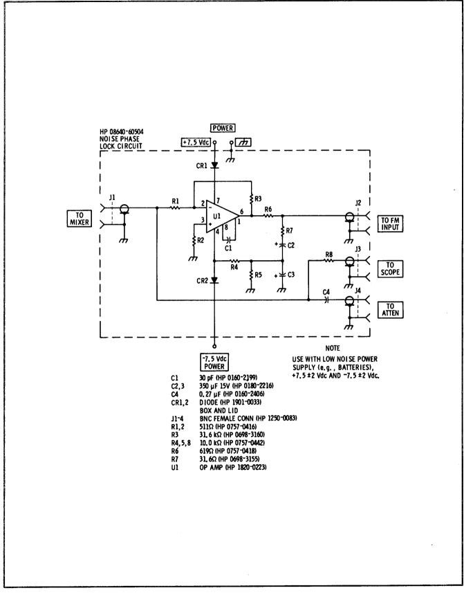
Figure 1-9. Noise Phase Lock Circuit
