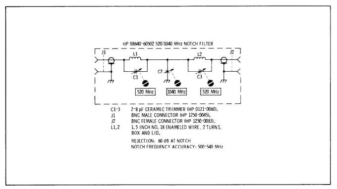
Figure 1-7. 520/1040 MHz Notch Filter
