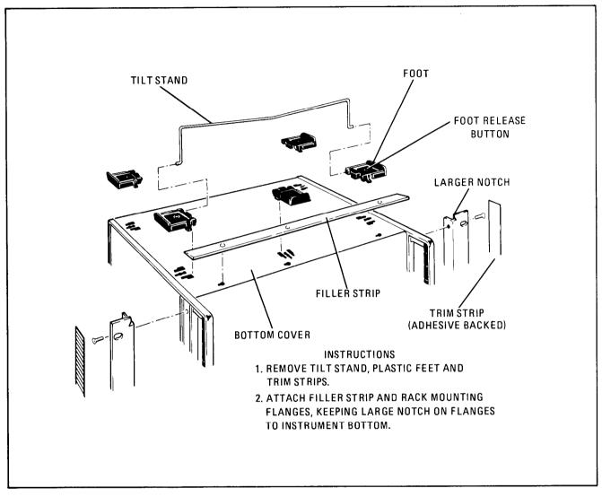
Figure 2-3. Preparation for Rack Mounting
