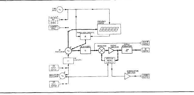
Figure 8-17. Simplified Block Diagram
