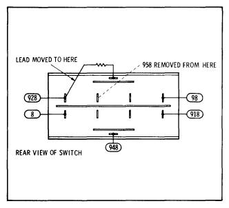
Figure 7-9. Modified Line Switch Wiring
