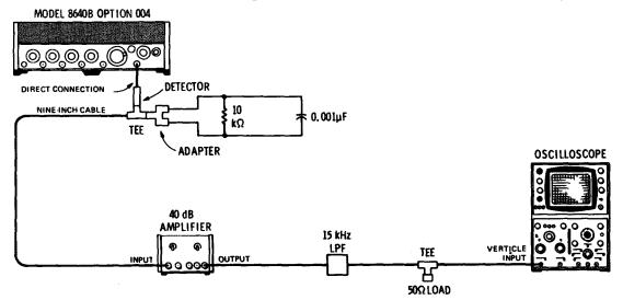
Figure 4-31. Incidental AM Test Setup
