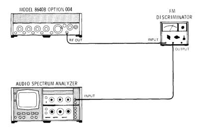
Figure 4-29. FM Distortion Test Setup
