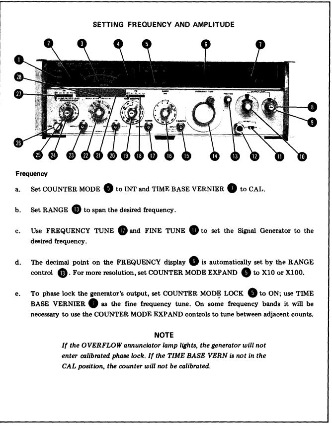
Figure 3-6. Setting the Frequency and Amplitude Controls (1 of 3)
