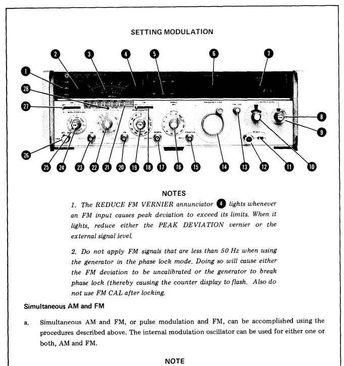
On Signal Generators with the Option 001 Variable Modulation Oscillator, don't load both AM OUTPUT (2) and FM OUTPUT (2) when the oscillator is providing both modulating signals. The outputs are in parallel and the parallel load should be greater than 600 ohms.
