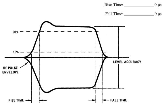
Figure 4-27. Pulse Measurements
