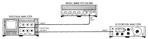
Figure 4-19. AM Distortion Test Setup
