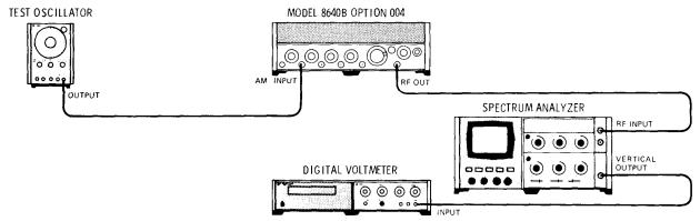
Figure 4-25. AM Flatness Test Setup
