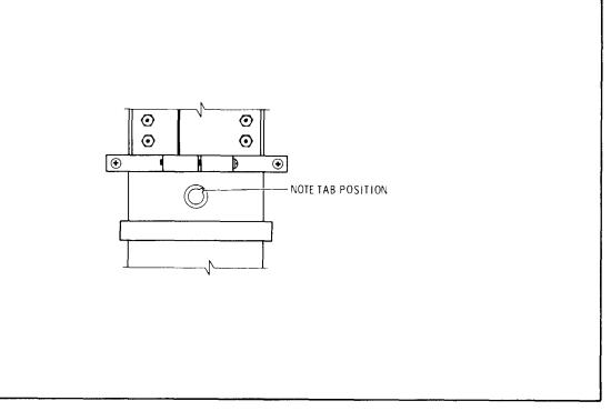
Figure 8-83. RF Oscillator Transistor Orientation
