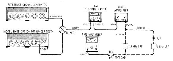
Figure 4-9. Residual FM Test Setup
