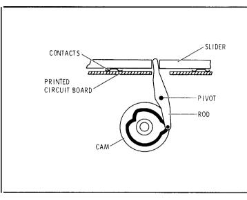
Figure 8-38. Action of RANGE Switch
