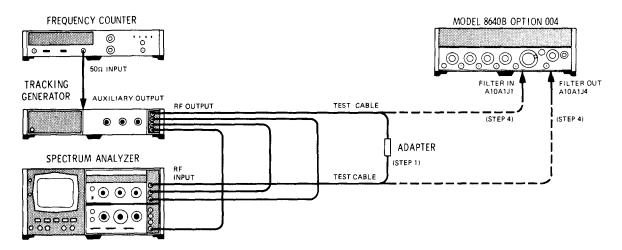
Figure 5-9. RF Filter Adjustment Test Setup
