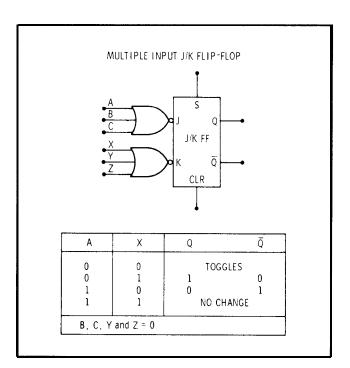
Figure 8-9. Multiple Input J/K Flip-Flop
