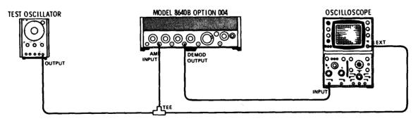
Figure 4-23. AM Phase Shift Test Setup
