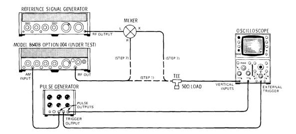
Figure 4-26, Pulse Modulation Test Setup
