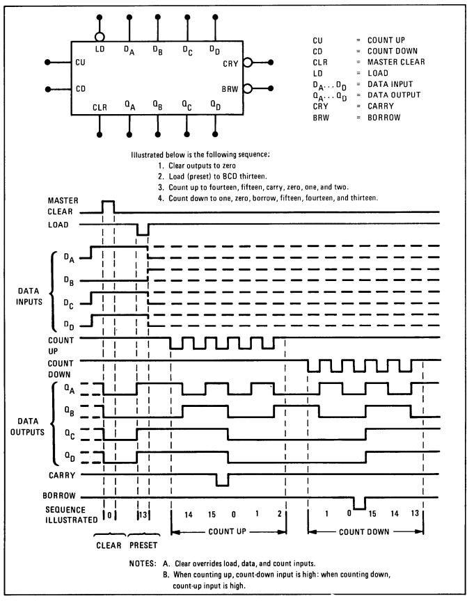
Figure 8-14. Programmable Up/Down Counter
